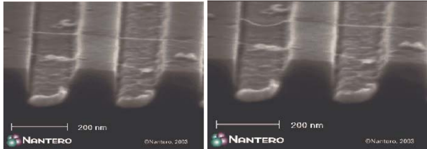
Electro-mechanical random access memory (memory) device in the off (left) and on (right) states.
