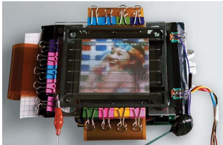
Samsung prototype field emission display using carbon nanotubes. Technology Review, November 2004 , May 2005
