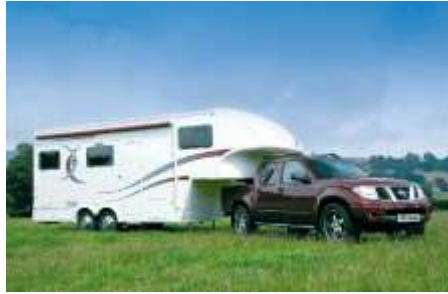
Figure 3: Photograph of a pick-up truck towing a trailer using a fifth wheel hitch.
