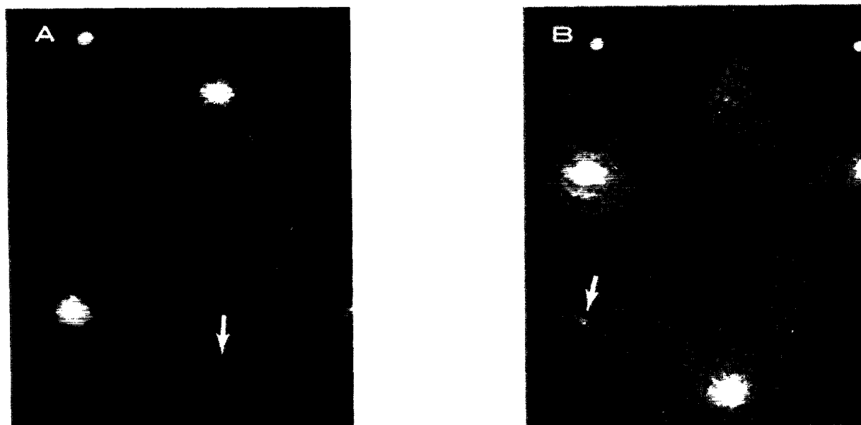
FIG. 1. Low-energy electron-diffraction pattern of the surface of a pure type- A oriented \text{NiSi}_2 layer and an essentially type- B layer with \sim 5\% of the area covered by type- A material. The intensity of the arrowed spots gives an indication of the percentage of area occupied by silicide of the opposite orientation.
