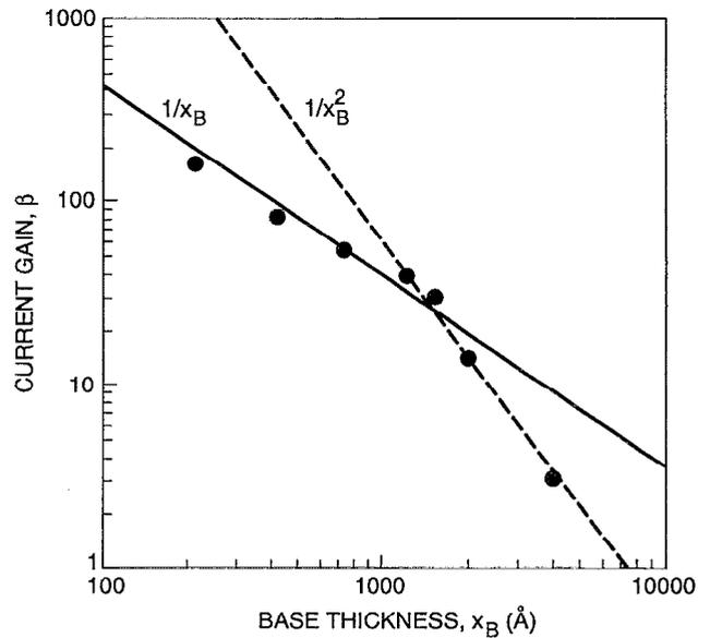
FIG. 2. Plot of measured room temperature common emitter current gain,  $\beta$ , as a function of base thickness,  $x_B$ , for  $I_C = 100 \mu\text{A}$  and  $V_{BC} = 0 \text{ V}$ . The broken line is the behavior expected for  $\beta \propto 1/x_B^2$  and the solid line is for  $\beta \propto 1/x_B$ .
