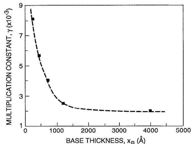
FIG. 3. Measured room temperature value of multiplication constant  $\gamma$  vs. base thickness  $x_B$  for abrupt junction  $\text{In}_{0.52}\text{Al}_{0.48}\text{As}/\text{In}_{0.53}\text{Ga}_{0.47}\text{As}$  HBTs.  $\gamma$  was obtained by measuring the variation in current from  $V_{CB} = 0.2$  to  $1.0 \text{ V}$ .
