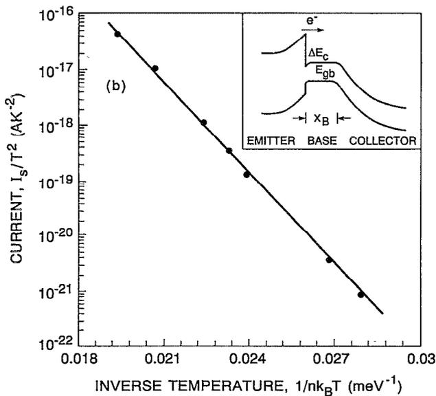
FIG. 1. (a) Measured room temperature Gummel plot for an  $\text{In}_{0.52}\text{Al}_{0.48}\text{As}/\text{In}_{0.53}\text{Ga}_{0.47}\text{As}$  HBT with  $x_B = 200 \text{ \AA}$ . (b) Measured temperature dependence of current  $I_S$  for  $V_{BC} = 0 \text{ V}$ . The inset shows a schematic of the band diagram of an abrupt  $\text{In}_{0.52}\text{Al}_{0.48}\text{As}/\text{In}_{0.53}\text{Ga}_{0.47}\text{As}$  n-p-n HBT under bias.
