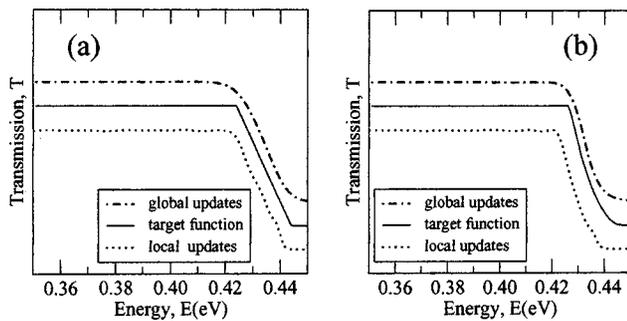
FIG. 4. Comparison of the adaptive global update and local random update algorithms in a system with 15+2+15 optical barriers: (a) linear target filter function and (b) parabolic target filter function. An offset of  $\pm 0.2$  has been introduced to simplify the comparison.
