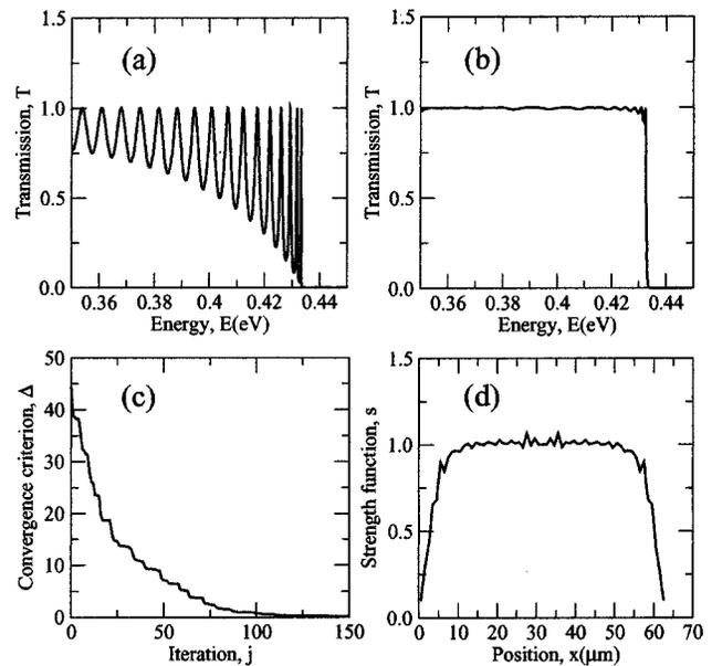
FIG. 2. Adaptive random updates on an array with  $30+2+30$  optical barrier pairs. (a) Transmission as a function of energy for the translationally symmetric case. (b) Transmission as a function of energy for broken spatial symmetry to achieve a cutoff filter function. (c) Deviation of  $T(E)$  from target function. (d) Corresponding strength function.
