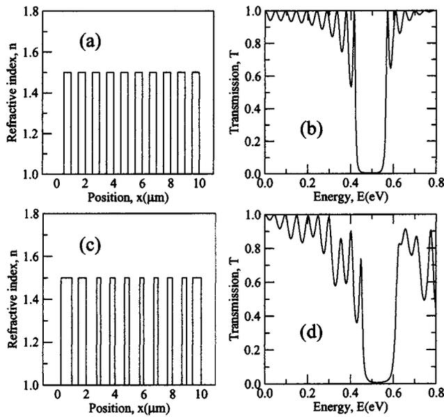
FIG. 1. Transmission as a function of energy in one-dimensional arrays of ten optical wells and barriers with alternating refractive indices  $n_1=1.0$  and  $n_2=1.5$ , respectively. (a) and (b) Symmetric array with barrier widths of  $0.5 \mu\text{m}$ . (c) and (d) Slightly randomized array with broken translational symmetry. The duty cycle is fixed at  $1 \mu\text{m}$ , whereas the widths are generated from a uniform random distribution function, centered at  $0.5 \mu\text{m}$ .
