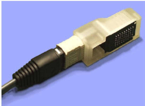
Figure 1.7: PONI module, now part numbers HFBR-712BP Tx VCSEL array or HFBR-722BP Rx GaAs PIN detector receiver array. The figure shows a single 12-wide transmitter module that can support data rates of 2.5 Gb/s per multimode fiber at 850 nm  $\lambda$  with low bit error ratio ( $BER < 10^{-14}$ ).
