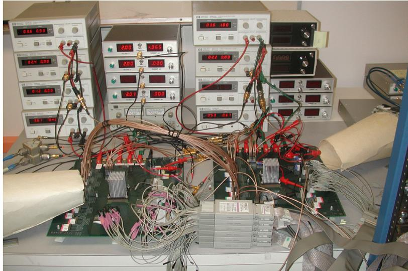
Figure 5.31: Photograph of two LAC chips connected in back-to-back configuration using 24" of RG178 copper microcoax electrical cables with 3M SCI stake assemblies. The power supplies used are visible in the background.
