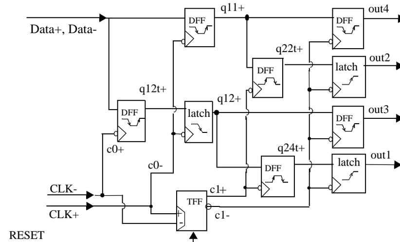
Figure 5.14: Schematic of half-speed 1:4 demultiplexer.
