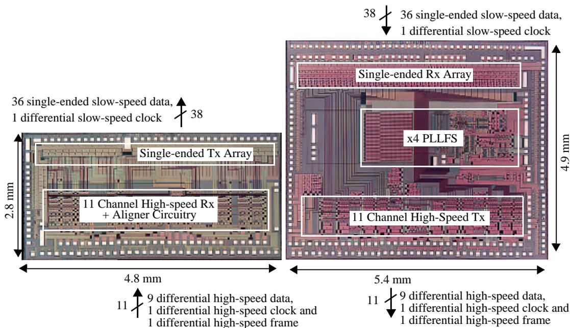
Figure 5.46: The ROPE DEMUX IC (**ropexh**), shown on the left-hand side is 4.8 mm x 2.8 mm and the ROPE MUX IC (**ropetxh**), shown on the right-hand side, is 5.4 mm x 4.9 mm.
