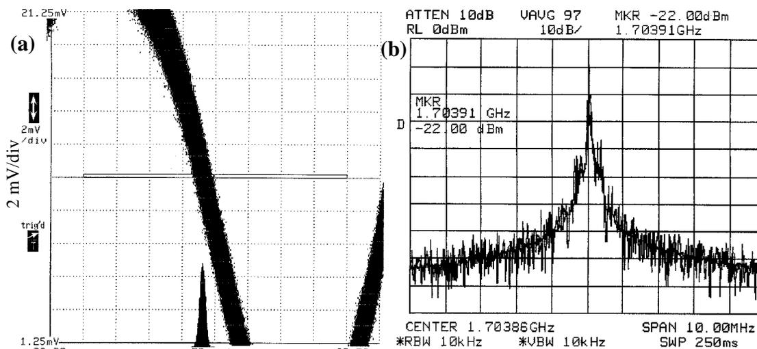
Figure 4.30: (a) Jitter histogram (self-referenced) of 1.7 GHz VCO output after 20 dB attenuation showing jitter of 4.46 ps rms (35 ps peak-to-peak). The horizontal scale is 50 ps/div and the vertical scale is 2 mV/div. (b) Spectrum analyzer output for 1.7 GHz output of T8 VCO with noise source **ni1** active.
