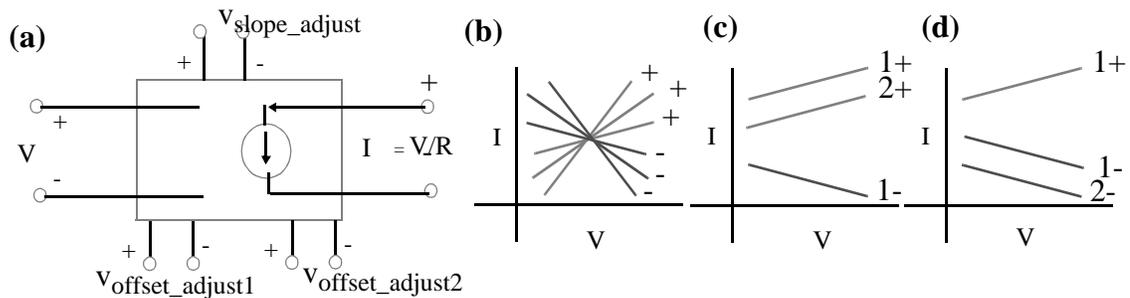
Figure 4.9: Linear two-port model of control stage.
