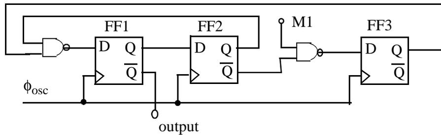
Figure 3.15: Schematic of 4/5 prescaler. M1 is the 4/5 control bit.
