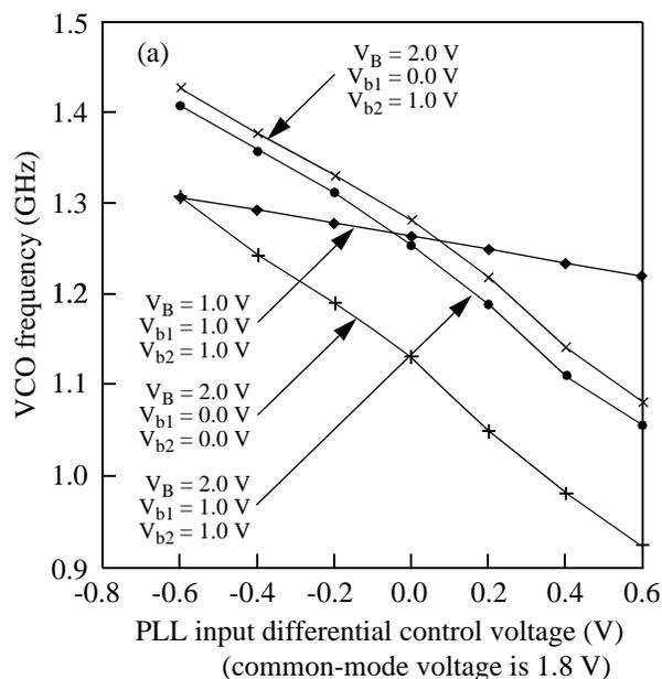
Figure 4.48: (a) Measured PLLFS VCO frequency variation with differential control voltage at different offset-control voltages ( $V_{b1}$ ,  $V_{b2}$ ) at slope control voltages  $V_B = 1.0$  V.
