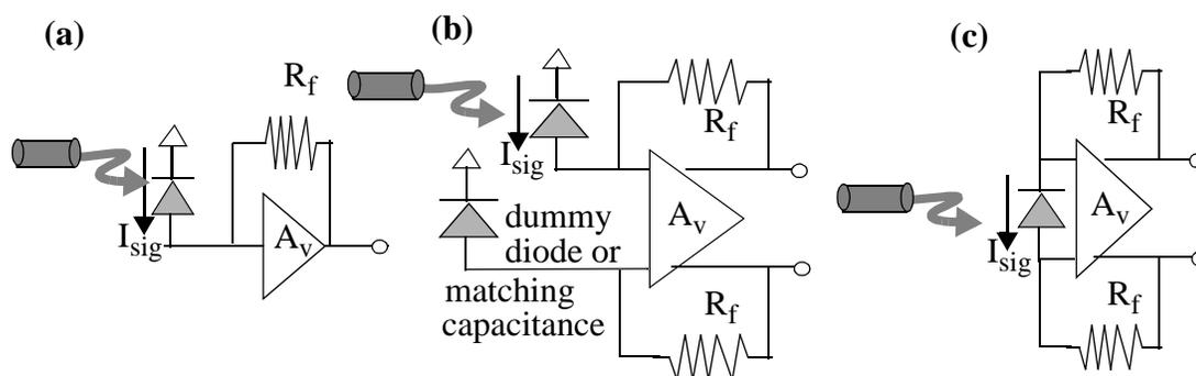
Figure 6.55: Schematic illustration of possible realizations of (a) single-ended and ((b) and (c)) differential receivers, all of which operate with light signal from a single fiber.
