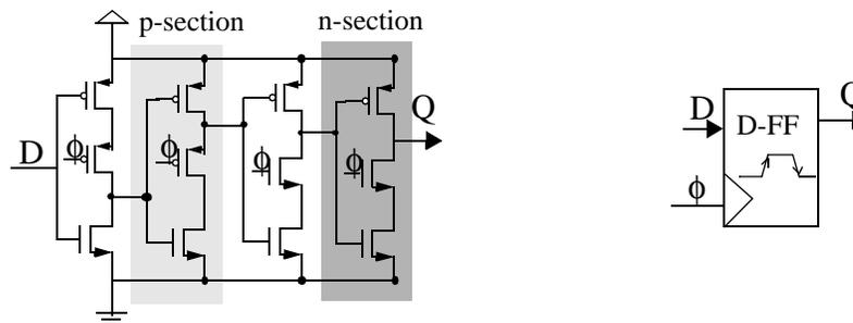
Figure 3.38: Schematic and symbol of a ppnn DFF.
