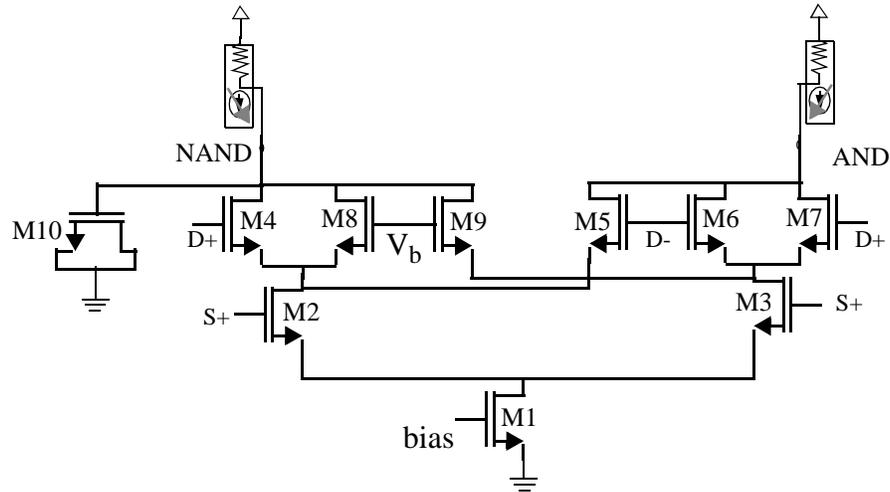
Figure 3.28: Schematic of balanced differential AND/NAND gate.
