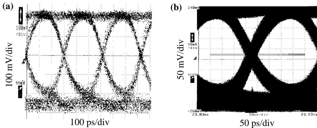
Figure 3.14: Measured (a) output eye-diagram and (b) output jitter of 9 ps rms (58 ps peak-to-peak) corresponding to 3.2 Gb/s operation of the full-speed flip-flop in Figure 3.12 for BER  $< 10^{-13}$ .
