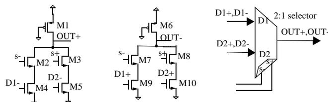
Figure 5.2: Schematic and symbol of 2:1 selector using pseudo-nmos style wired-or logic.
