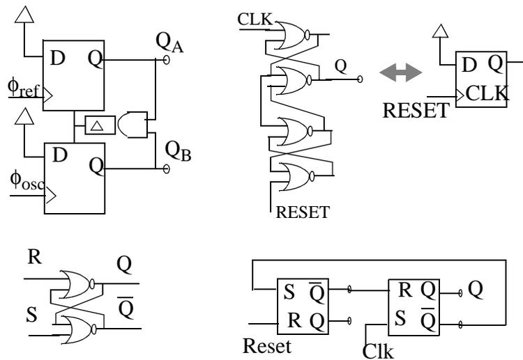
Figure 4.36: Digital Phase Frequency (sequential) Detector (DPFD)
