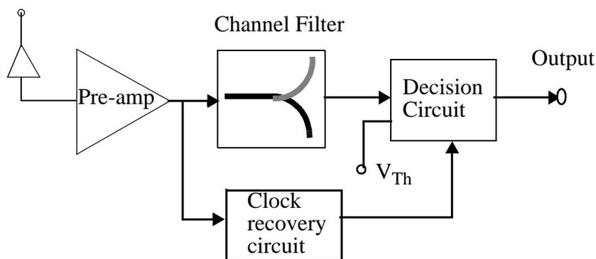
Figure 6.12: Block level diagram of synchronous optical receiver
