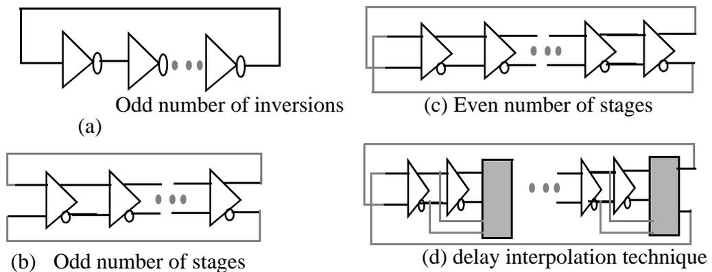
Figure 4.4: Single-ended and differential ring oscillator realization.
