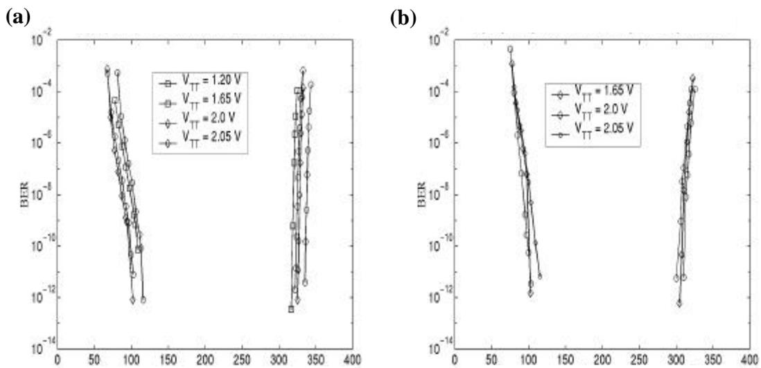
Figure 5.43: Variation of the high-speed input side clock-to-data phase-margin for (a) PDIN3 and (b) PCIN0, measured in electrical loopback. Squares, diamonds, circles and crosses correspond to input common-mode voltages of 1.20 V, 1.65 V, 2.0 V and 2.05 V respectively.
