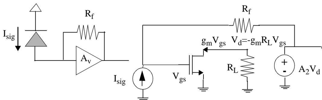
Figure 6.25: Elementary TIA and its equivalent small-signal model.
