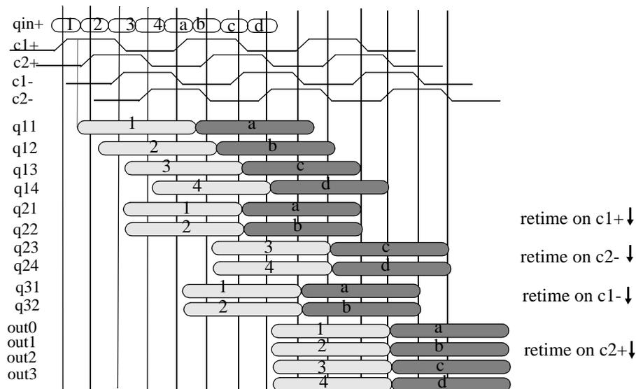
Figure 6.19: Schematic of waveforms at the various nodes in phase-aligner example in Figure 6.18.
