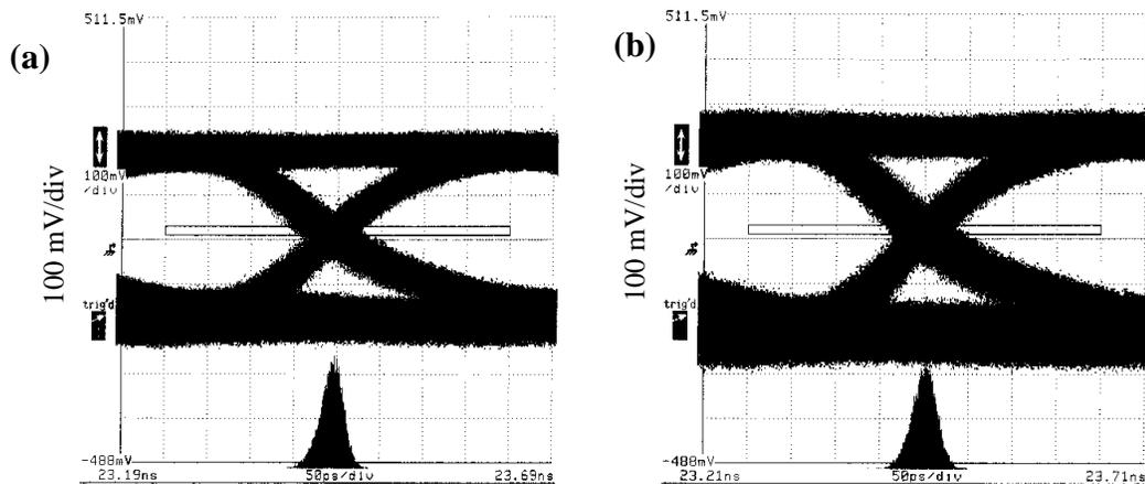
Figure 5.58: Source-referenced jitter statistics of (a) PDOUT3+ and (b) PDOUT7+. The horizontal scale is 50 ps/div for both (a) and (b).
