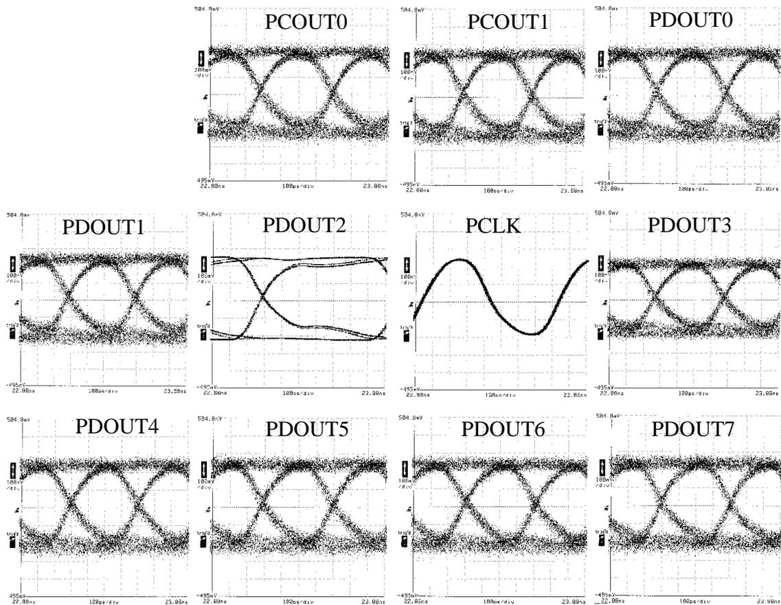
Figure 5.55: 2.5 Gb/s self-referenced (using the PLLFS trigger output as the oscilloscope trigger) eye-diagrams obtained at the positive high-speed mux output. The vertical scale is 100 mV/div and the horizontal scale is 100 ps/div for all plots.
