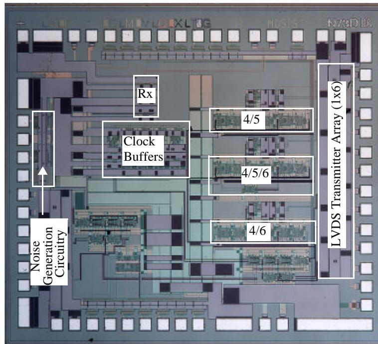
Testdie (T7) to measure performance of 4/5, 4/5/6 and 4/6 prescalers in 0.5  $\mu\text{m}$  CMOS technology. The IC measures 2.5 mm x 2 mm. Accounting for the bypass capacitors for each prescaler, the 4/5 prescaler occupies 213  $\mu\text{m}$  x 700  $\mu\text{m}$ , the 4/5/6 prescaler occupies 286  $\mu\text{m}$  x 700  $\mu\text{m}$  and the 4/6 prescaler occupies 215  $\mu\text{m}$  x 700  $\mu\text{m}$ . Each prescaler has an output buffer which is 105  $\mu\text{m}$  x 273  $\mu\text{m}$ .
