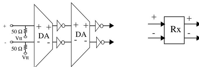
Figure 3.40: Schematic and symbol of the Clock Receive (Rx) Circuit.
