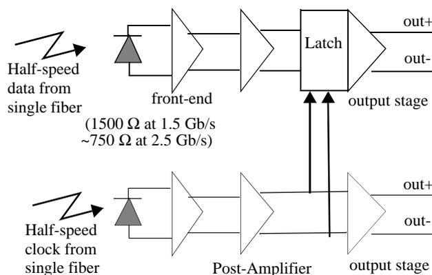
Figure 6.66: Schematic of latched TIA array.
