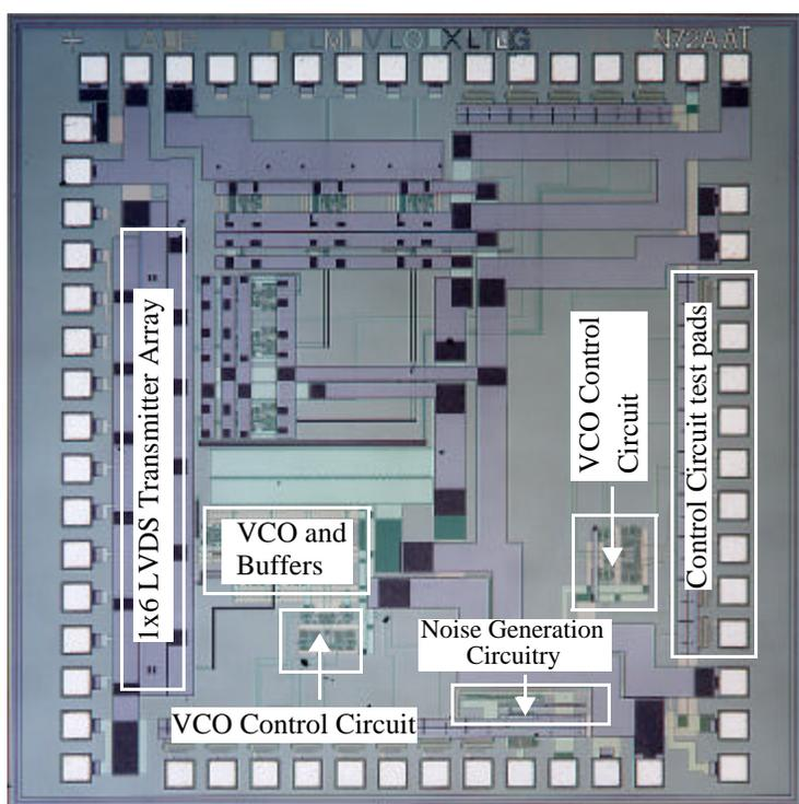
Testdie (T6) to measure performance of the VCO and control circuit. The IC measures 2.17 mm x 2.0 mm. Accounting for the bypass capacitors, the VCO occupies 354  $\mu\text{m}$  x 293  $\mu\text{m}$ , the control circuit, 173  $\mu\text{m}$  x 149  $\mu\text{m}$ .
