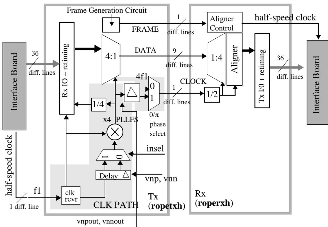
Figure 5.47: Block diagram of 4:1/1:4 mux/demux chipset (clock distribution circuitry details are not shown).
