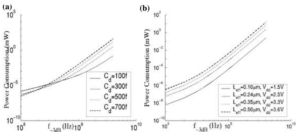
Figure 6.34: Variation of OE pre-amplifier power consumption with -3dB frequency of stage ( $=1.414 \cdot \text{Bitrate}$  assuming 3 stage overall amp).
