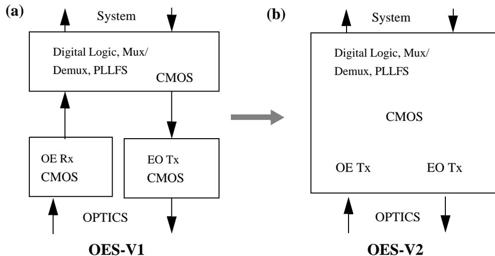
Figure 1.9: Migration path of opto-electronic link from OES-V0 to (a) OES-V1 and (b) OES-V2.
