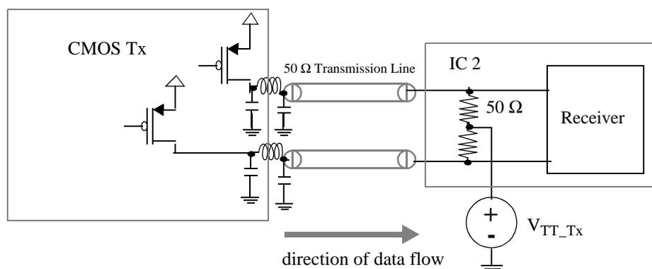
Figure 3.51: Schematic of the interface connection of 2.5 Gb/s LVDS CMOS Tx circuit. IC2 can be Si-Bipolar or future CMOS IC.
