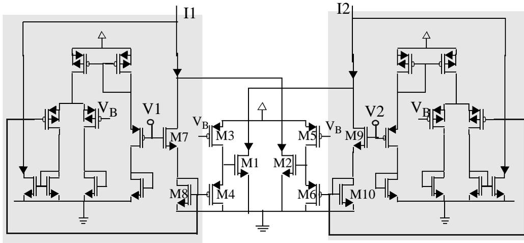
Figure 4.12: Complete rail-to-rail V-I converter core (load devices not shown).
