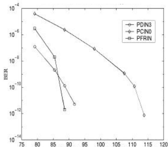
Figure 5.44: Variation of high-speed input sensitivity with BER for PDIN3, PCIN0 and PFRIN, measured in electrical loopback on the slow-speed side at an input common-mode voltage of 1.65 V.
