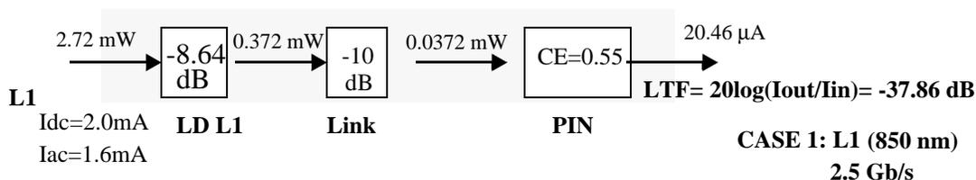
Figure 6.7: EO-OE LTF for typical OE data link with L1 and 10 db optical link-loss.
