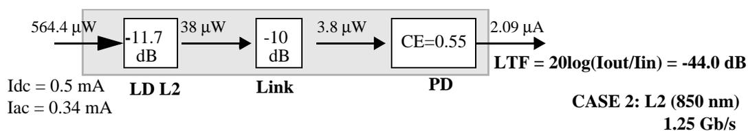
Figure 6.8: EO-OE LTF for a typical OE data link with L2 and 10 dB optical link-loss.
