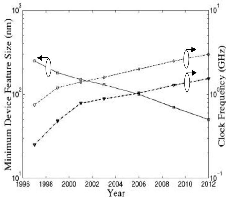
Figure 1.1: SIA 97 Roadmap indicating reduction in minimum device feature size (vertical axis on left side, squares), off-chip high performance multiplexed bus frequency (vertical axis on right side) (diamonds) and off-chip peripheral bus frequency (triangles).
