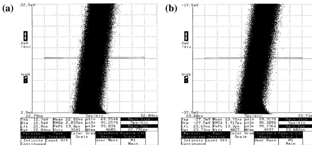
Figure 3.33: Trigger -pattern referenced (a) 4/5 prescaler jitter of 2.04 ps rms (13.8 ps peak-to-peak) and (b) 4/6 prescaler jitter of 1.92 ps rms (13.3 ps peak-to-peak).
