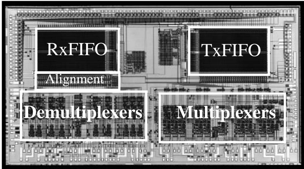
Figure 3.3: Die photograph of P2P link interface IC in 0.8  $\mu\text{m}$  CMOS process technology.
