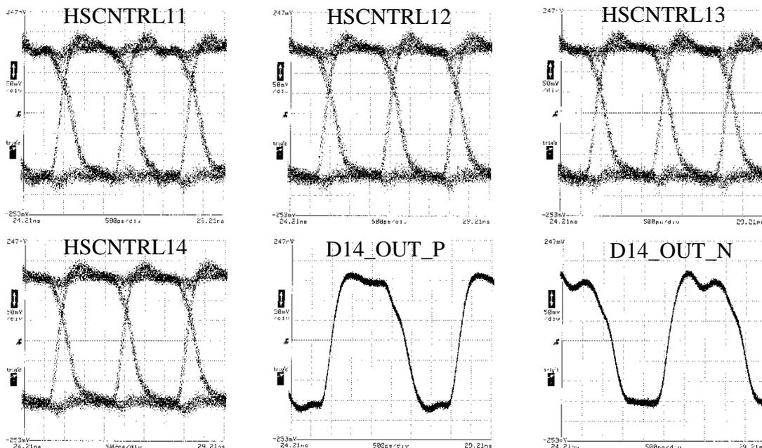
Figure 5.56: Representative demultiplexed eye-diagrams of PDIN7 at 625 Mb/s/channel at the slow-speed outputs of the **ropexh** IC in Figure 5.38. D14\_OUT\_P and D14\_OUT\_N correspond to the half-speed clock outputs of the **ropexh** IC. The horizontal scale for all plots is 500 ps/div and vertical scale is 50 mV/div for all plots.
