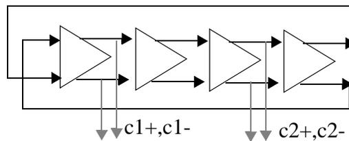
Figure 6.20: Example of differential ring oscillator with four stages to generate quadrature outputs in a PLLFS.
