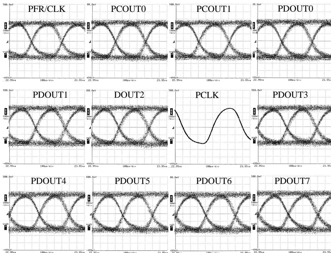
Figure 5.27: 2.5 Gb/s eye-diagrams measured at the positive high-speed output for  $2^{31} - 1$  NRZ PRBS input patterns at a BER  $< 5 \times 10^{-13}$ . The vertical scale is 100 mV/div and the horizontal scale is 100 ps/div for all plots.
