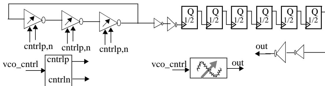
Figure 4.26: Schematic and symbol of single-ended noise oscillator.
