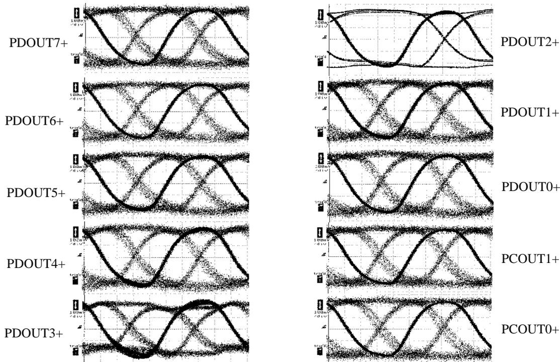
Figure 5.61: Overlaid high-speed data and clock eye-diagrams for each high-speed output corresponding to  $2^{31}-1$  NRZ PRBS patterns. The horizontal scale is 100 ps/div and the vertical scale is 100 mV/div for all plots.
