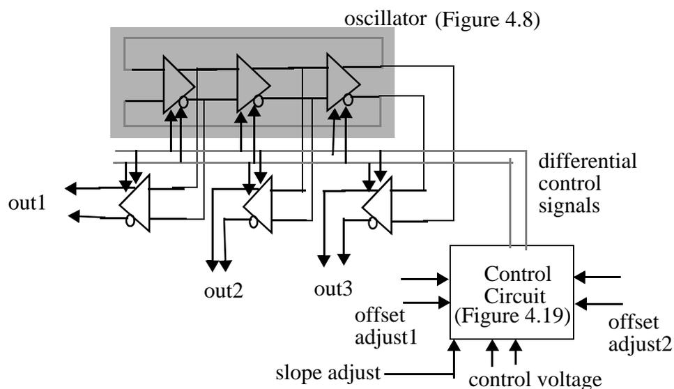
Figure 4.20: Schematic of VCO and control circuit that is simulated, fabricated and measured.
