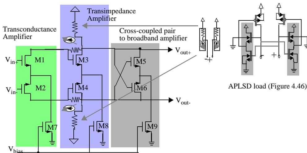
Figure 6.61: Schematic of Cherry-Hooper limiting amplifier with APLSD load (insert (Figure 3.10)) and cross-coupled pair to broadband the amplifier.
