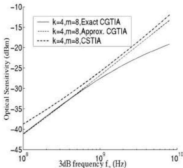
Figure 6.47: Plots of the full CGTIA sensitivity expression (Equation 6.99 and Equation 6.35) (solid line), full CSTIA sensitivity (Equation 6.91 and Equation 6.35) (dash dot line) and the CGTIA sensitivity expression without taking the CG pole into account.  $0.5 \mu\text{m}$  CMOS values of  $m = 8$ ,  $k = 4$ ,  $\omega_T = 44 \text{ Grad/s}$ ,  $A = 5$ ,  $\Gamma = 1.5$ ,  $\text{BER} < 10^{-13}$ ,  $C_d = 500 \text{ fF}$  and  $C_p = 0 \text{ fF}$  are used.
