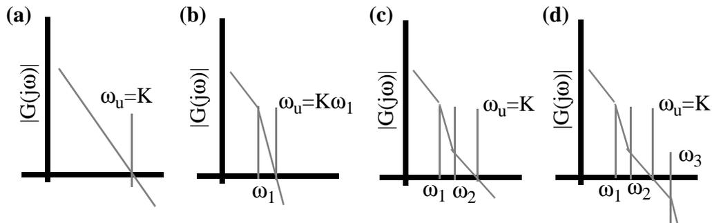
Figure 4.42: Bode plots of  $|G(j\omega)|$  for different loop-filters.
