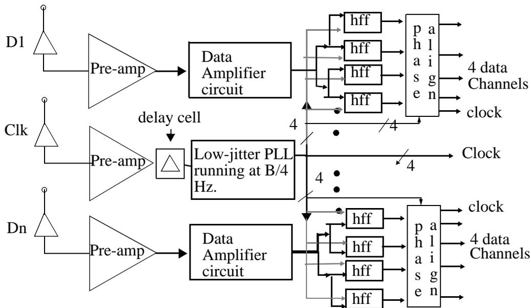
Figure 6.18: Half-speed OE receiver array schematic with synchronous receivers and a PLL in the clock channel, assuming the degree of demultiplexing to be 4 and B to be bit rate of each data channel.
