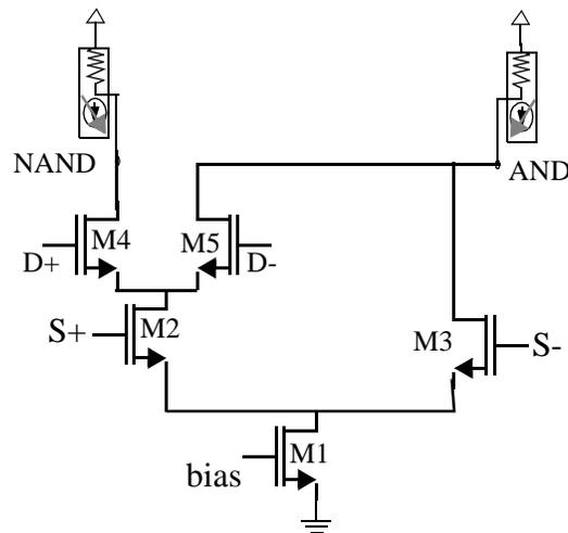
Figure 3.27: Schematic of differential AND/NAND gate.
