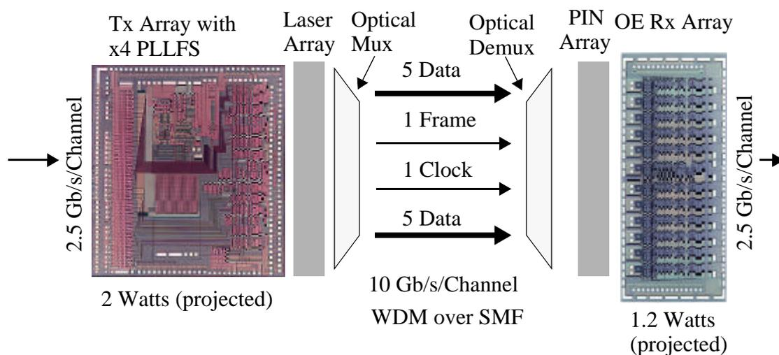
Figure 7.4: Proposed design point of 100 Gb/s Ethernet in 0.1  $\mu\text{m}$  CMOS process technology using WDM in SMF-ribbon with 12 wavelengths at 1300 nm center wavelength.
