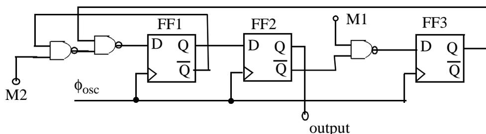
Figure 3.17: Schematic of the 4/5/6 prescaler. M1, M2 are the 4/5/6 control signals.
