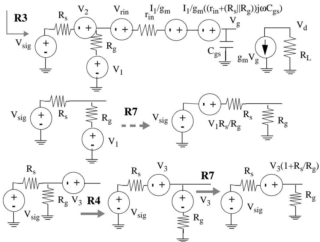
Figure 6.30: Transposition of all noise sources to the input.
