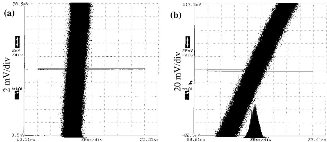
Figure 5.51: Measured self-referenced jitter of the high-speed clock output of the **ropetxh** IC (a) excluding the clock distribution network and delay-chain and (b) including all delay-chains and the clock-distribution network in PLLFS feedback loop. Horizontal scale is 20 ps/div for both (a) and (b).
