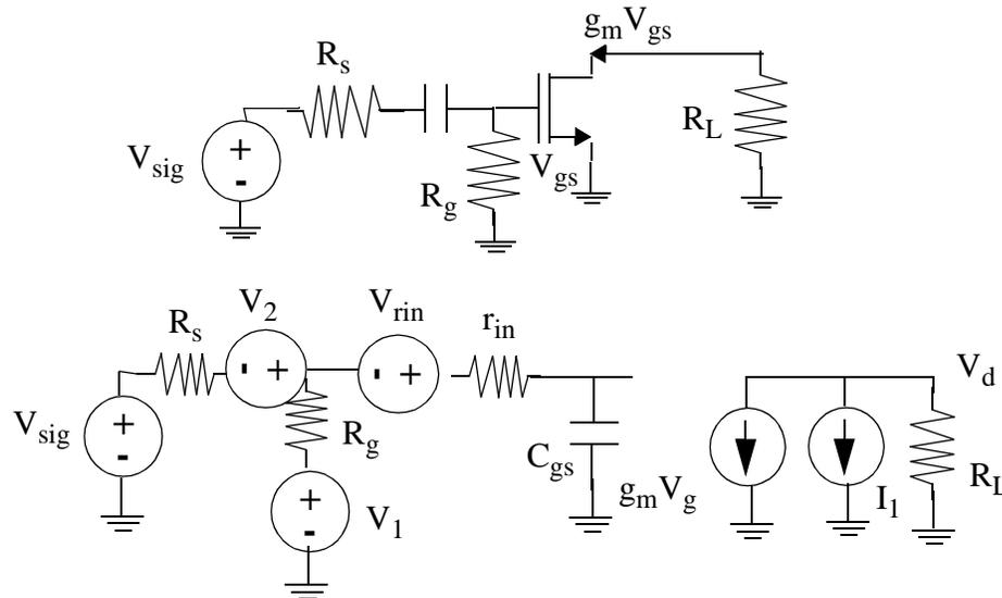
Figure 6.28: AC-schematic and small-signal model with noise sources of a CS amplifier.
