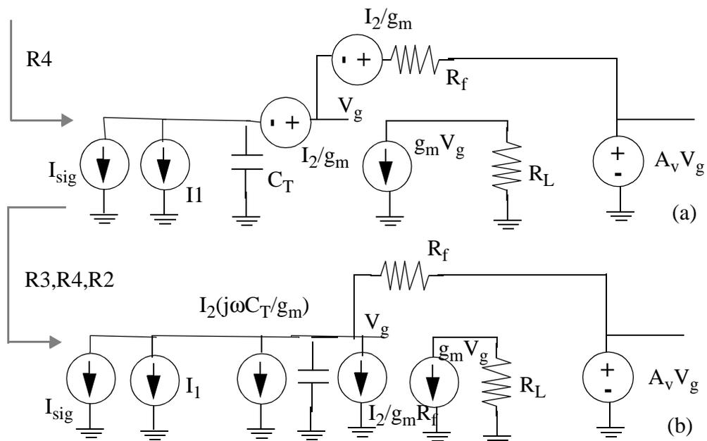
Figure 6.27: Small-signal model after transposition of  $I_2/g_m$  in Figure 6.26
