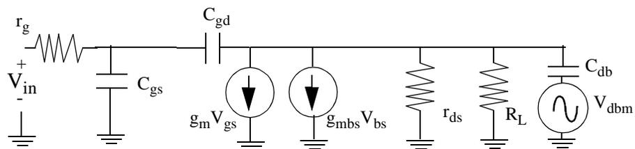
Figure 6.46: Small-signal model of the *open-loop* common-source amplifier in Figure 6.45.  $V_{dbm}$  is the noise source modulating the drain of the active transistor M1.
