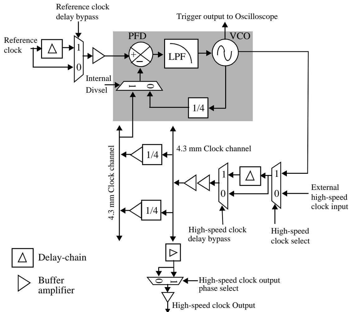
Figure 5.50: Schematic of the clock distribution circuit on **ropetxh** IC (Figure 5.49) which incorporates an integrated times-4 PLLFS circuit. The shaded area corresponds to the PLLFS core.
