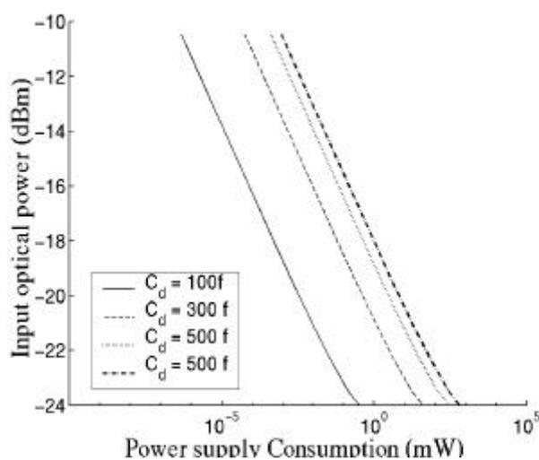
Figure 6.38: Power consumption variation (mW) with input stage sensitivity for desired stage bandwidth of 3.5 GHz, varying  $C_d$ ,  $L_{\text{eff}}$ ,  $V_{\text{dd}}$  and  $\Gamma$  with  $R_f = 1 \text{ K}\Omega$ .
