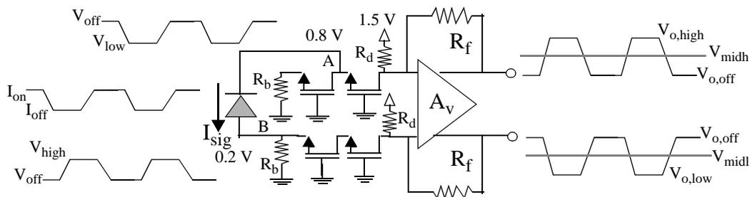
Figure 7.6: AC-schematic of differential CG receiver front-end.
