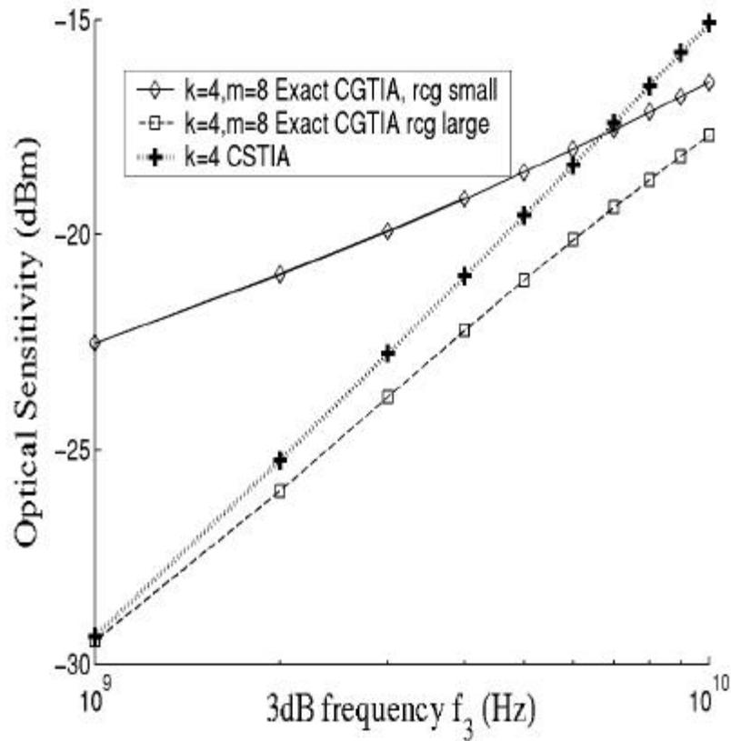
Figure 7.5: Optical sensitivity of a CS and CG receiver in 0.1  $\mu\text{m}$  CMOS with  $\eta=0.8$ ,  $\lambda = 1.3 \mu\text{m}$ ,  $f_T = 40 \text{ GHz}$ ,  $C_d = 300 \text{ fF}$ ,  $C_p = 100 \text{ fF}$ ,  $\Gamma = 2.5$ ,  $T = 358 \text{ }^\circ\text{K}$  and  $R_{d1} = 200 \Omega$ .
