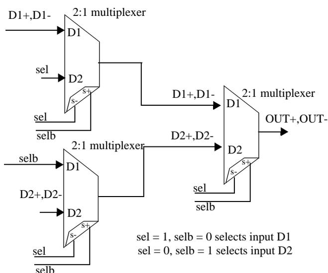
Figure 3.48: Schematic and symbol of low-jitter 2:1 clock select multiplexer.
