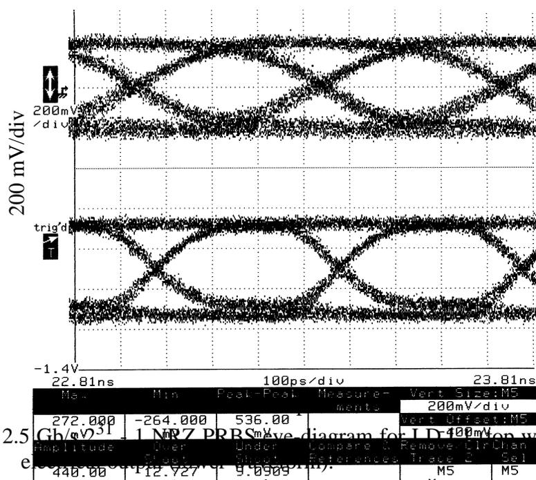
Figure 6.5: 2.5 Gb/s eye diagram for LD (top waveform) and electrical output (bottom waveform)
