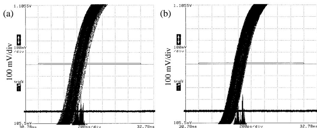
Figure 4.28: Jitter histogram of **ni1** at 14.83 MHz (950 MHz) with (a) **nsgnd** connected showing 49.24 ps rms jitter (240 ps peak-to-peak) and (b) **nsgnd** disconnected, with 46.53 ps rms jitter (200 ps peak-to-peak). The horizontal scale is 200 ps/div and the vertical scale is 100 mV/div for both (a) and (b).
