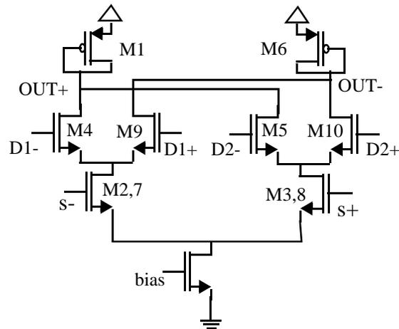
Figure 5.3: Schematic of differential 2:1 multiplexer
