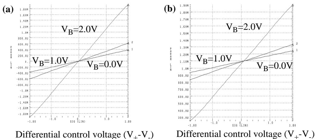
Figure 4.17: (a)  $I_p-I_n$  and (b)  $I_{po}-I_{no}$  for the revised LVIC for  $V_B=0\text{ V}$ ,  $1.0\text{ V}$  and  $2.0\text{ V}$ .
