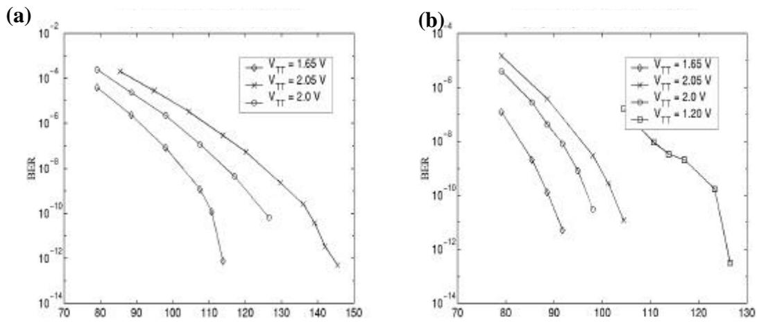
Figure 5.42: Variation of the high-speed differential input sensitivity with BER for different input common-mode voltages for high-speed input channels (a) PDIN3 and (b) PCIN0.
