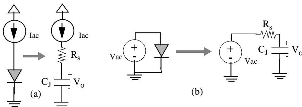
Figure 6.2: AC-schematic of VCSEL (a) current drive and (b) voltage drive.  $R_s$  is the VCSEL series resistance and  $C_J$  is the VCSEL capacitance.
