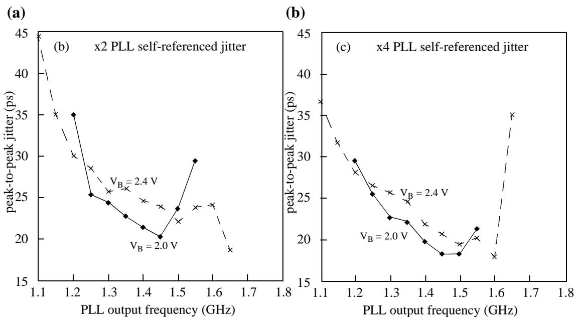
Figure 4.49: (a) and (b) are measured self-referenced jitter of the x2 and x4 PLLFS at two different VCO gain settings for 1.25 GHz.
