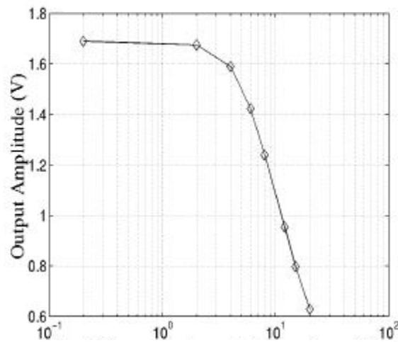
Figure 3.47: Simulated amplitude of clock channel waveforms of an array of three clock drivers (Figure 3.46) driving the capacitive loads (gate + wire) indicated on the x axis.
