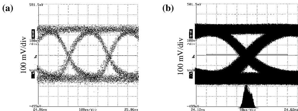
Figure 5.40: (a) Representative (PDOUT1+) high-speed output eye-diagram and (b) source-referenced jitter statistics of PDOUT1+ showing measured jitter of 16.31 ps rms (99 ps peak-to-peak). The horizontal scale is 100 ps/div for both (a) and (b).
