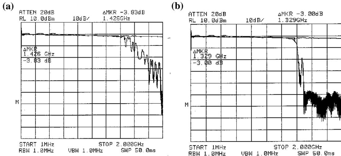
Figure 5.35: Insertion-loss measurements of the clk2 input to PCLKOUT path for input common-mode voltages of (a) 2.0 V and (b) 1.75 V.
