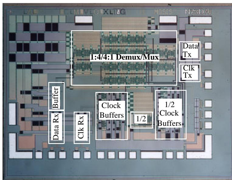
Die photograph of testdie (T9) to test 4:1/1:4 Mux/Demux. The testdie has an area of 2.4 mm x 1.67 mm in 0.5  $\mu$ m CMOS. IC implements BER circuit.
