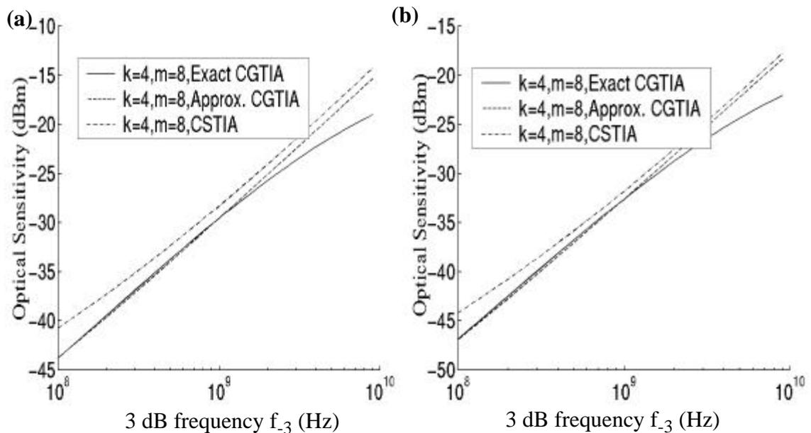
Figure 6.50: Plots of full CGTIA sensitivity expression (Equation 6.99 and Equation 6.35) (solid line), full CSTIA sensitivity (Equation 6.91 and Equation 6.35) (dotted line) and the CGTIA sensitivity expression without taking the CG pole into account (dash dot line) for  $0.1 \mu\text{m}$  CMOS process technology with  $m = 8$ ,  $k = 4$ ,  $f_T = 100$  GHz,  $C_p = 0$ ,  $\Gamma = 2.5$  and  $\text{BER} < 10^{-13}$  for the case of (a)  $C_d = 500$  fF and (b)  $C_d = 100$  fF.
