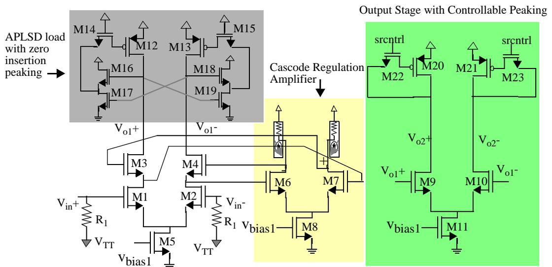
Figure 3.49: Schematic of controlled peaking amplifier implemented with regulated cascode amplifier input stage followed by output stage with controlled peaking implemented by the signal called srcntrl.
