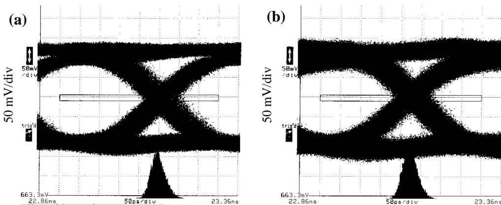
Figure 5.64: Source-referenced jitter statistics of the Rx module output of channel 1 and channel 6 in the optical loopback setup, with a BERT as the electrical data source driving the Tx module inputs. The horizontal scale is 50 ps/div and the vertical scale is 50 mV/div for both (a) and (b).
