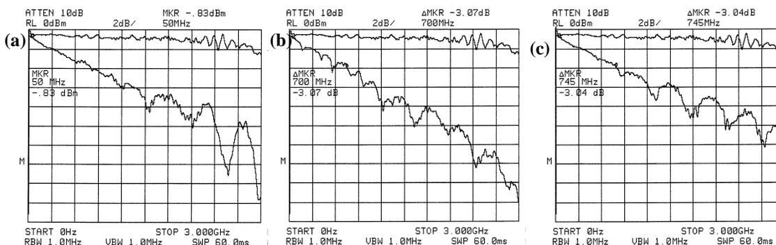
Figure 5.69: Insertion-loss measurement of (a) slow-speed side evaluation board, (b) slow-speed side to high-speed side evaluation board and (c) high-speed side evaluation board.
