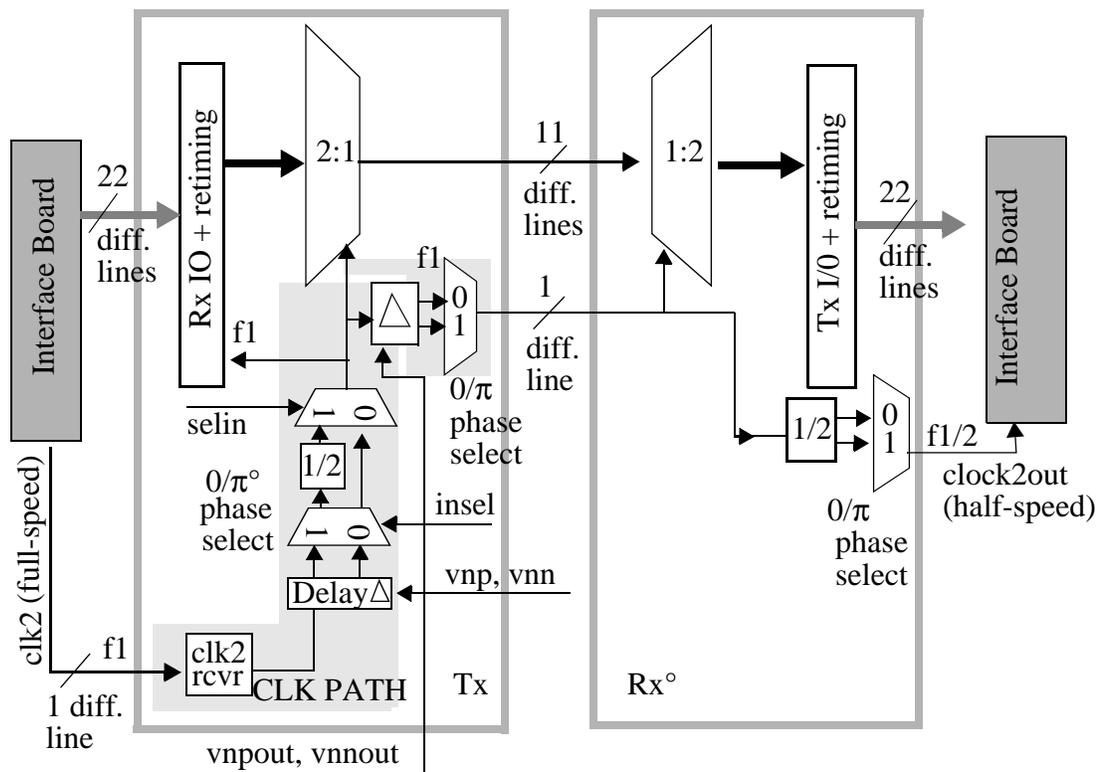
Figure 5.23: Block diagram of 2:1/1:2 mux/demux circuit with clock distribution circuit.
