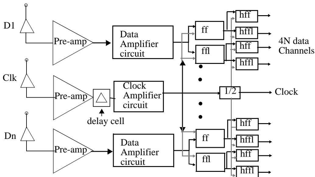
Figure 6.14: Half-speed optical receiver array schematic with synchronous receivers.
