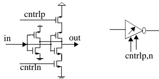
Figure 4.23: Schematic and symbol of delay cell of single-ended oscillator.
