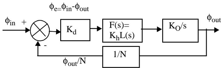
Figure 4.2: Linearized model of the PLLFS at lock.
