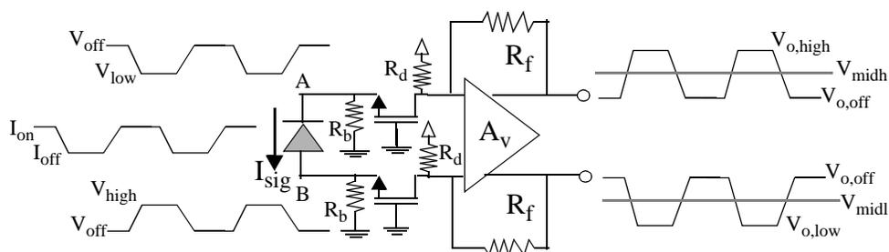
Figure 6.56: AC-schematic of the differential CG OE receiver.
