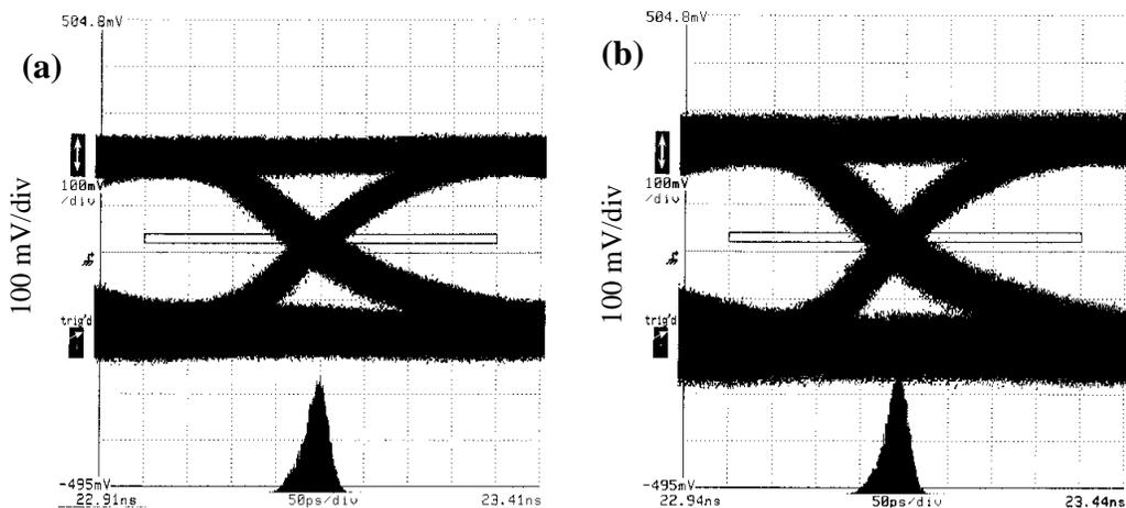
Figure 5.59: Self-referenced jitter statistics of (a) PDOUT3+ and (b) PDOUT7+. The horizontal scale is 50 ps/div for both (a) and (b).
