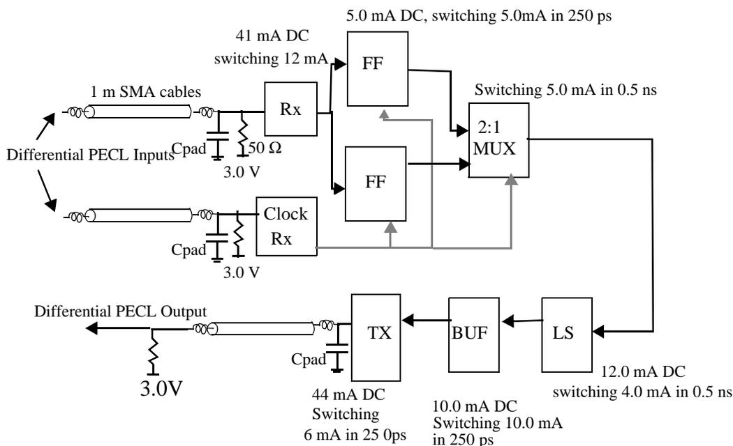
Figure 5.16:  $0.8\ \mu\text{m}$  CMOS BER circuit (T4) schematic.
