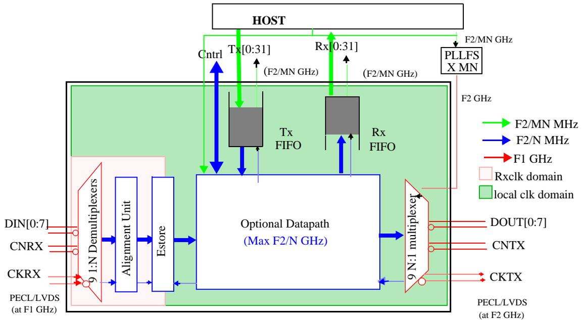
Figure 3.1: Block diagram of the POLO LA parallel data link.
