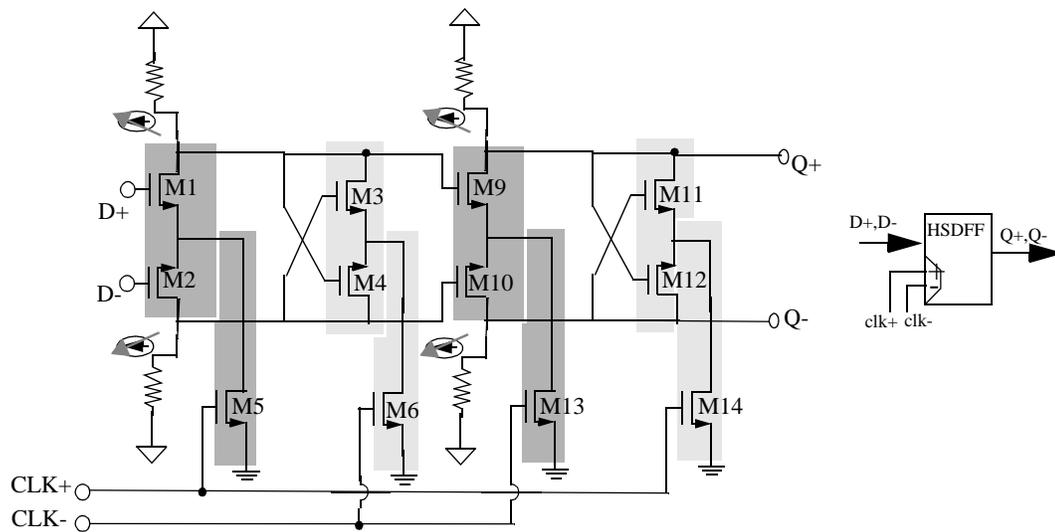
Figure 3.12: Schematic and symbol of high-performance CMOS differential master slave flip-flop. Load devices correspond to those in Figure 3.10.
