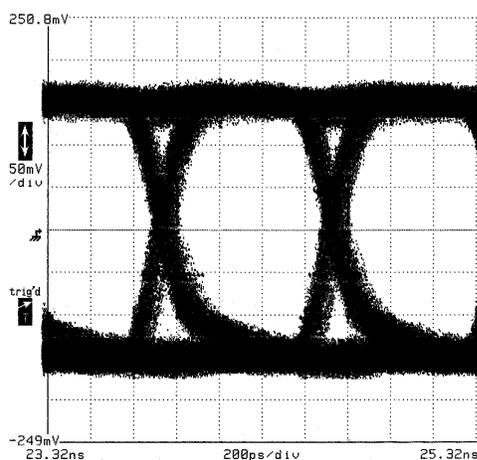
Figure 5.33: Composite eye-diagram of 22 slow-speed 1.25 Gb/s outputs. The vertical scale is 50 mV/div and the horizontal scale is 200 ps/div.
