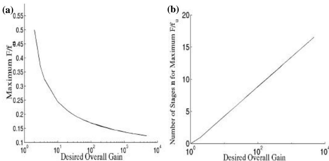
Figure 6.16: Variation of (a)  $F_{-3dBOverall}/f_u$  maximum with overall gain  $G_o$  and (b) number of stages  $n$  required to achieve it.
