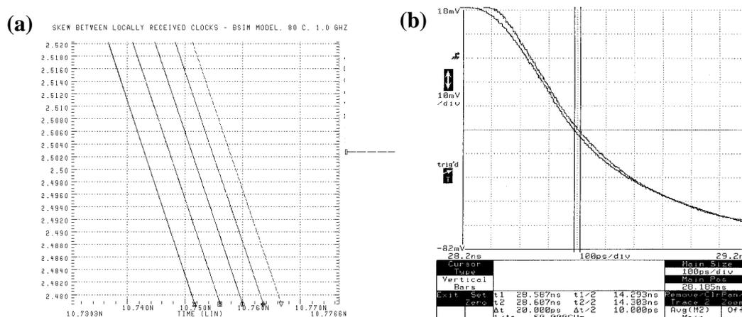
Figure 3.43: (a) Simulated and (b) measured results of the clock skew in the IC in Figure 3.42.
