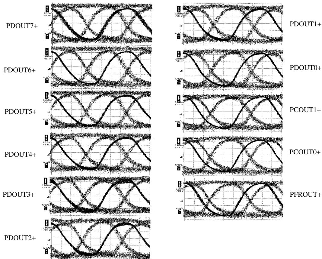
Figure 5.31: Overlaid high-speed data and clock (PCLK+) output eye-diagrams. The horizontal scale is 100 ps/div and the vertical scale is 100 mV/div for all plots.
