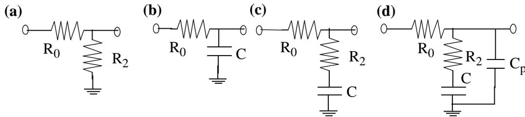
Figure 4.41: Possible loop-filter schematics from (a) simple attenuator to (d) third-order filter.
