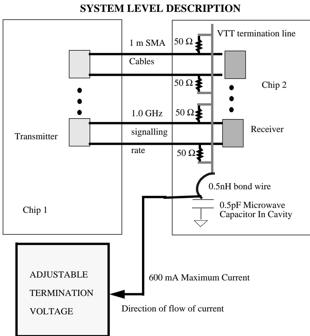
NOTE: ALL  $50 \Omega$  Resistors are on-chip resistors. Signalling is differential.
