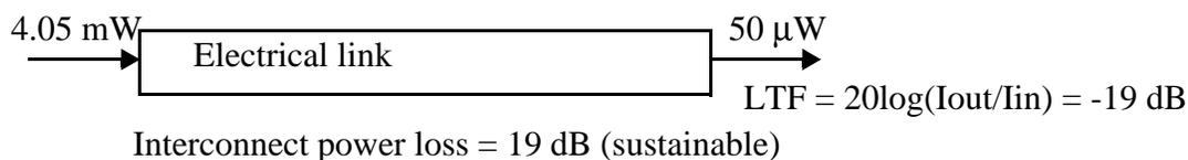
Figure 6.9: LTF of electrical link that can be supported by designed LVDS Rx-Tx circuitry in  $0.5 \mu\text{m}$  CMOS at 2.5 Gb/s.
