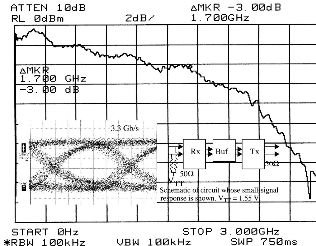
Figure 3.55: Insertion-gain measurement of CMOS Rx-Tx circuit on IC T8 with inset of 3.3 Gb/s eye-diagram corresponding to  $2^{31} - 1$  NRZ PRBS from the BERT and the schematic of the test circuit on IC T8. See text for details.
