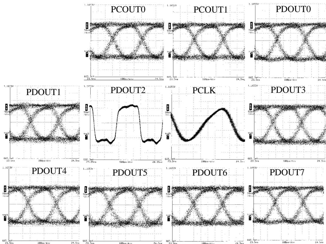
Figure 5.66: Source-referenced 2.5 Gb/s optical eye-diagrams measured (using the BERT trigger output as the oscilloscope trigger) at the positive high-speed optical Rx module outputs. The vertical scale is 50 mV/div and the horizontal scale is 100 ps/div.
