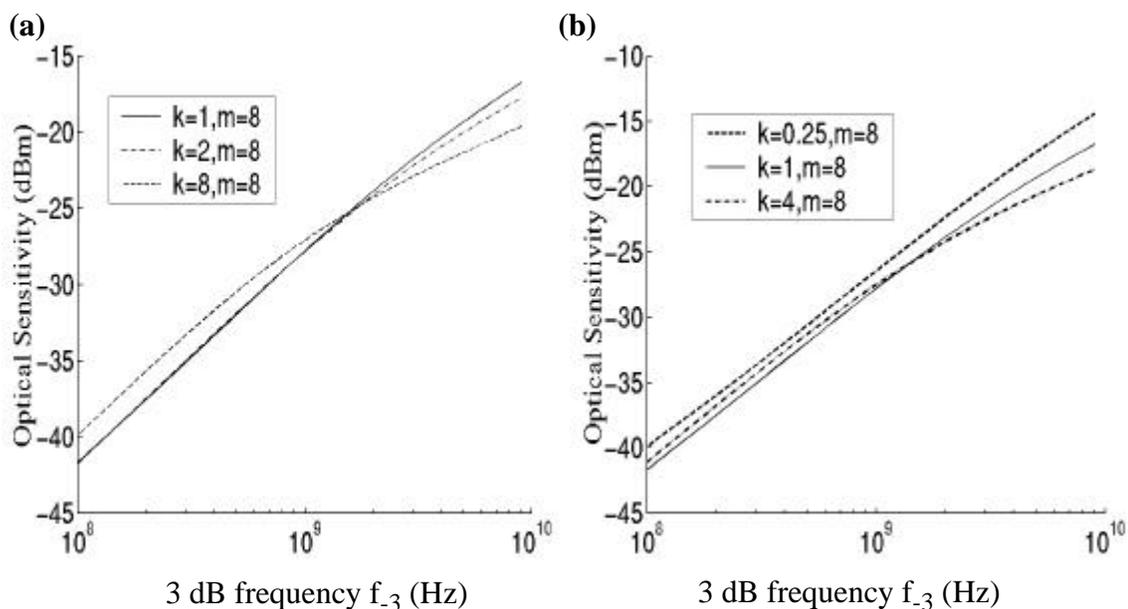
Figure 6.48: Plots of full CGTIA sensitivity expression (Equation 6.99 and Equation 6.35). (a) covers  $k = 1, 2, 4, 8$  for  $m = 8$  and (b) shows  $k = 0.25, 1, 4$  for  $m = 8$ .
