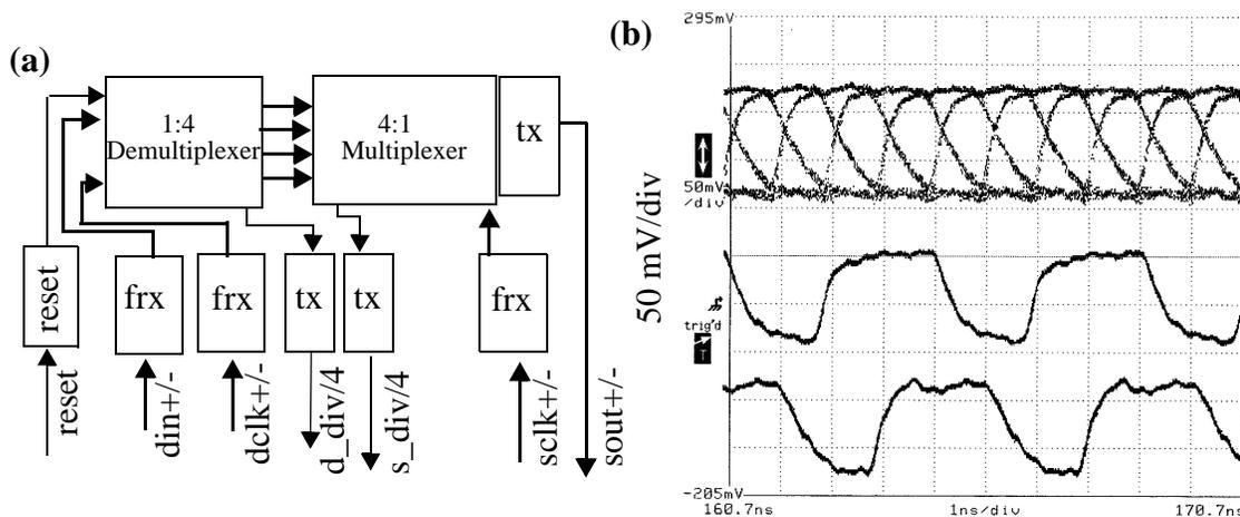
Figure 5.12: (a) Block diagram of 1:4/4:1 mux/demux BER circuit in  $0.8\ \mu\text{m}$  CMOS and (b) 980 Mb/s eye-diagram. The horizontal scale is 1 ns/div and the vertical scale is 50 mV/div.
