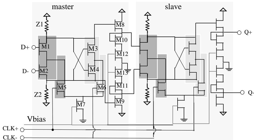
Figure 3.11: Schematic of high-speed differential master slave flip-flop in exotic process technologies such as Si/SiGe BJT, GaAs MESFET, InP/InGaAs HBT or AlGaAs/GaAs HEMT.
