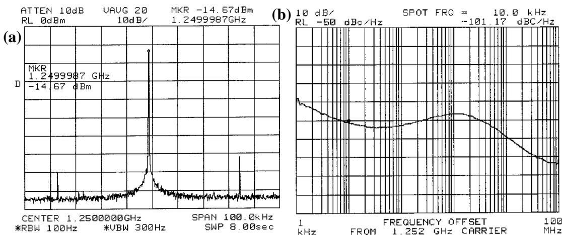
Figure 5.52: (a) Power spectrum of the high-speed clock output and (b) measured phase-noise of high-speed clock output showing phase-noise better than  $-101$  dBc/Hz at 10 KHz offset.
