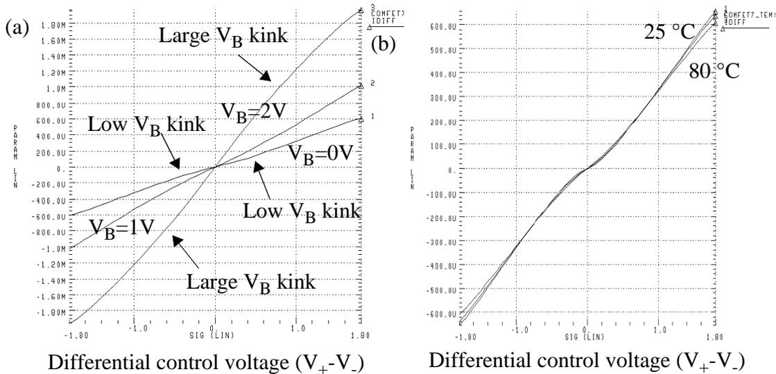
Figure 4.14: Current output of LVIC in Figure 4.13 (a) for different slope control voltages and for (b)  $25^\circ C$ ,  $45^\circ C$ , and  $80^\circ C$  for  $V_B = 1V$ .
