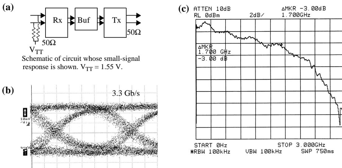
Figure 6.3: (a) Schematic of VCSEL driver circuit whose eye-diagram at 3.3 Gb/s corresponding to  $2^{31} - 1$  NRZ PRBS from the BERT is shown in (b). The measured insertion-gain is shown in (c). See text for details.
