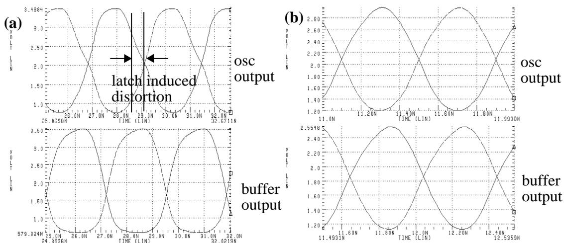
Figure 4.21: Simulated waveforms of the oscillator output at (a) 215 MHz and (b) 1.25 GHz using the slow process corner library decks at a junction temperature of 80 °C.
