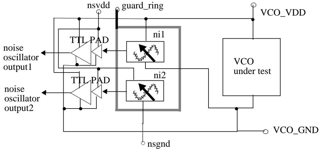
Figure 4.27: Schematic showing interaction of VCO under test with noise oscillator circuitry through power and ground connections.
