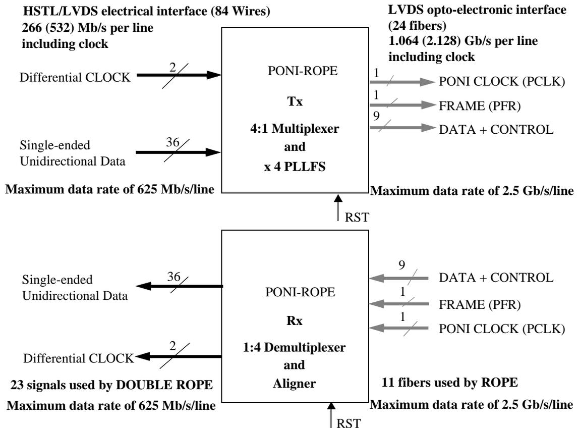
Figure 5.45: PONI ROPE MUX/DEMUX chipset block diagram.
