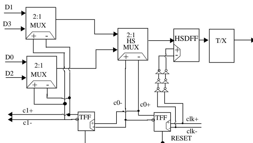
Figure 5.6: Schematic of full-speed 4:1 multiplexer composed of 2:1 muxes.
