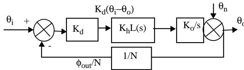
Figure 4.43: Linearized model of the PLLFS at lock with input and VCO noise sources.
