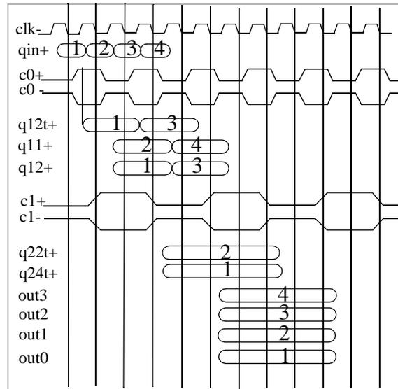
Figure 5.10: Schematic of waveforms at the various nodes in Figure 5.9.
