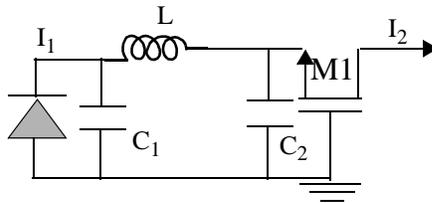
Figure 6.54: AC-schematic of single-ended CG OE receiver front-end.
