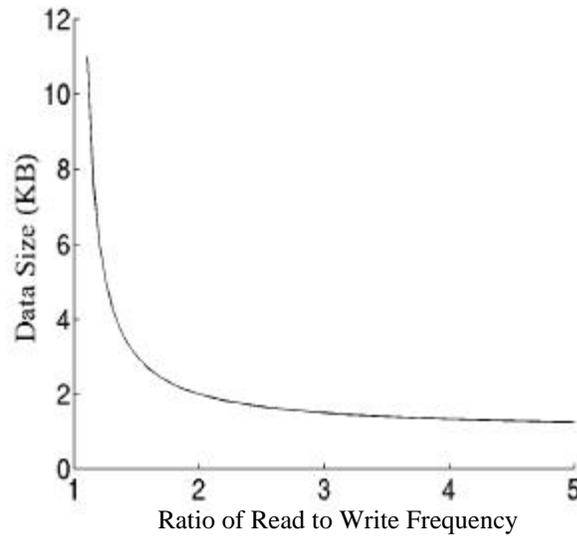
Figure 1.11: Variation of data size P (normalized to KB) with ratio of write frequency to read frequency.
