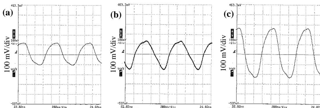
Figure 5.39: Plots of the different half-speed clock inputs that were used to determine the robustness of the high-speed input interface in slow-speed loopback. Results are tabulated in Table 5.2. The horizontal scale is 200 ps/div for (a), (b) and (c).
