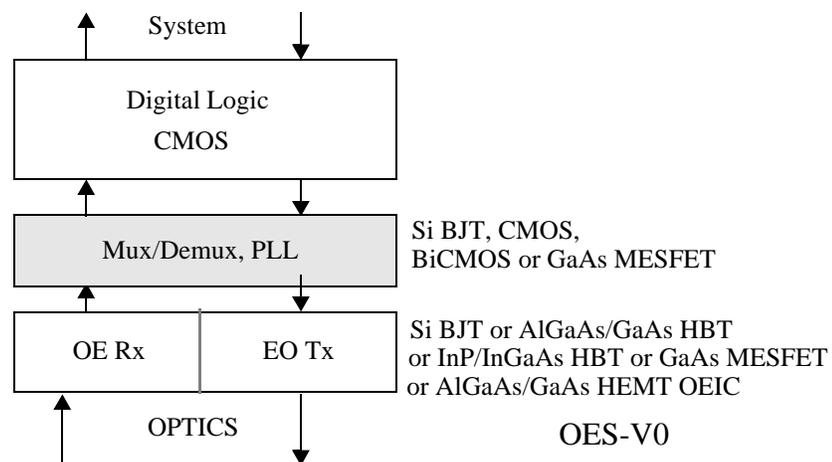
Figure 1.8: Block diagram of a general Opto-Electronic System Version 0 (OES-V0).
