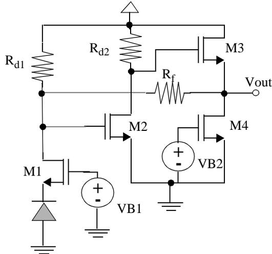
Figure 6.33: Schematic of a CGTIA.
