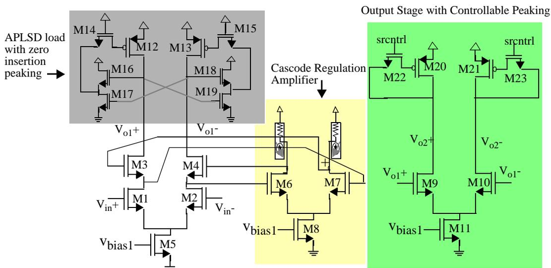
Figure 6.62: Schematic of controlled-peaking amplifier implemented with regulated cascode amplifier input stage followed by output stage with controlled zero insertion by control signal srcntrl.
