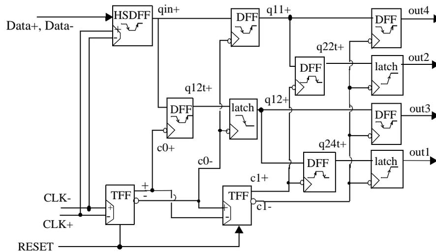
Figure 5.9: Schematic of the full-speed 1:4 demultiplexer.
