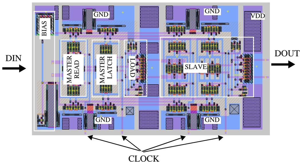
Figure 3.21: Layout of 1.6 GHz D flip-flop for prescaler.
