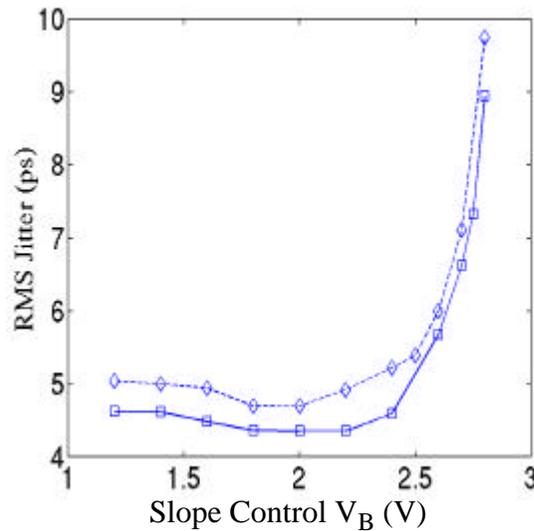
Figure 4.46: Variation of the x4 PLLFS self-referenced output rms jitter with slope control  $V_B$  at two different offset-control settings. Squares correspond to  $V_{y1p,n} = (0 \text{ V}, 3.6 \text{ V})$ ,  $V_{y2p,n} = (3.0 \text{ V}, 0.6 \text{ V})$  and diamonds to  $V_{y1p,n} = (1.2 \text{ V}, 2.4 \text{ V})$ ,  $V_{y2p,n} = (1.8 \text{ V}, 1.8 \text{ V})$ .
