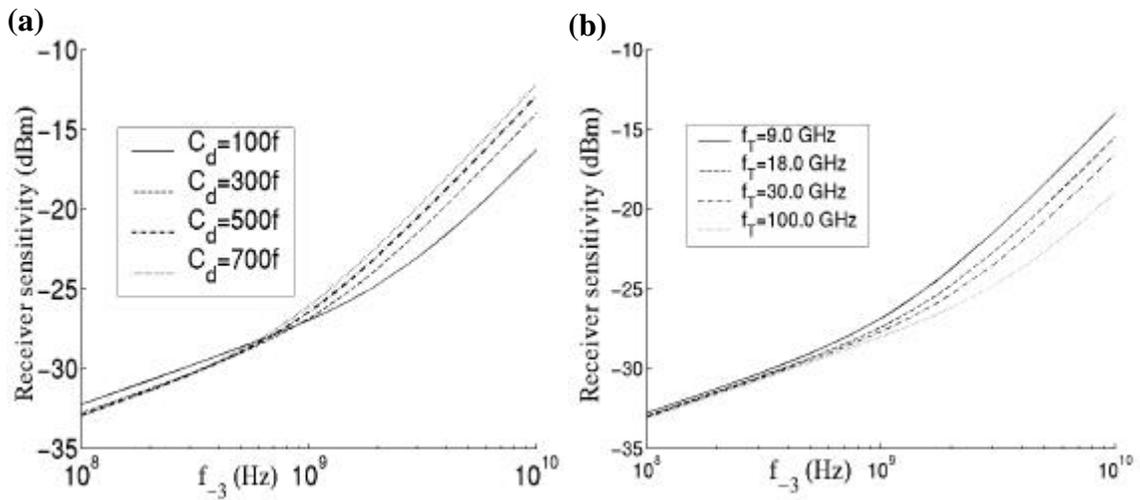
Figure 6.35: Receiver input sensitivity variation with input stage bandwidth in  $0.5 \mu\text{m}$  CMOS process technology,  $\text{BER} < 10^{-13}$ ,  $\Gamma=1.5$  for varying (a)  $C_d$  and (b)  $f_T$ .
