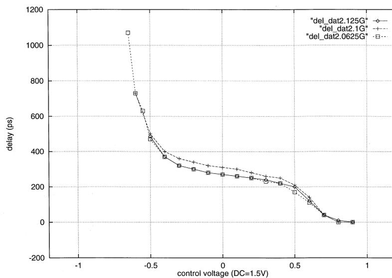
Figure 5.37: Measured delay characteristic on the high-speed clock output delay chain for a common-mode voltage of 1.5 V on the control voltage.
