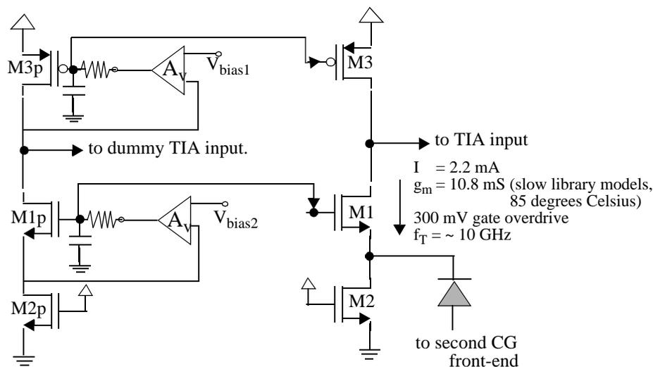
Figure 6.57: Schematic illustration of bias servoing using a dummy amplifier.
