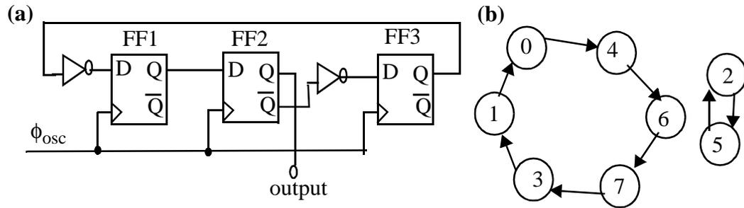
Figure 3.18: Schematic of 4/5/6 prescaler in divide-by-6 mode and its associated state diagram.
