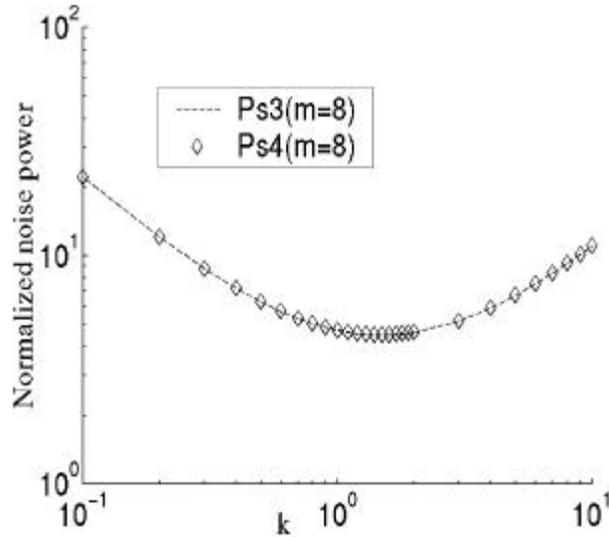
Figure 6.44: Plots of Equation 6.80 (solid line) and modified Equation 6.82 (diamonds) for values of  $\beta = 0.9$  with  $m = 8$ . Diamonds correspond to the corrected expression with CG pole accounted for  $f_{-3dB} = 2$  GHz and  $f_T = 9.0$  GHz.
