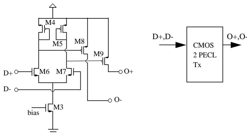
Figure 3.50: Schematic and symbol of differential CMOS2PECL Transmit (Tx) circuitry
