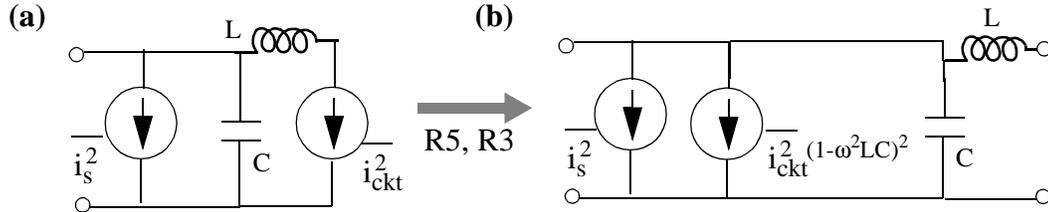
Figure 6.53: Schematic illustration of the influence of the front-end inductor on the input-referred noise-current PSD  $i_{\text{ckt}}^2$ . The transposition is achieved by using rules R5 and R3 described in Figure 6.23.
