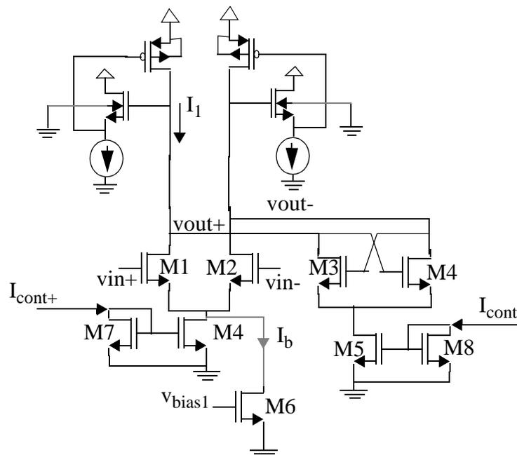
Figure 4.7: Differential delay cell with local positive feedback [135].
