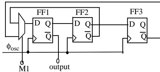
Figure 3.19: Schematic of 4/6 prescaler. M1 selects the mux between divide-by-4 and divide-by-6 modes.
