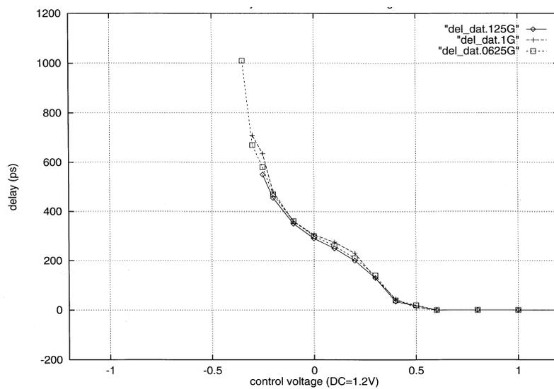
Figure 5.36: Measured delay characteristic on the high-speed clock output delay chain for a common-mode voltage of 1.2 V on the control voltage.
