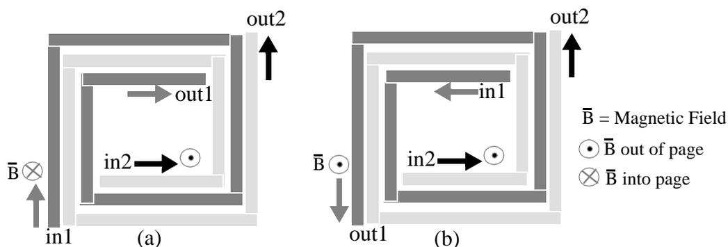
Figure 6.58: Coupled planar transformer to increase effective inductance by negative mutual coupling (a) and positive mutual coupling (b).
