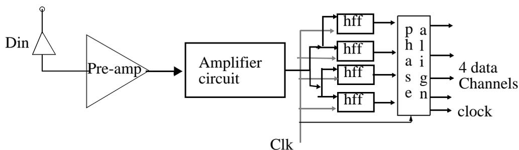
Figure 6.21: Half-speed optical receiver schematic with synchronous receiver, assuming degree of demultiplexing to be 4.
