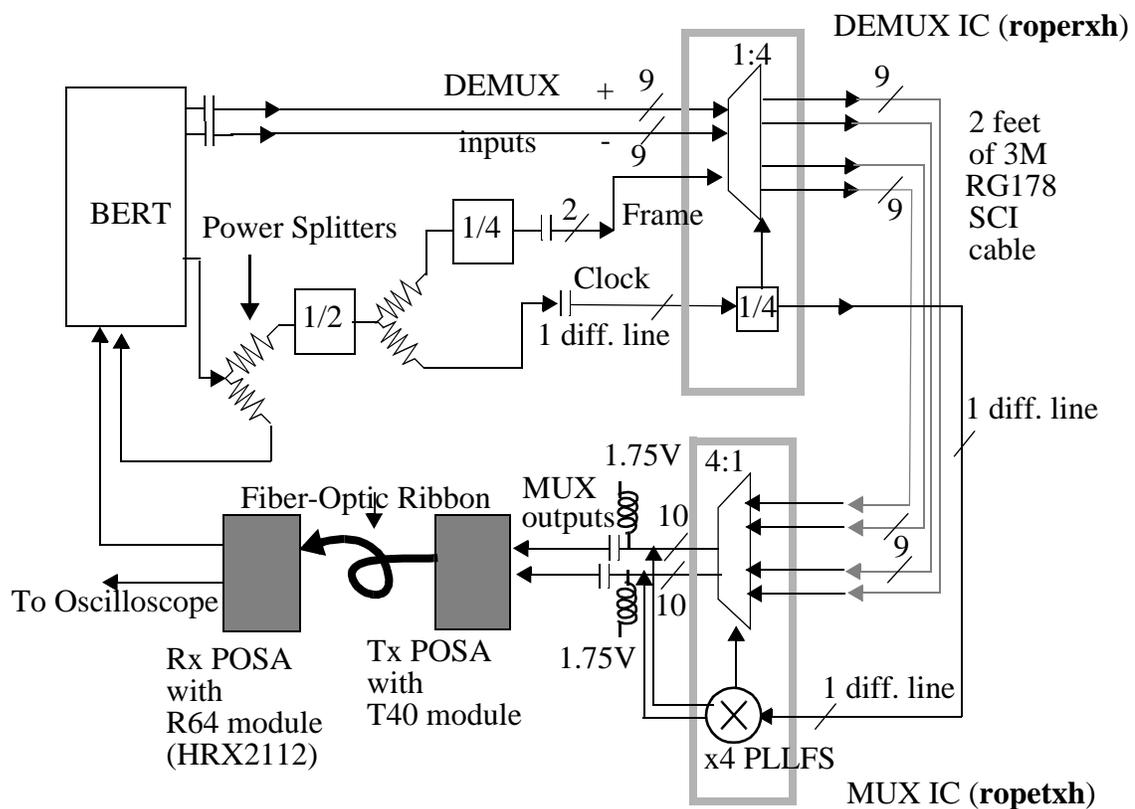
Figure 5.65: Schematic of the slow-speed loopback setup with optical loopback using the Agilent parallel optical Tx and Rx modules driven by the high-speed output of the **ropetxh** IC. Note that all the BER measurements are source-referenced.
