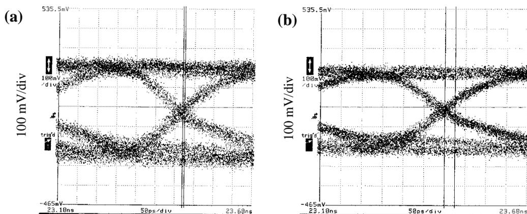
Figure 5.62: Skew (a) of 5 ps the outermost channels PDOUT7 (not displayed in panel) and PCOUT0 and (b) 25 ps between the outermost channel PCOUT0 (not displayed in panel) and the innermost channel PDOUT3. The horizontal scale is 50 ps/div for both (a) and (b).
