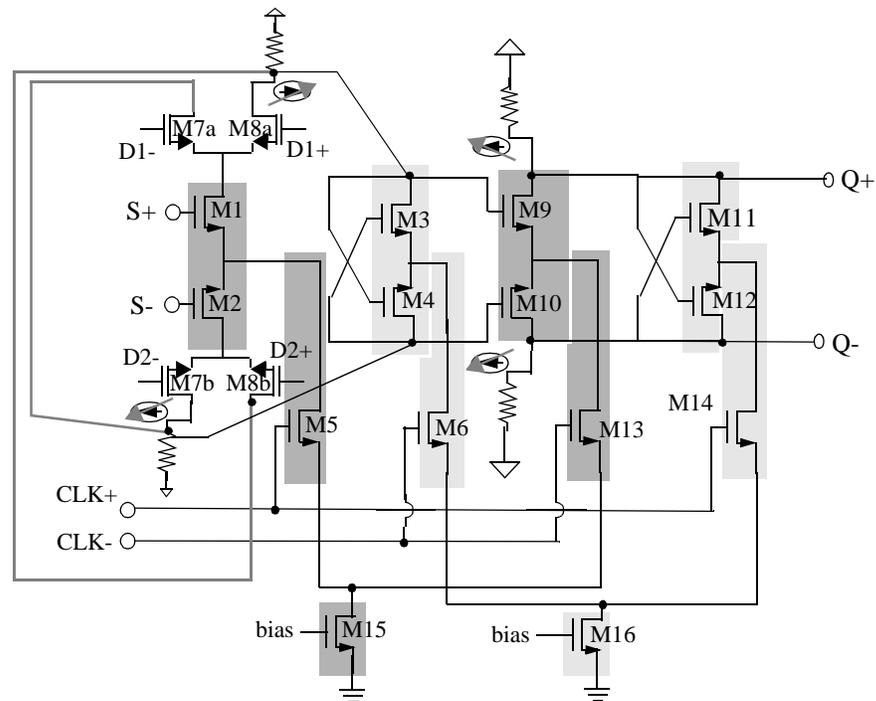
Figure 3.29: Schematic of differential master slave flip-flop with merged mux in master latch.
