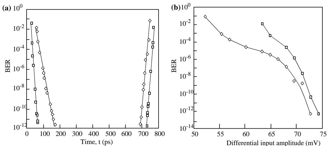
Figure 5.34: Measured slow-speed side (1.25 Gb/s, 800 ps bit-period) (a) best-case (squares) and worst-case (diamonds) output phase-margin and (b) best-case (diamonds) and worst-case (squares) input sensitivity.
