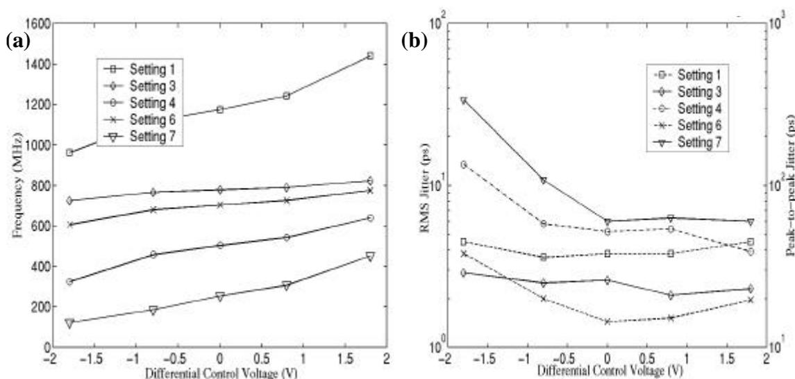
Figure 4.32: (a) Measured T8 VCO frequency and (b) self-referenced rms jitter corresponding to each setting in (a). Note that the on-chip noise source **ni1** is active during the measurements,
