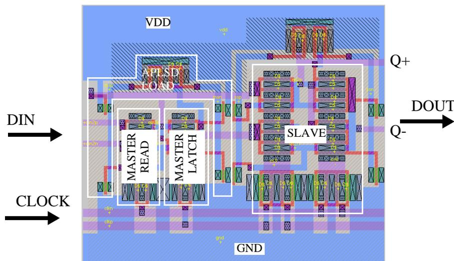
Figure 3.22: 1.25 Gb/s data flip-flop with 52 drawn devices occupying an area of  $58.2 \mu\text{m} \times 69 \mu\text{m}$ .
