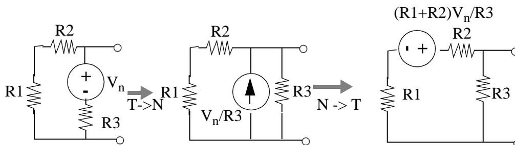
Figure 6.24: Rule R7: pushing a voltage through a resistive divider.
