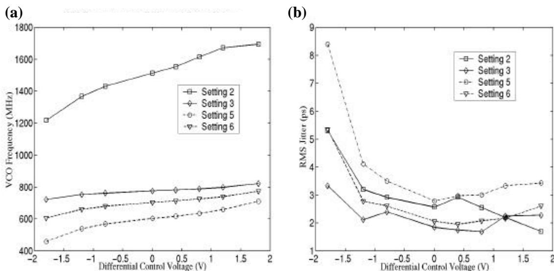
Figure 4.33: Measured T8 VCO (a) frequency and (b) self-referenced rms and peak-to-peak jitter corresponding to each setting in (a). Note that the on-chip noise source **ni1** is active during the measurements.
