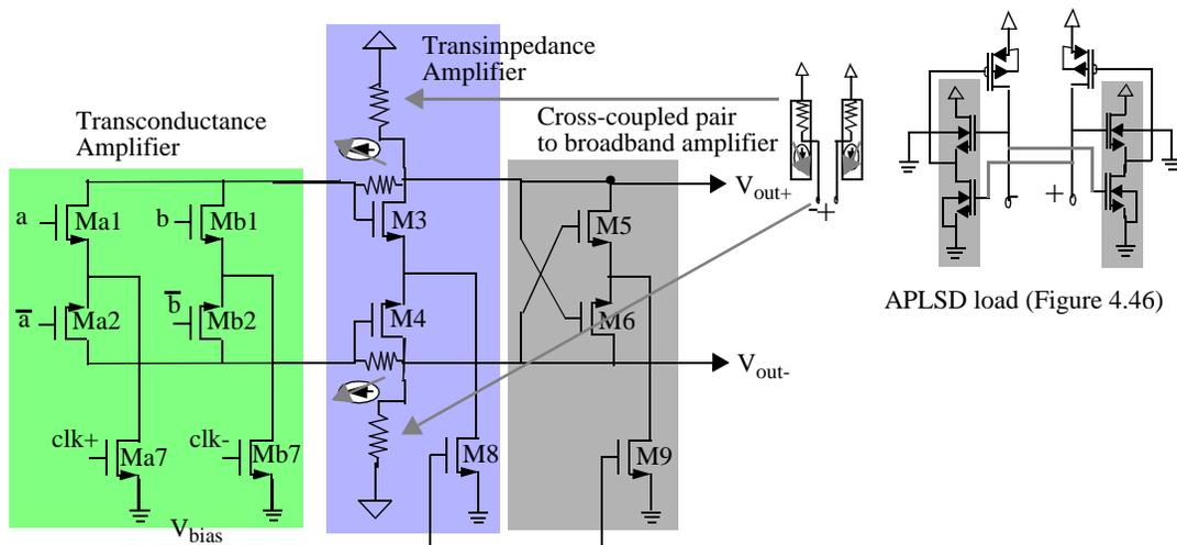
Figure 6.64: Schematic of merged 2:1 multiplexer and limiting amplifier in Figure 6.61.
