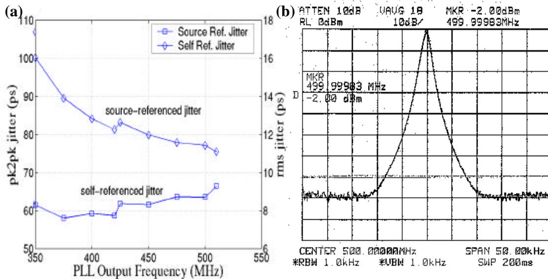
Figure 4.47: (a) Measured self-referenced and source-reference jitter of the x2 PLLFS at the low-end of frequency range of the PLLFS IC. (b) Spectrum of the 500 MHz output of the x2 PLLFS in this setting.
