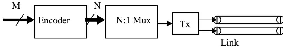
Figure 2.2: Block diagram of a typical transmitter.
