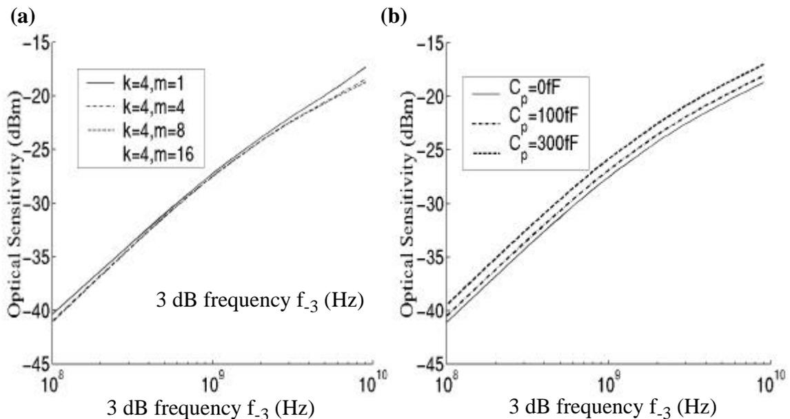
Figure 6.49: Plots of CGTIA sensitivity expression (Equation 6.99 and Equation 6.35). (a) covers the variation of  $m$  from 1,4,8,16 for  $k = 4$  and (b) shows the penalty accrued due to  $C_p = 0, 100, \text{ and } 300 \text{ fF}$  for  $k=4, m=8, C_d=500 \text{ fF}$ .
