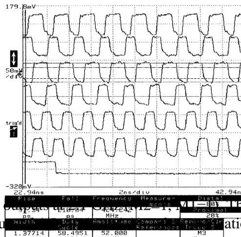
Figure 3.35: Prescaler outputs at 2.1 GHz. The display order is + and - outputs of 4/5, 4/5/6 and 4/6, after attenuation by 20 dB.
