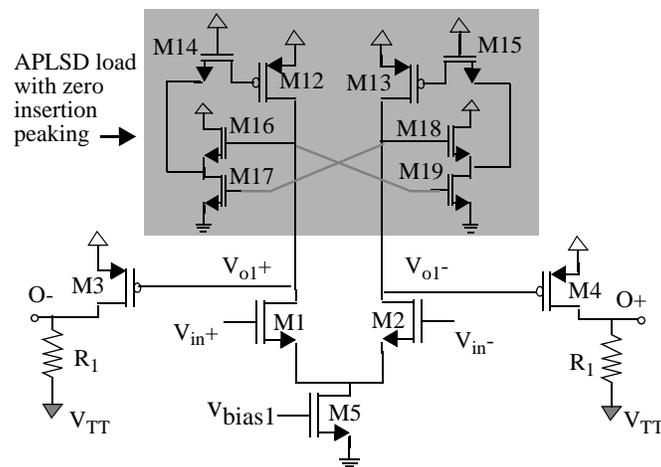
Figure 3.53: Schematic of differential LVDS Transmit (Tx) circuitry with optional source-termination resistor  $R_1$ .
