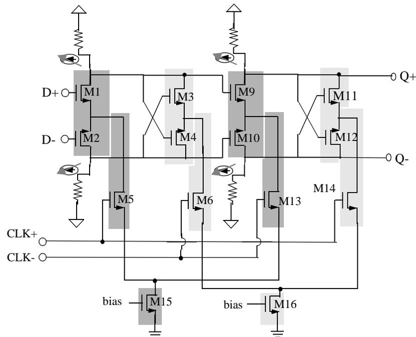
Figure 3.20: Schematic and symbol of differential master slave flip-flop
