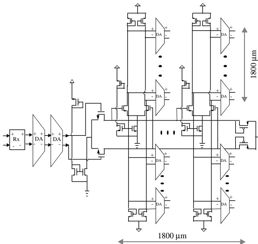
Figure 3.45: Schematic of a possible hierarchical extension of the clock distribution approach to larger systems.
