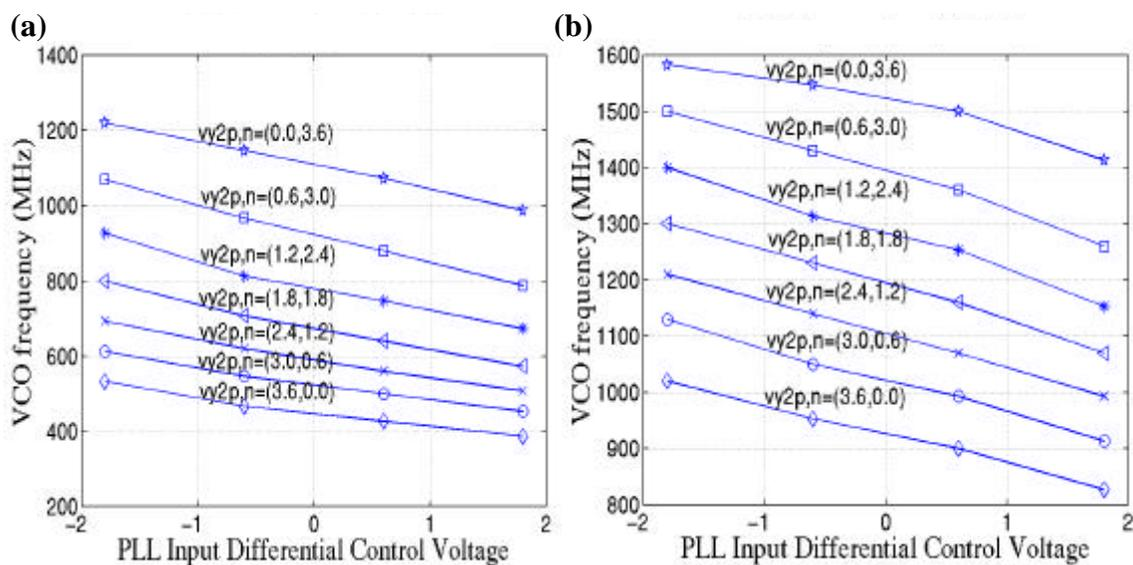
Figure 4.45: (a) Measured PLLFS VCO frequency variation with differential control voltage at different offset-control voltages at slope-control voltage  $V_B = 1.0$  V.
