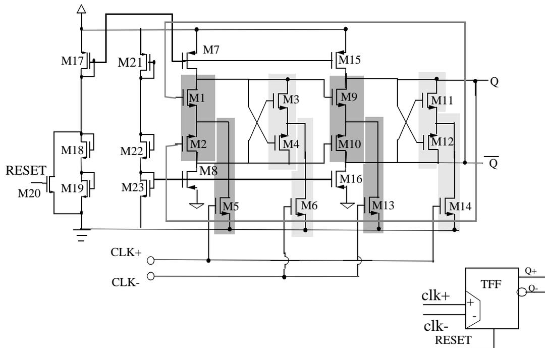
Figure 3.36: Schematic and symbol of high-speed Toggle Flip-Flop (TFF).
