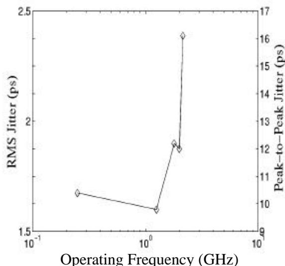
Figure 3.31: Self-referenced jitter (rms and peak-to-peak) dependence of 4/6 prescaler on operating frequency.
