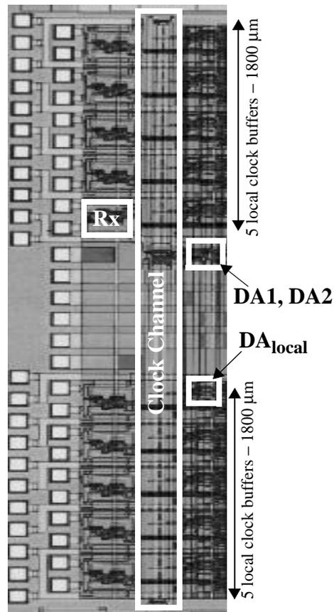
Figure 3.42: Die photograph of test IC in 0.8  $\mu\text{m}$  CMOS which implements the proposed clock distribution scheme.
