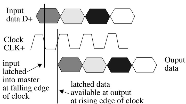
Figure 3.13: Waveforms describing behavior of differential flip-flop in Figure 3.12.
