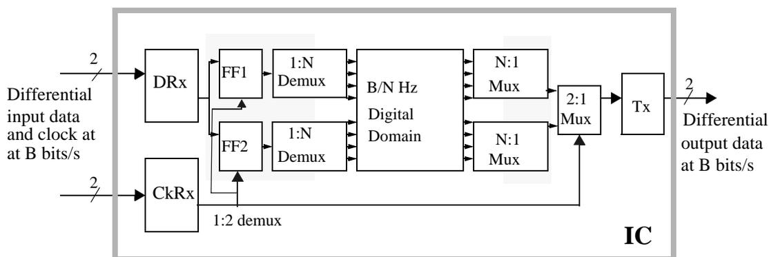
Figure 5.15: Block diagram of a half-speed link with 1:N/N;1 demux/mux circuits.
