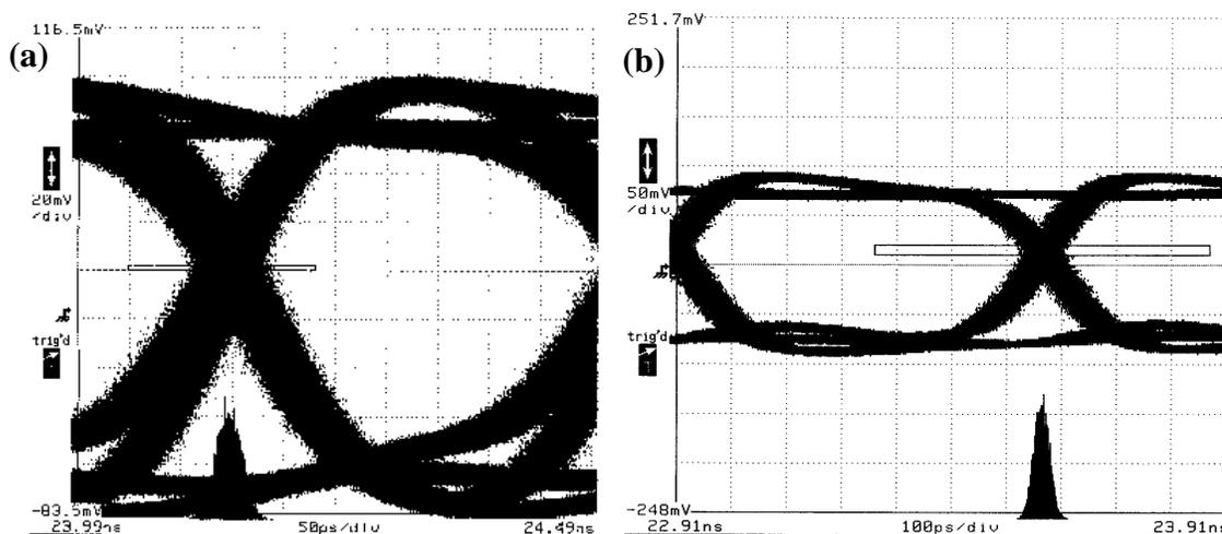
Figure 6.71: Measured output jitter of a representative OE channel at (a) 2.5 Gb/s for -16 dBm and (b) 1.5 Gb/s for -19 dBm  $2^{31} - 1$  NRZ PRBS input data patterns and clock signals. The jitter is measured to be (a) 12.47 ps rms (82 ps peak-to-peak) and (b) 14.35 ps rms and 94 ps peak-to-peak.
