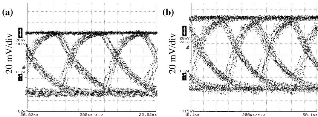
Figure 5.18: Eye-diagrams of 1:2/2:1 demux/mux BER circuit on T4 at (a) 1.5 Gb/s and (b) 1.8 Gb/s. The horizontal scale is 200 ps/div for both (a) and (b).
