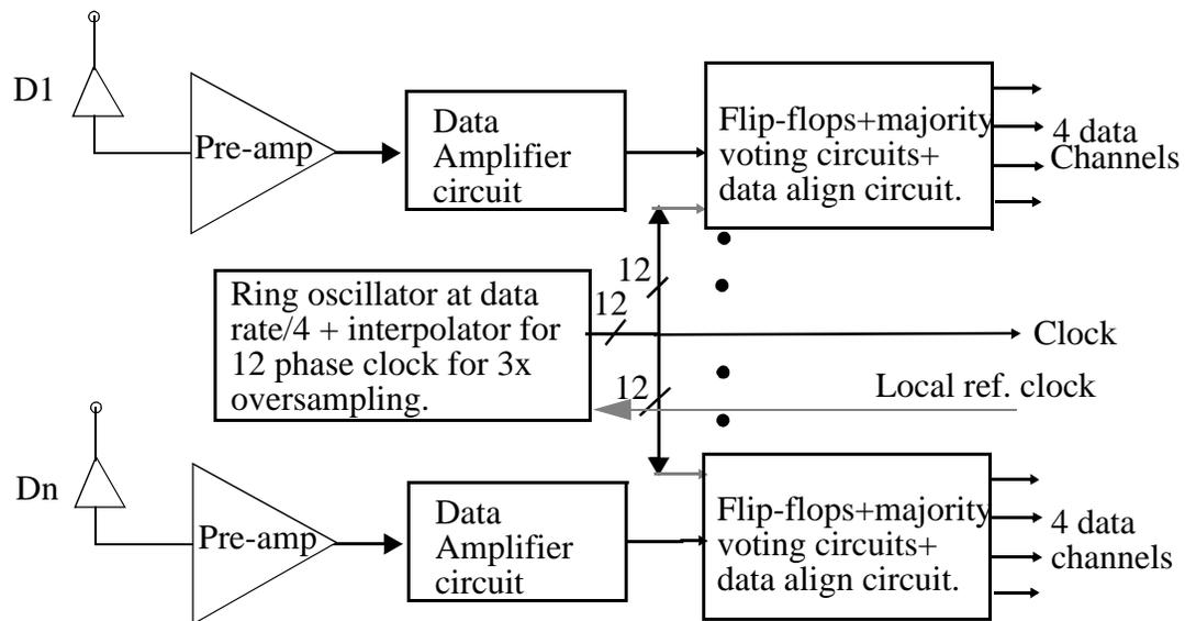
Figure 6.17: Half-speed OE receiver array schematic with oversampling receivers adapted from [10][42] for a 1:4 demultiplexer array.
