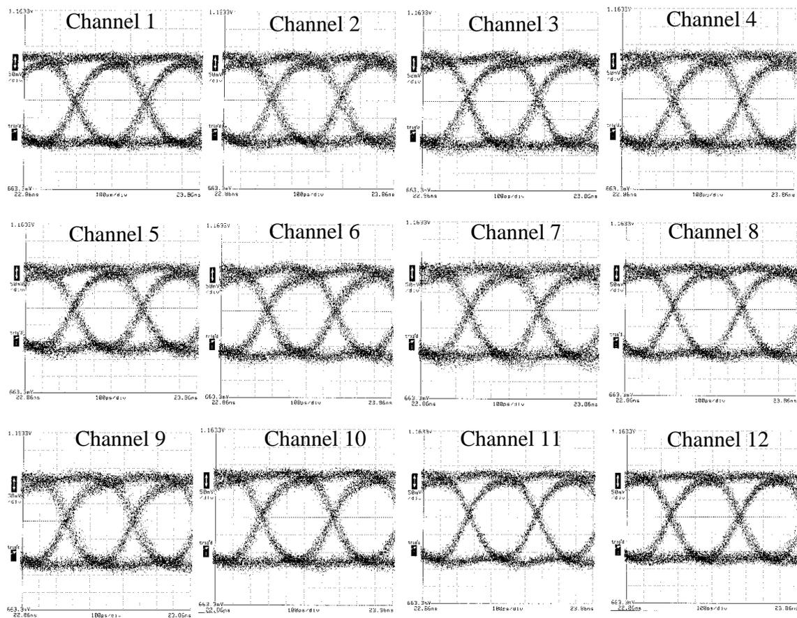
Figure 5.63: Source-referenced PONI Tx-Rx 2.5 Gb/s optical eye-diagrams measured (using the BERT trigger output as the oscilloscope trigger) at the positive high-speed optical outputs. The vertical scale is 100 mV/div and the horizontal scale is 100 ps/div for all eye-diagrams.
