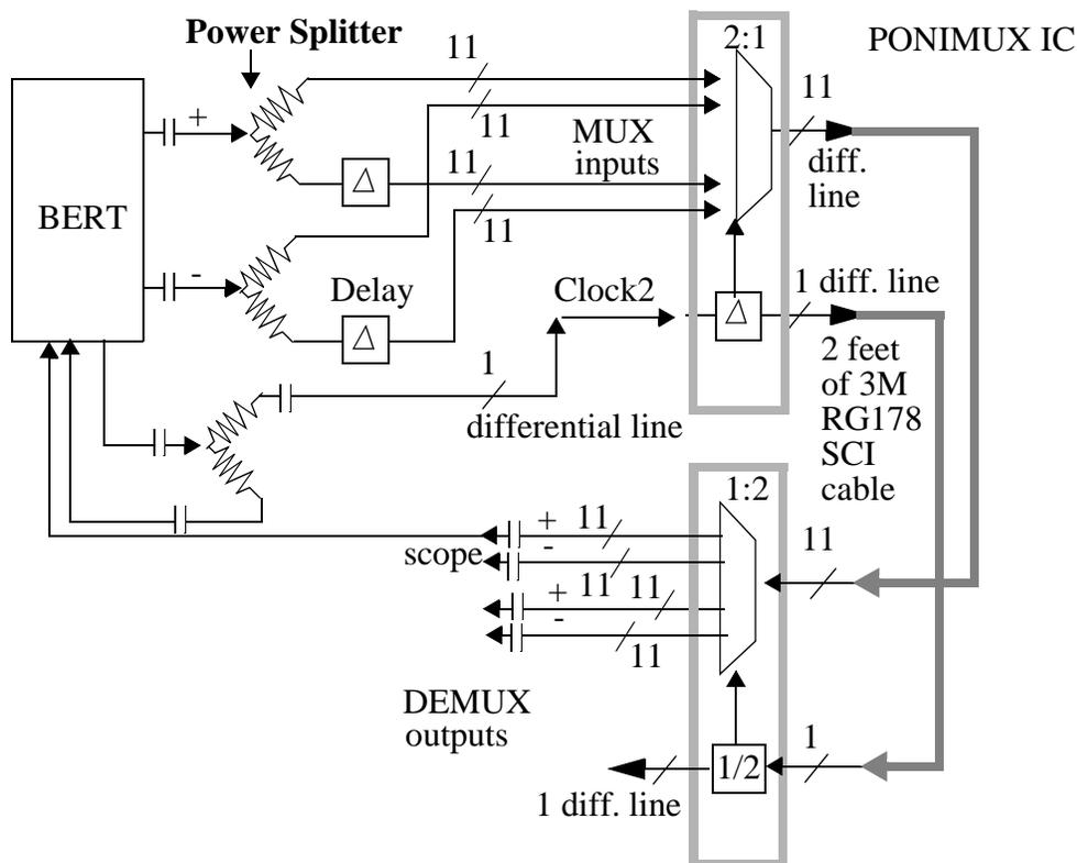
Figure 5.26: Schematic of the test setup for high-speed loopback and the generation of high-speed output eye-diagrams.
