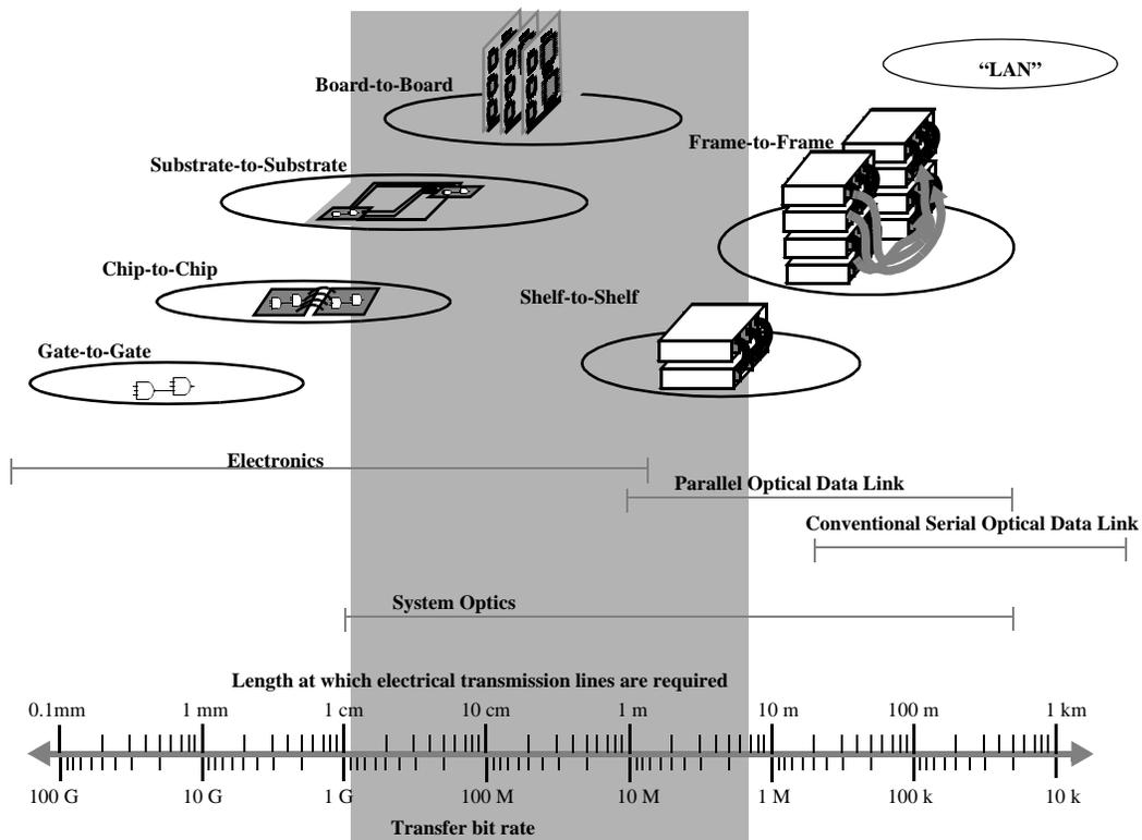
Figure 1.7: System-level insertion point of parallel optical links [13].
