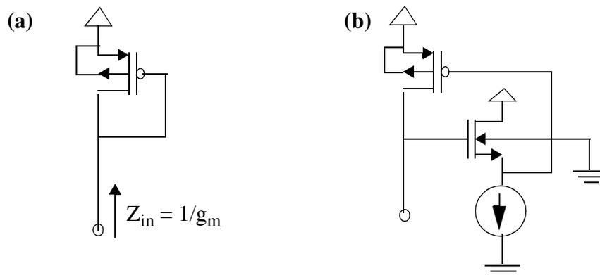
Figure 3.5: Schematic of possible diode-connected PMOS transistor load devices.
