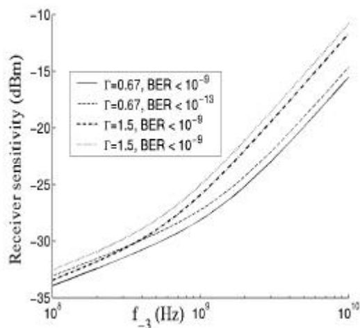
Figure 6.36: Receiver input sensitivity variation with input stage bandwidth for varying BER requirement and excess channel thermal-noise factor,  $\Gamma$ .
