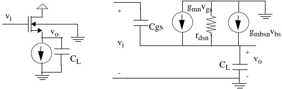
Figure 3.7: Small-signal model of source follower with current-sink bias.
