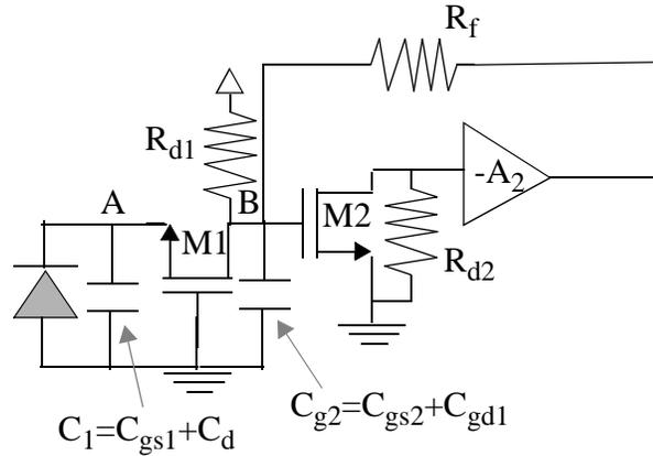
Figure 6.40: AC-diagram of CG OE pre-amplifier.
