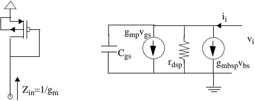
Figure 3.6: Small-signal model of diode-connected PMOS transistor load device.
