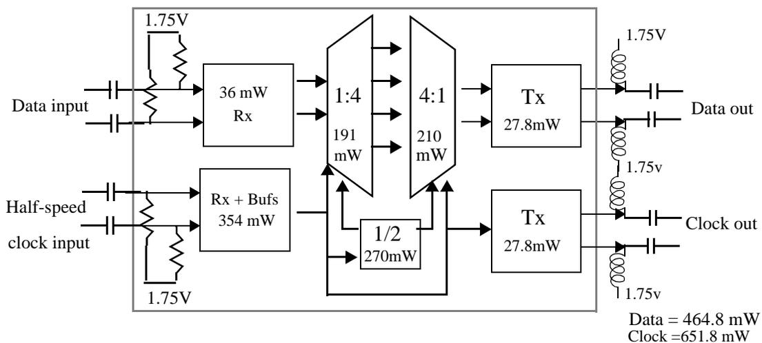
Figure 5.19: Schematic and test-setup of IC (T9) shown in Figure 5.20.
