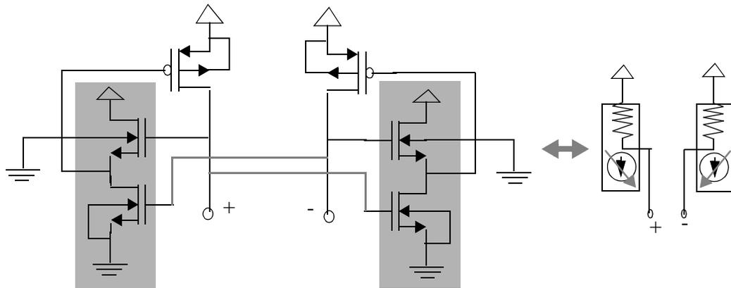
Figure 3.10: Schematic and symbol of Active Pull-down Level-Shift Diode-connected (APLSD) PMOS transistor loads in differential circuits.
