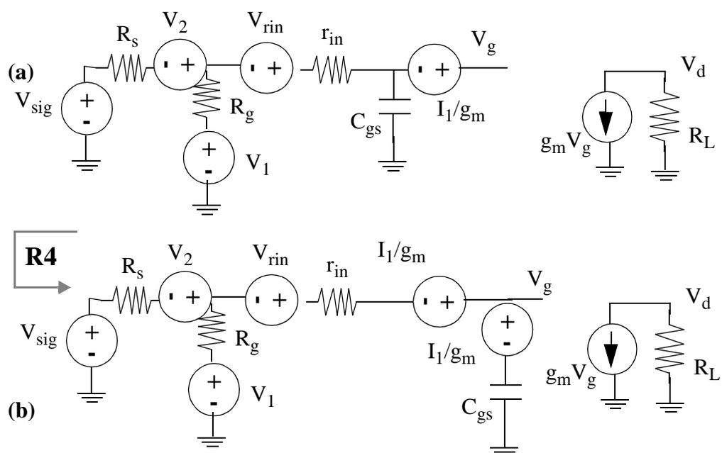
Figure 6.29: Transposition of  $I_1$  in Figure 6.28 to the input.
