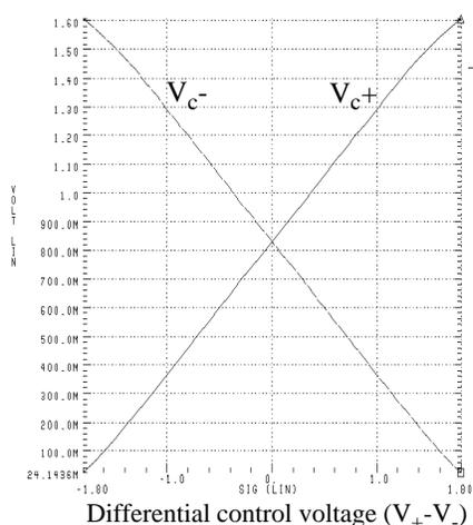
Figure 4.16: Gate-to-source voltage of transistors M8 and M10 in Figure 4.10 for revised LVIC.
