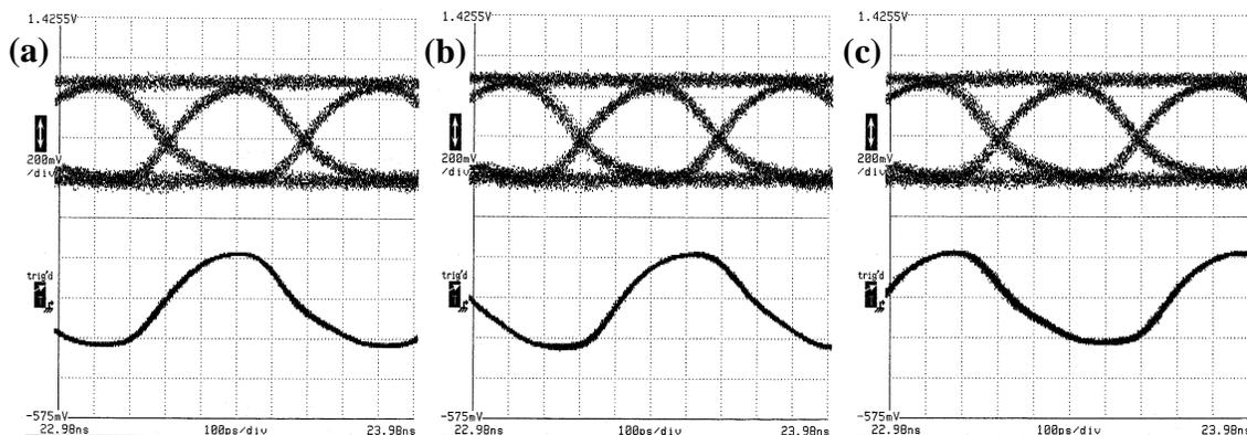
Figure 5.29: PCLK and PDOUT5 eye-diagrams at 2.5 Gb/s with (a) the clock output delay-chain at extreme left setting (least delay), (b) at nominal delay setting, and (c) at extreme right setting (maximum delay). Note that the PDOUT5 eye-diagram is at the same time position in (a), (b), and (c). The vertical scale is 200 mV/div and the horizontal scale is 100 ps/div for (a), (b) and (c).
