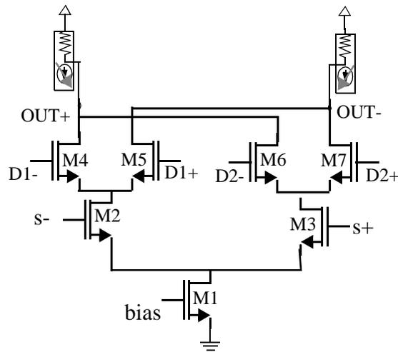
Figure 3.26: Schematic of differential 2:1 multiplexer
