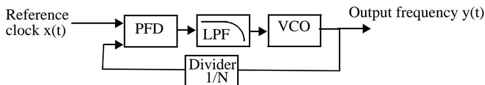
Figure 4.1: Block diagram of a generic PLLFS.
