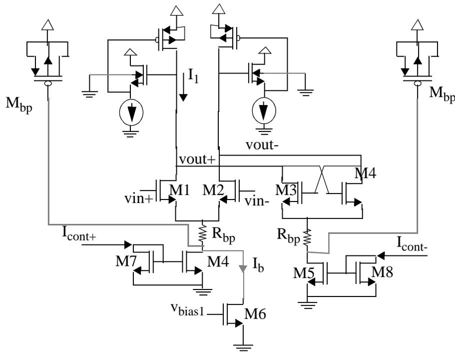
Figure 4.8: Differential delay cell with local positive feedback with power supply decoupling.
