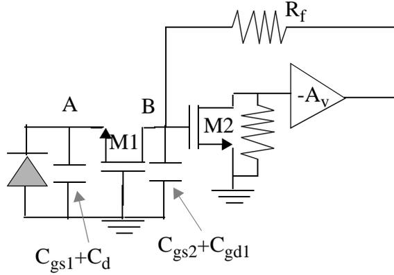
Figure 6.32: AC-schematic of CG OE pre-amplifier.
