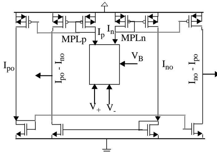
Figure 4.13: Differential linear voltage-to-current converter (LVIC).
