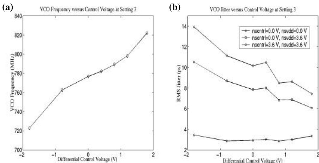
Figure 4.34: (a) Measured frequency and (b) self-referenced rms jitter histogram variation of T8 VCO at setting 3, for different levels of noise injection. The TLL pads are not terminated in measurements.
