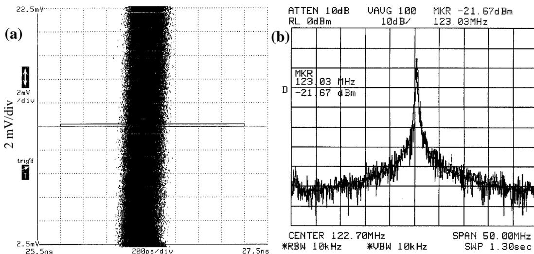
Figure 4.31: (a) Self-referenced jitter of 123 MHz VCO output with 70.73 ps rms (420 ps peak-to-peak). The horizontal scale is 200 ps/div. (b) Spectrum analyzer output of 123 MHz oscillation of T8 VCO. The noise source **ni1** is active for both (a) and (b).
