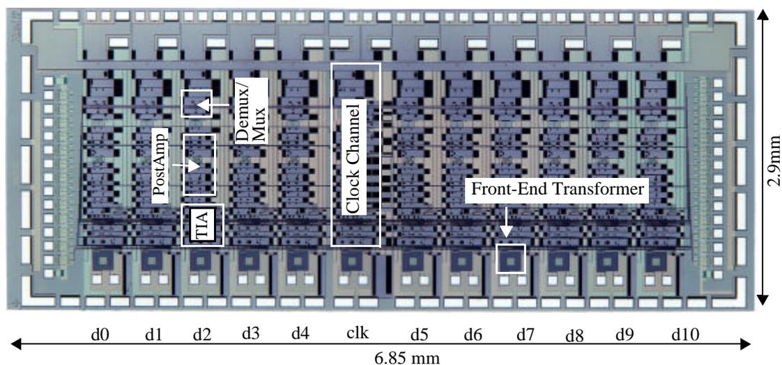
Figure 6.65: Micro-photograph of OE receiver array in 0.5  $\mu\text{m}$  CMOS technology. The submitted layout size is 6.40 mm x 2.7 mm and the IC die size is 6.85 mm x 2.9 mm.
