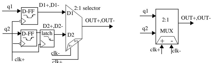
Figure 5.4: Schematic and symbol of 2:1 mux composed of dynamic flip-flops.
