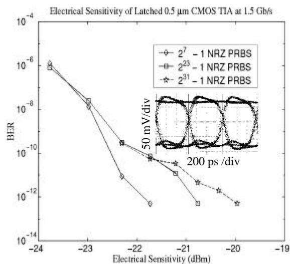
Figure 6.70: Measured sensitivity curve for a representative OE receiver array channel at 1.5 Gb/s for  $2^7 - 1$ ,  $2^{23} - 1$  and  $2^{31} - 1$  NRZ PRBS input data patterns. The insert shows the electrical output eye diagram at a BER  $< 10^{-12}$  for -19 dBm  $2^{31} - 1$  NRZ PRBS input data patterns and -19 dBm clock inputs.
