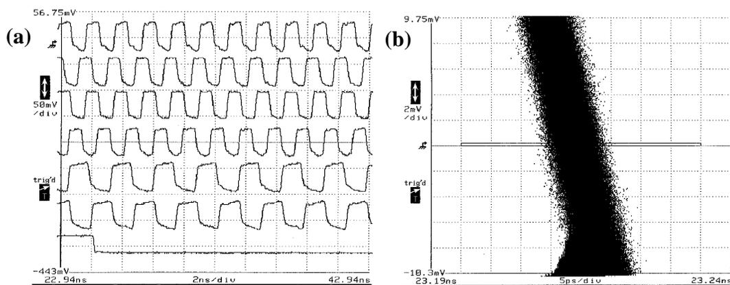
Figure 3.32: (a) Prescaler outputs at 2.17 GHz (M2=1,M1=0). 4/5, 4/5/6 prescalers in divide-by-4 mode and 4/6 mode in divide-by-6 mode. (b) shows the jitter histogram of 4/5/6 prescaler output with respect to the trigger pattern.
