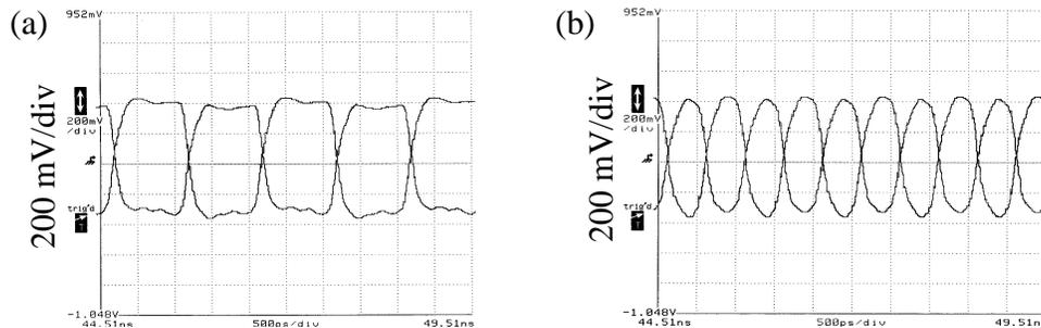
Figure 5.17: External divider output at (a) 0.5 GHz and (b) 1.0 GHz. The horizontal scale is 500 ps/div for both (a) and (b).
