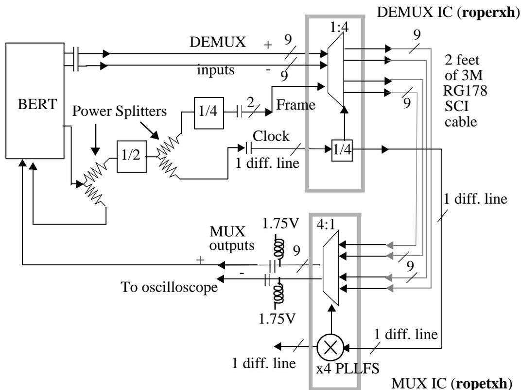
Figure 5.53: Schematic of the slow-speed 4:1/1:4 Mux/Demux loopback test setup. Clock is a differential signal, though drawn with only one wire.
