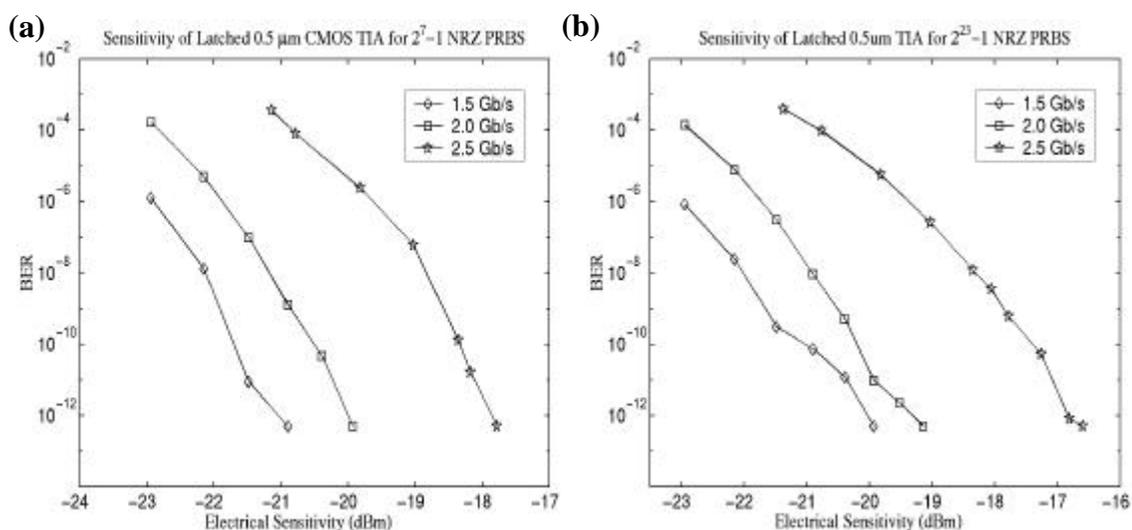
Figure 6.67: Measured sensitivity curves for 1.5 Gb/s, 2.0 Gb/s and 2.5 Gb/s for (a)  $2^7 - 1$  and (b)  $2^{23} - 1$  NRZ PRBS input data patterns.
