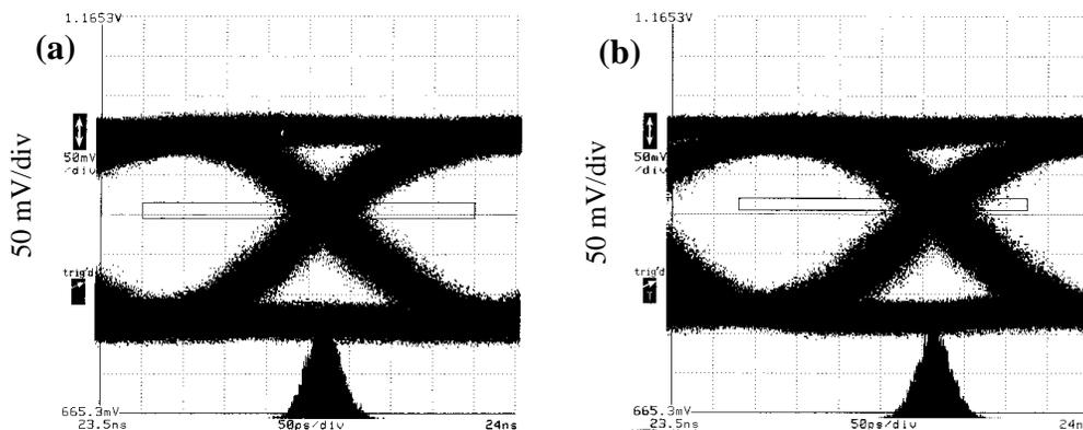
Figure 5.67: Source-referenced jitter statistics of the optical Rx module corresponding to PDOUT3+ and PDOUT7+. The vertical scale is 50 mV/div and the horizontal scale is 100 ps/div for both (a) and (b).
