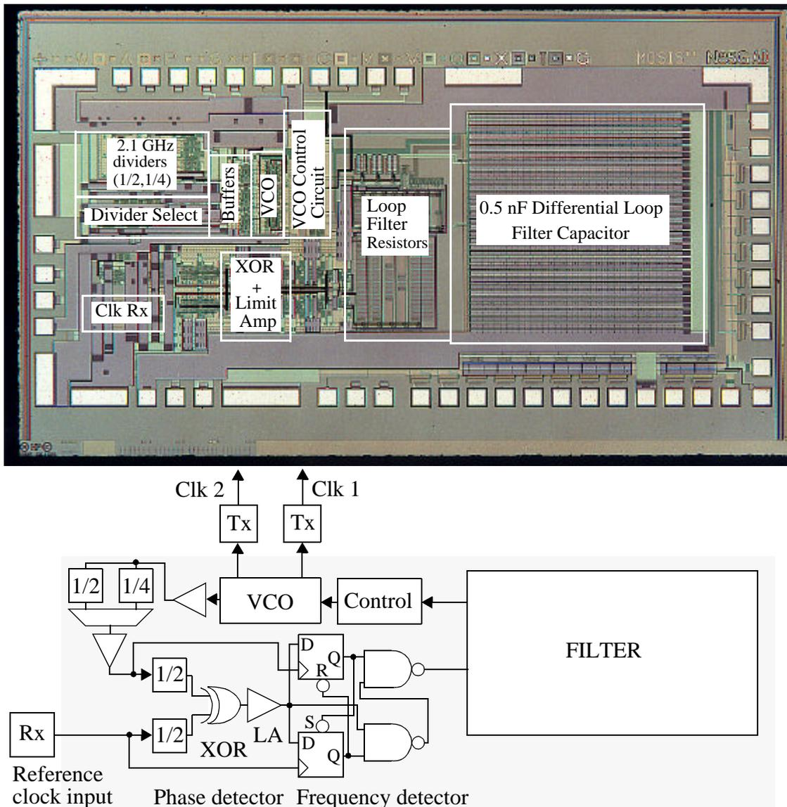
Figure 4.44: (a) Photograph of the PLLFS IC implemented in  $0.5\ \mu\text{m}$  CMOS. The IC size is  $3.29 \times 1.63\ \text{mm}^2$ , which includes a  $1.7 \times 1.2\ \text{mm}^2$  integrated differential-loop capacitor and programmable filter resistors. The IC consumes  $1.2\ \text{W}$  from a  $3.6\ \text{V}$  power supply. (b) Block diagram of the PLLFS.
