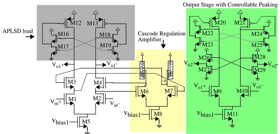
Figure 3.46: Schematic of controlled peaking amplifier implemented with regulated cascode amplifier input stage followed by output stage with controlled zero insertion by the control signal sncntrl.
