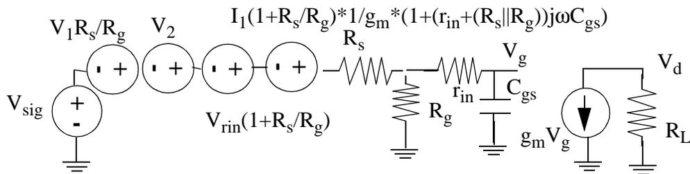
Figure 6.31: Final small-signal model of the CS amplifier showing all noise sources referred to the input.
