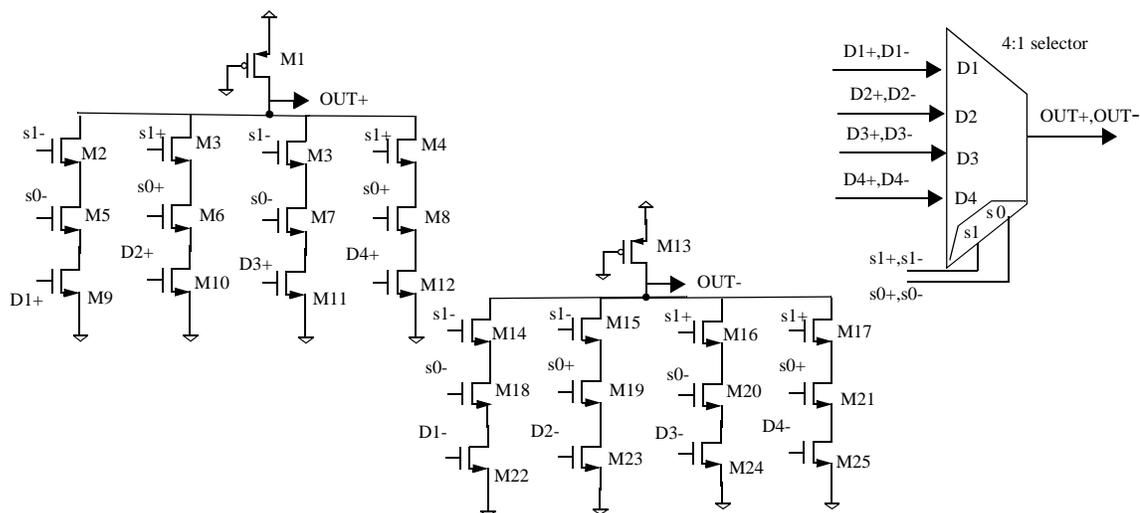
Figure 5.8: Schematic and Symbol of 4:1 selector for wired-OR 4:1 mux design.
