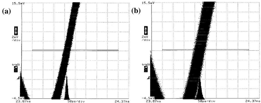
Figure 4.35: Self-referenced jitter histogram of the T8 VCO at 1.53 GHz with (a) **ni1** and (b) both noise oscillators and the TTL pad drivers injecting noise into the VCO. The measured jitter is 4.73 ps rms (36 ps peak-to-peak) and 8.1 ps rms (59 ps peak-to-peak) in plots (a) and (b) respectively. The horizontal scale is 50 ps/div and the vertical scale is 2 mV/div for both (a) and (b).
