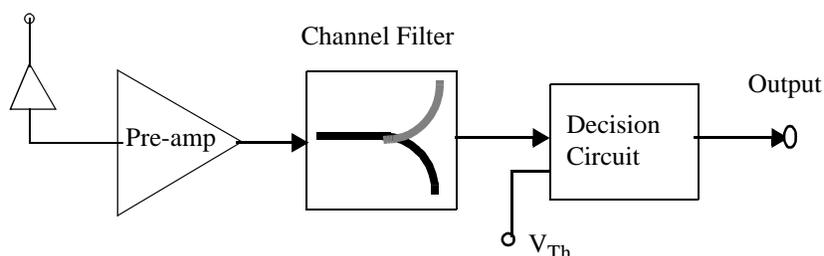
Figure 6.11: Block diagram of an asynchronous OE receiver
