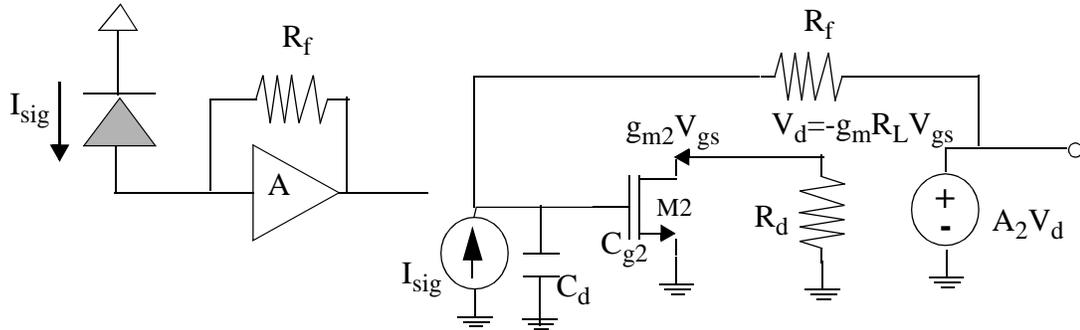
Figure 6.39: Elementary TIA and its small-signal model.
