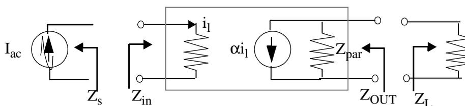
Figure 6.10: Linear two-port representation of interconnect.
