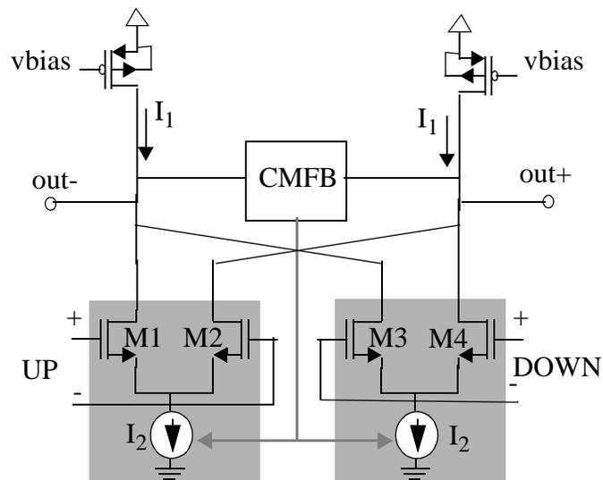
Figure 4.38: Differential charge pump schematic [135]
