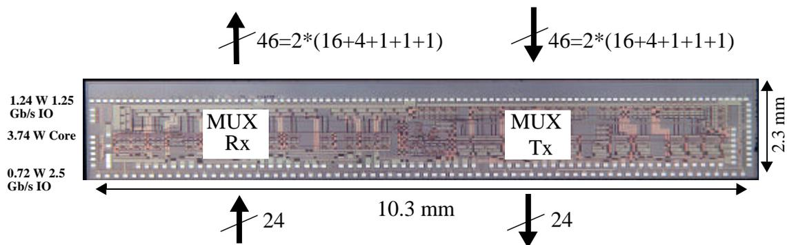
Figure 5.24: Microphotograph of the 0.5  $\mu\text{m}$  CMOS PONIMUX IC. The submitted IC layout was 10.1 mm x 1.8 mm. The die size of the IC is 10.3 mm x 2.3 mm.
