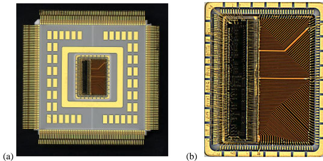
Figure 5.25: (a) Photograph of the PONIMUX IC in the PONI MUX QFP cavity. The QFP is 1.35 inches on a side and has 244 leads on a 20 mil pitch. (b) Blow-up of cavity detail showing IC and the insert which carries the signals from the slow-speed bonding pads on the IC to the PONI MUX QFP cavity signal shelf.
