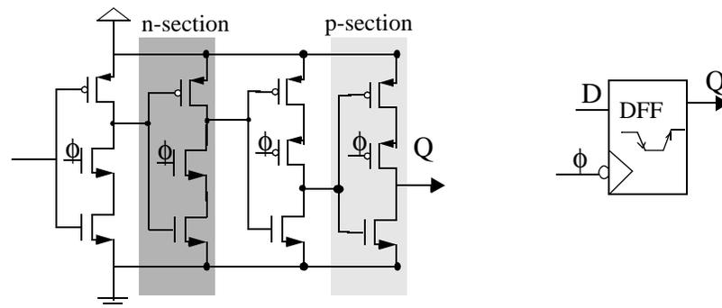
Figure 3.37: Schematic and symbol of an nnpp DFF.
