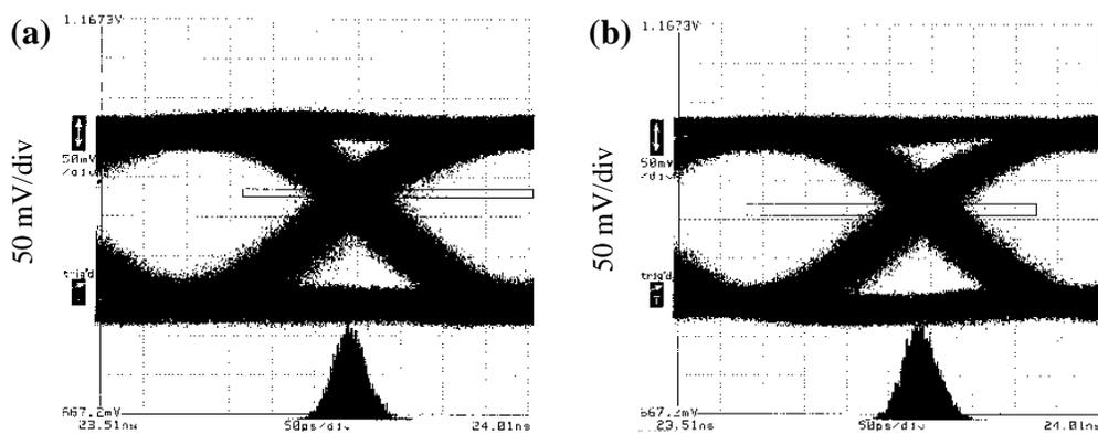
Figure 5.68: Self-referenced jitter statistics of the optical Rx module outputs corresponding to PDOUT1+ and PDOUT7+. The horizontal scale is 50 ps/div and the vertical scale is 50 mV/div for both (a) and (b).
