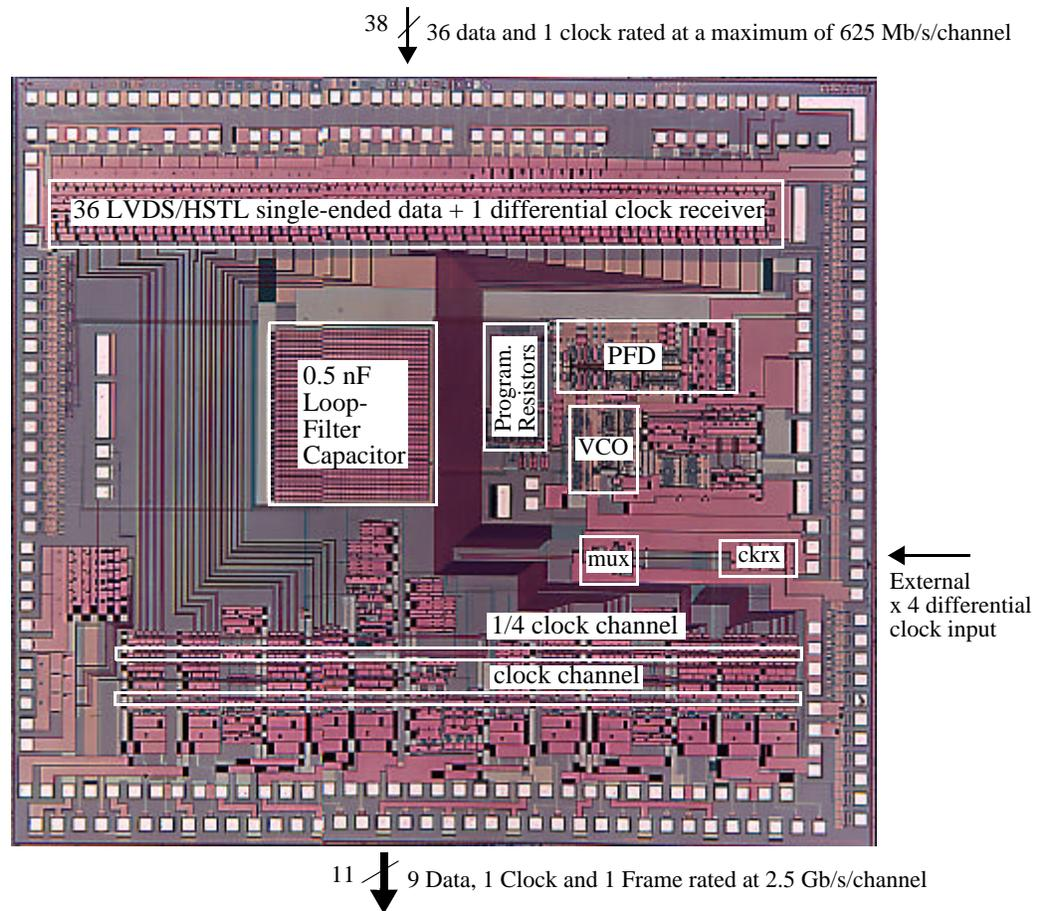
Figure 5.49: Microphotograph of the **ropetxh** IC, which incorporates an integrated x4 PLLFS circuit.
