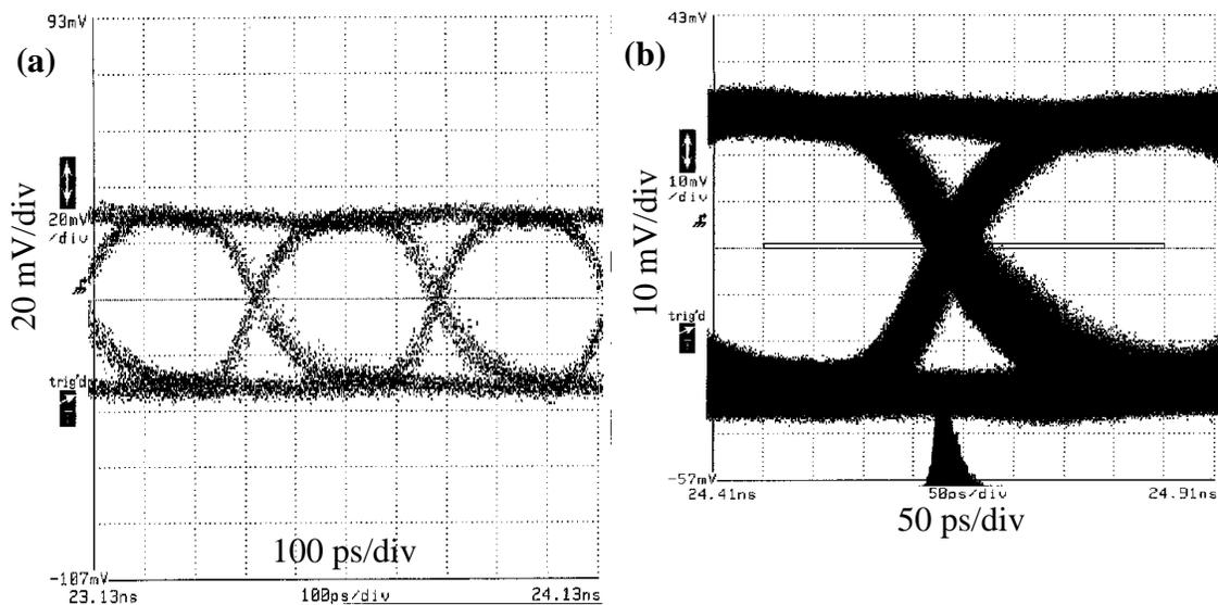
Figure 5.21: (a) Error-free 2.8 Gb/s eye-diagram and (b) BERT trigger referenced jitter histogram.
