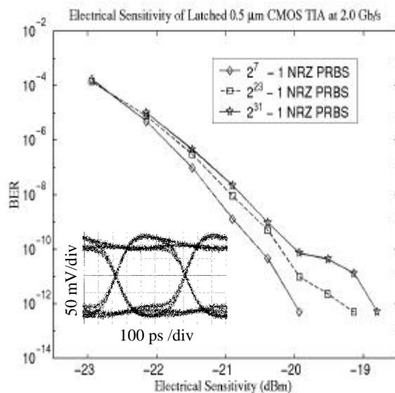
Figure 6.69: Measured sensitivity curve for a representative OE receiver array channel at 2.0 Gb/s for  $2^7 - 1$ ,  $2^{23} - 1$  and  $2^{31} - 1$  NRZ PRBS input data patterns. The insert shows the electrical output eye diagram at a BER  $< 10^{-12}$  for -19 dBm  $2^{31} - 1$  NRZ PRBS input data patterns and -19 dBm clock inputs.
