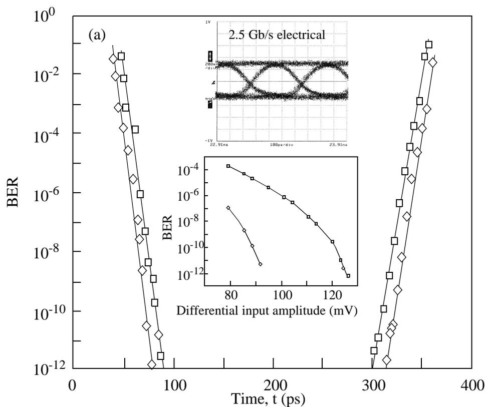
Figure 5.41: (a) Measured high-speed side (2.5 Gb/s, 400 ps bit-period) output phase-margin with electrical loopback on the slow-speed side (1.25 Gb/s) and 126.5 mV differential input data amplitude.
