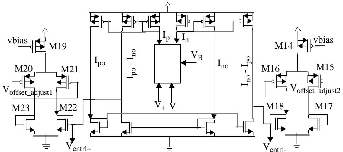
Figure 4.19: Differential linear voltage-to-current converter with offset adjust circuitry.  $V_B$  is the slope control.
