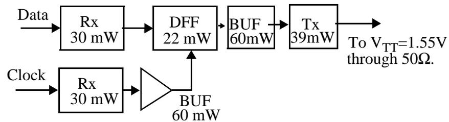
Figure 3.23: Schematic of layout to test operation of D flip-flop in Figure 3.20.
