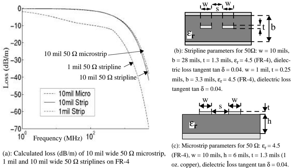
Figure 1.5: Calculated loss of microstrip and stripline with frequency [191].
