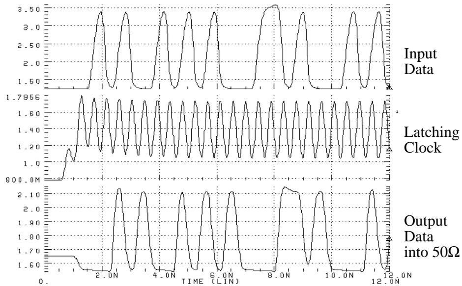
Figure 3.25: D flip-flop (Figure 3.12) operation at 2.3 Gb/s at 160 ps clock-to-data setup time.
