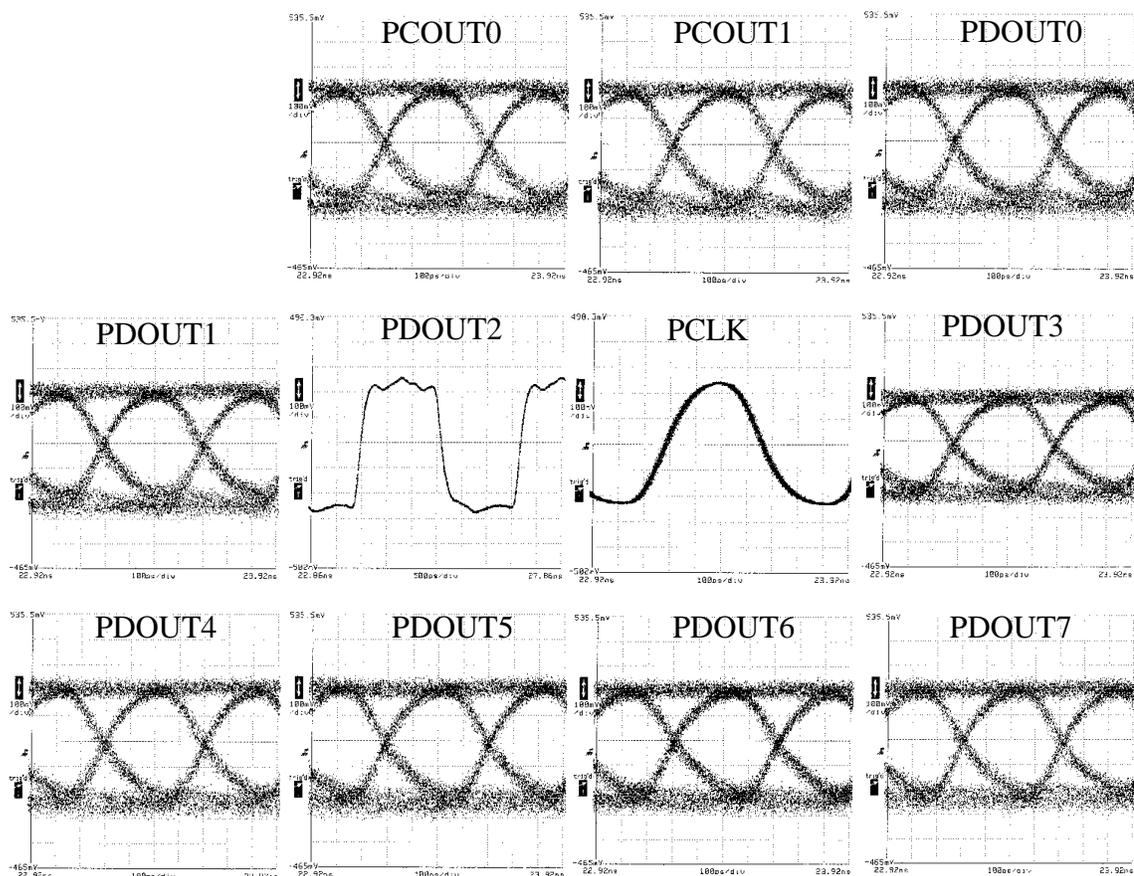
Figure 5.54: 2.5 Gb/s source-referenced eye-diagrams obtained at the positive high-speed mux output. The vertical scale is 100 mV/div and the horizontal scale is 100 ps/div for all plots.
