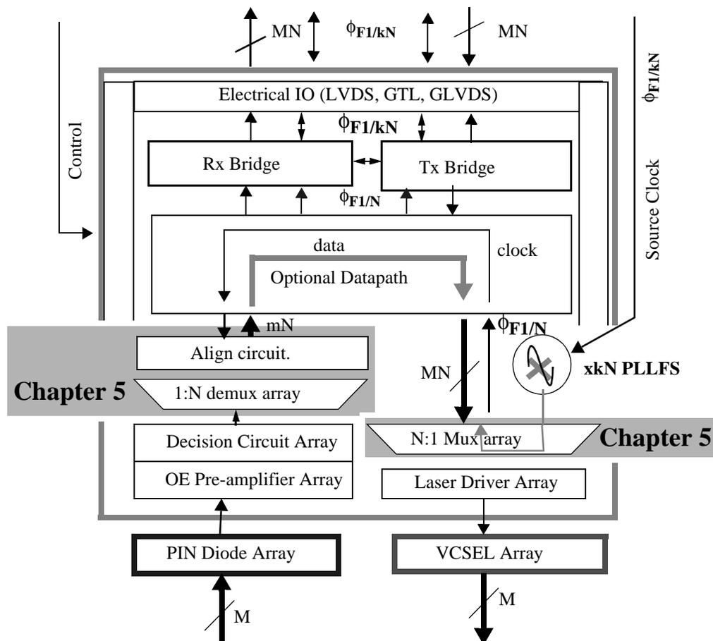
Figure 5.1: Correspondence of the discussion in this chapter to the OESIC block diagram in Figure 1.10.
