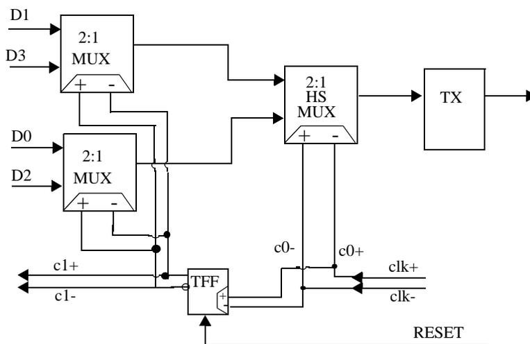
Figure 5.13: Schematic of half-speed 4:1 multiplexer composed of 2:1 muxes.
