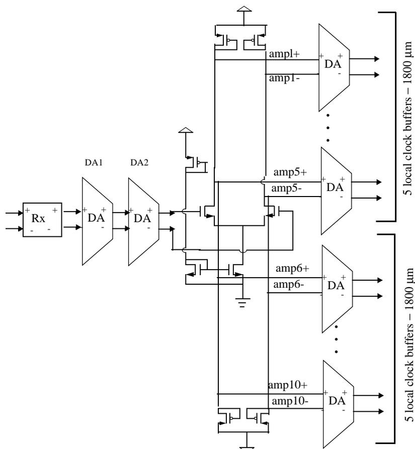
Figure 3.41: Schematic of clock distribution scheme from the input pads.
