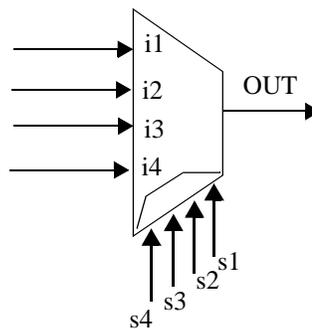
Figure 5.48: Symbol of 4:1 multiplexer used to shuffle the demultiplexed data outputs **i1**, **i2**, **i3** and **i4** of each high-speed channel.
