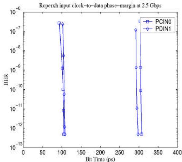
Figure 5.57: Variation of the **roperxh** IC high-speed input clock-to-data phase-margin for the outermost (squares) and the innermost (diamonds) input channels measured in electrical loopback on the slow-speed side.
