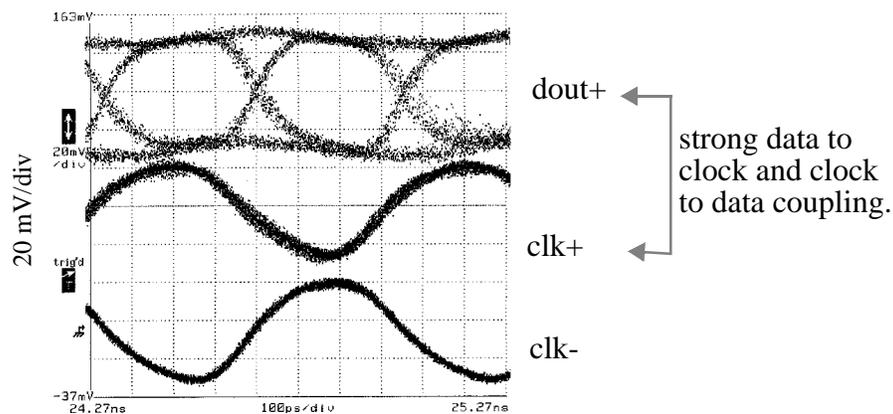
Figure 5.22: Bondwire coupling induced eye degradation. The horizontal scale is 100 ps/div and the vertical scale is 20 mV/div.
