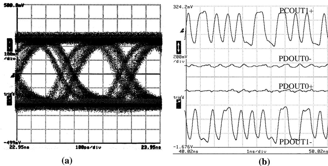
Figure 5.28: (a) Composite eye-diagram of 11 high-speed outputs at 2.5 Gb/s (The vertical scale is 100 mV/div and the horizontal scale is 100 ps), and (b) The noise induced on high-speed output lines from adjacent output lines. The vertical scale is 200 mV/div and the horizontal scale is 1 ns/div.
