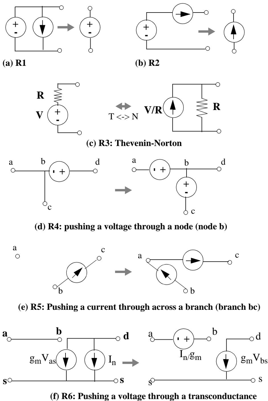
Figure 6.23: Rules R1 through R6 for the transposition of sources method of determining input-referred noise-current PSD of a linear two-port network.
