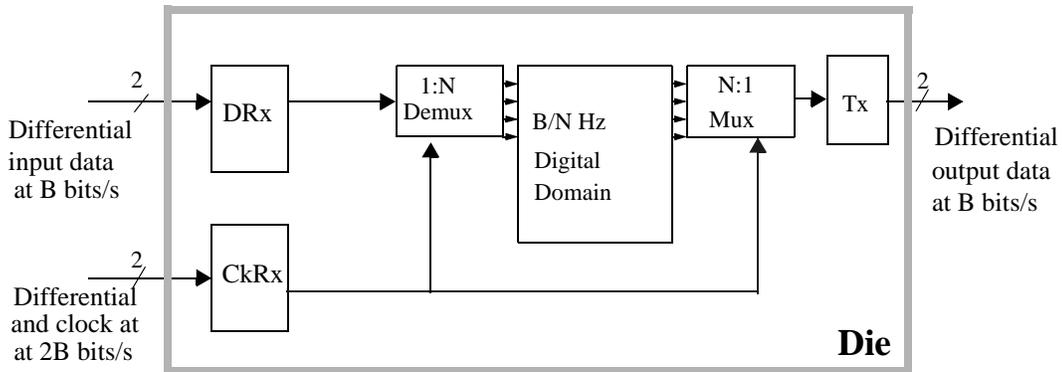
Figure 5.11: Block diagram of a full-speed link with 1:N/N:1 demux/mux circuits.
