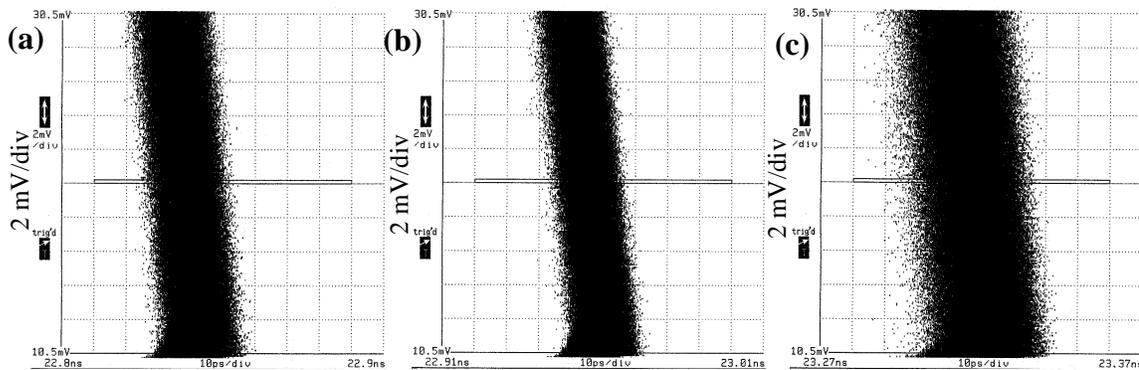
Figure 5.30: Falling-edge jitter on PCLK with PDOUT5 data at 2.5 Gb/s. (a) With clock output delay chain at extreme left setting (least delay), (b) at nominal setting, and (c) at extreme right setting (maximum delay). The vertical scale is 2 mV/div and the horizontal scale is 10 ps/div for (a), (b) and (c).
