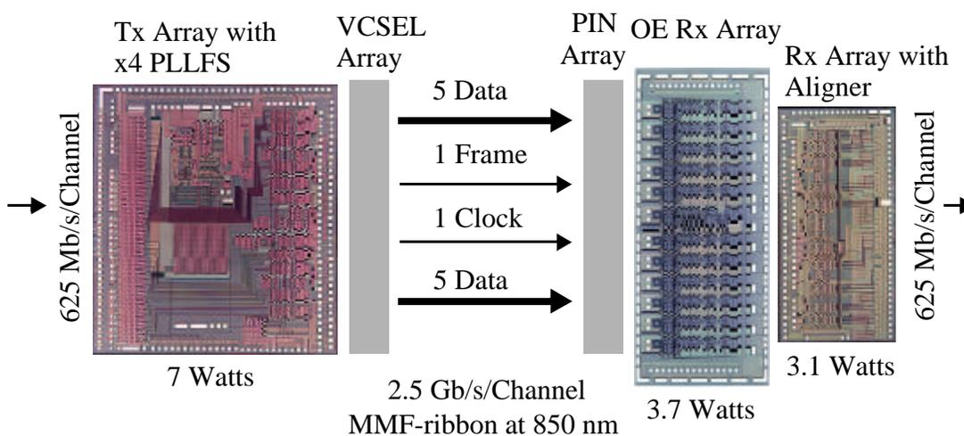
Figure 7.1: Proven design point of 25 Gb/s in 0.5  $\mu\text{m}$  CMOS process technology over 12-wide MMF-ribbon with 10 channels of data.
