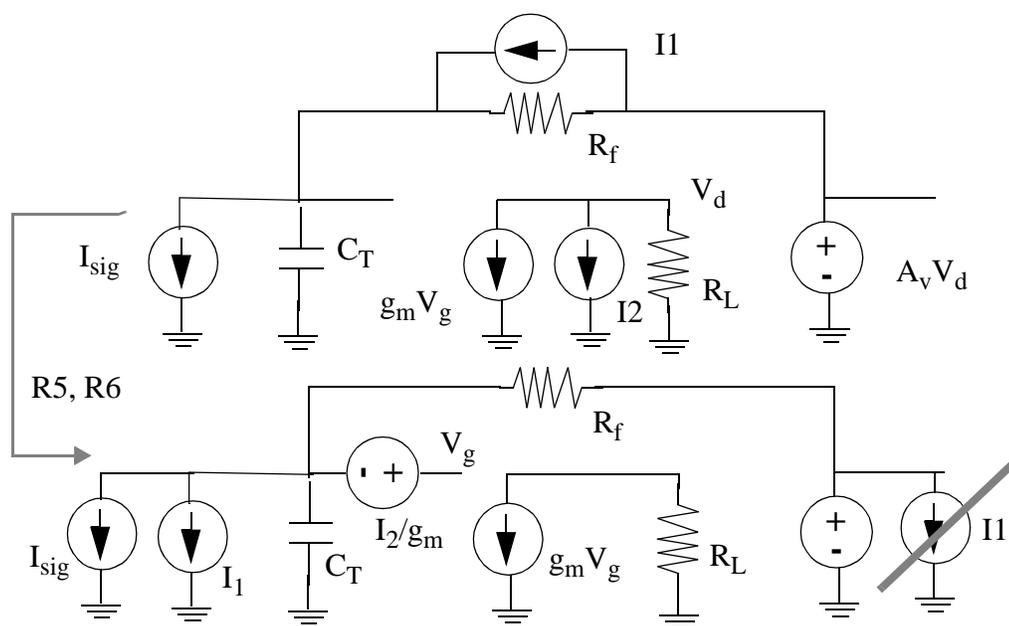
Figure 6.26: Transformation of small-signal model by transposition of noise sources **I1** and **I2** from the output to the input. The transposed noise-current source **I1** in parallel with a voltage source is
