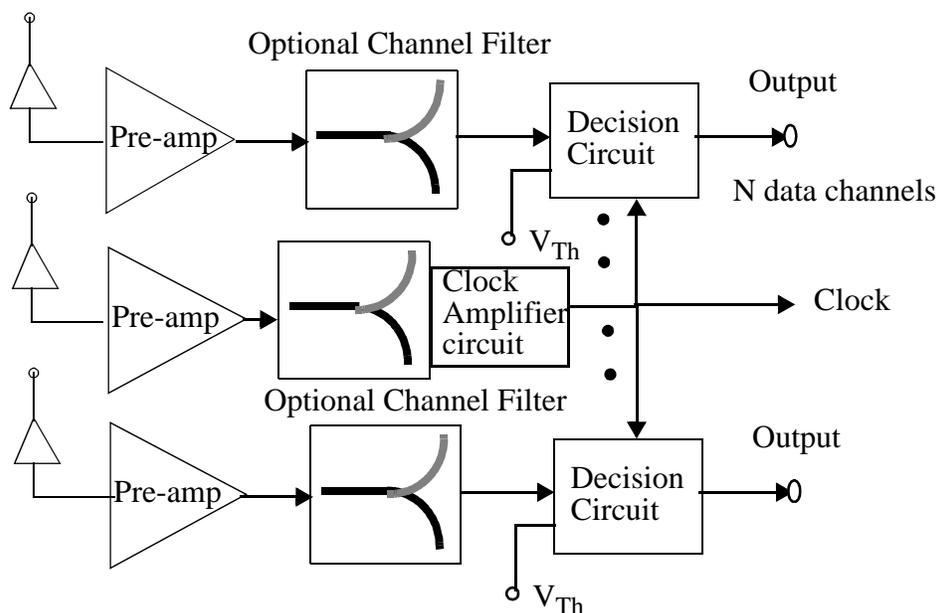
Figure 6.13: Extension of synchronous and asynchronous receiver circuits to parallel synchronous OE data link.
