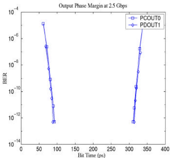
Figure 5.60: **ropetxh** high-speed output phase-margin for the innermost (PDOUT1, diamonds) and outermost (PCOUT0, squares) channels measured in electrical loopback on the slow-speed side.
