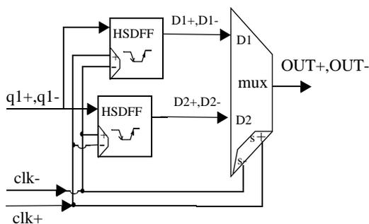
Figure 6.63: Schematic of differential retiming circuit.
