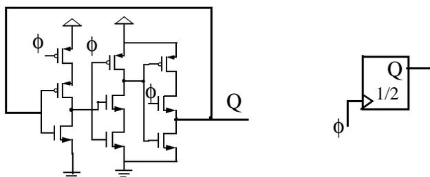
Figure 4.25: Schematic and symbol of toggle flip-flop used to divide the output of the single-ended oscillator.
