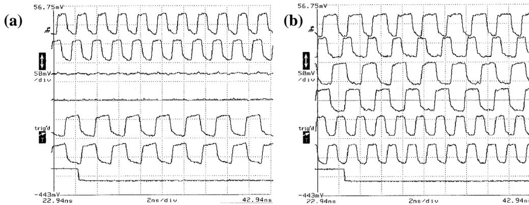
Figure 3.34: Prescaler outputs at 2.16 GHz for (a) (M2=0, M1=0) and at 2.14 GHz for (b) (M2=0, M1=1). The display order is + and - outputs of 4/5, 4/5/6 and 4/6, after attenuation by 20 dB.
