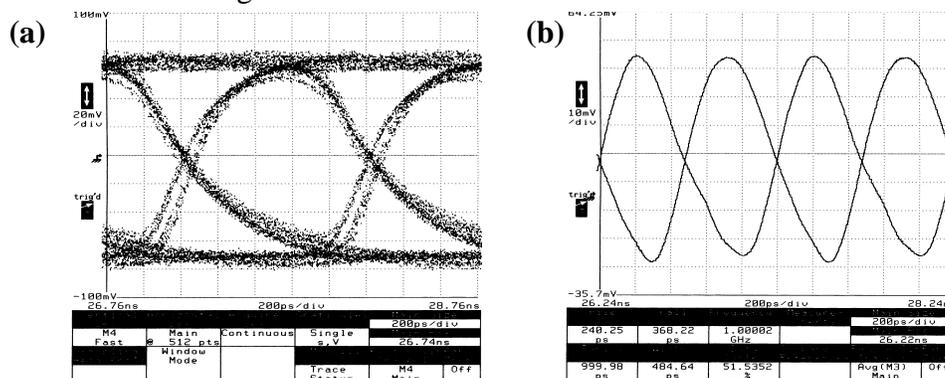
Figure 3.44: Measured performance of receive-transmit pair with 1 Gb/s data stream and 1 GHz clock.
