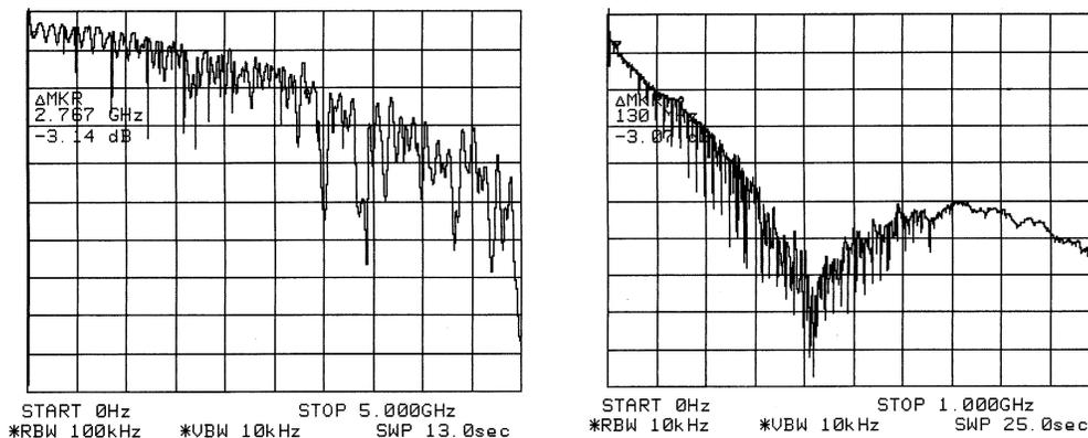
(a) Insertion-loss measurement of 1m of 22 AWG Belden 50  $\Omega$  cable. (b) Insertion-loss measurement of 30 m of 22 AWG Belden 50  $\Omega$  cable
