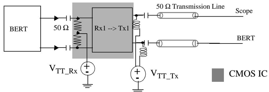
Figure 3.54: Schematic of setup one (S-1) interface connection.
