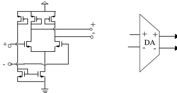
Figure 3.39: Schematic and symbol of a generic Differential Amplifier (DA).
