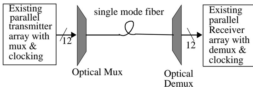
Figure 7.2: Block diagram of 12 channel 100 Gbit/s WDM link leveraging advances in parallel OE data links.
