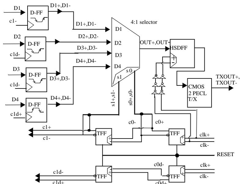
Figure 5.7: Schematic of Pseudo-NMOS style 4:1 multiplexer.
