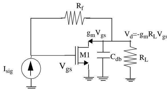
Figure 6.45: AC-equivalent circuit of elementary TIA.
