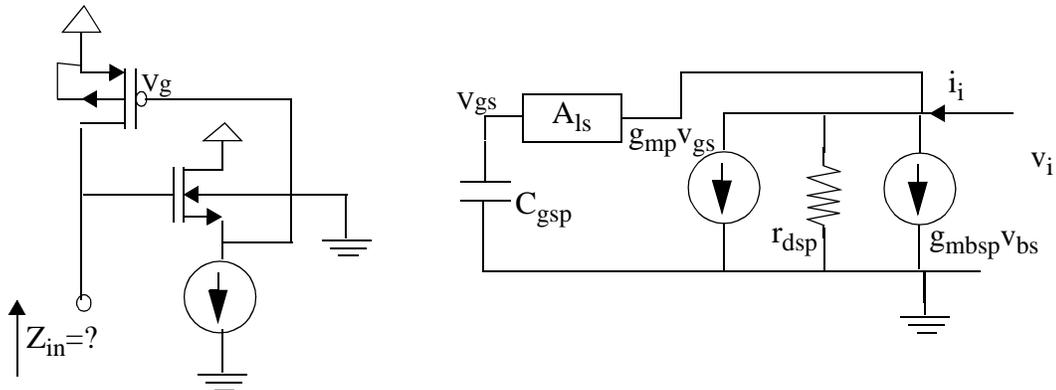
Figure 3.9: Schematic of level-shifted diode-connected PMOS transistor load and its small-signal model.
