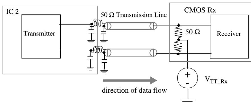
Figure 3.52: Schematic of the interface connection of the 2.5 Gb/s CMOS Rx circuit. IC2 can be Bipolar or future CMOS IC.
