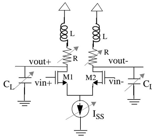
Figure 4.5: Schematic of a general differential gain-cell with delay-adjusting control knobs indicated by shaded arrows.
