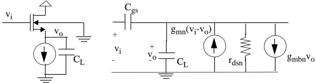
Figure 3.8: Redrawn small-signal model of Figure 3.7.
