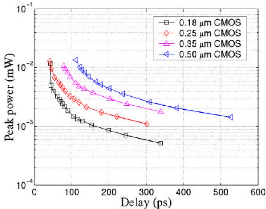
Figure 1.12: Power-delay curve of an inverter driving 100 fF of capacitive load in representative 0.5  $\mu\text{m}$  (rotated triangles), 0.35  $\mu\text{m}$  (triangles), 0.25  $\mu\text{m}$  (diamonds), and 0.18  $\mu\text{m}$  (squares) CMOS process technologies.
