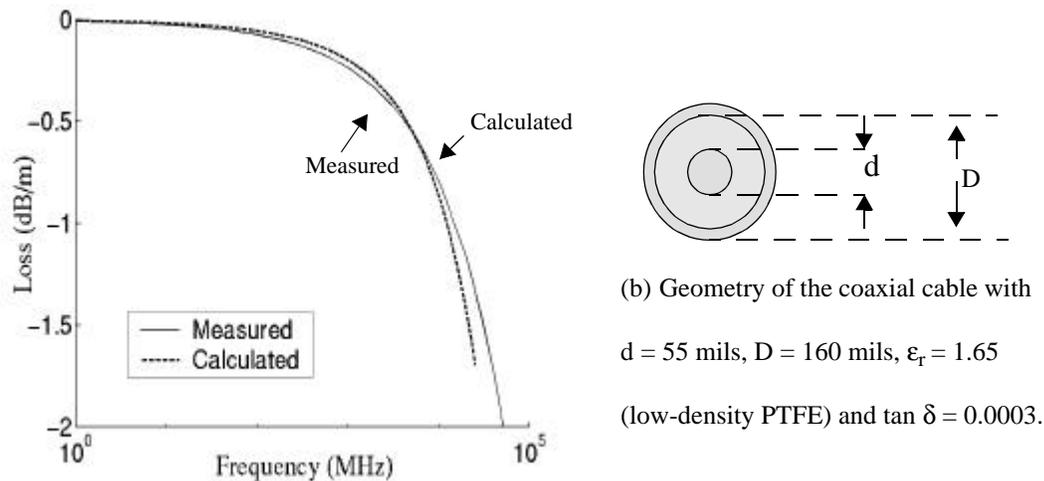
(a) Loss (dB/m) vs. Frequency for Coax (Sucoflex SF104)
