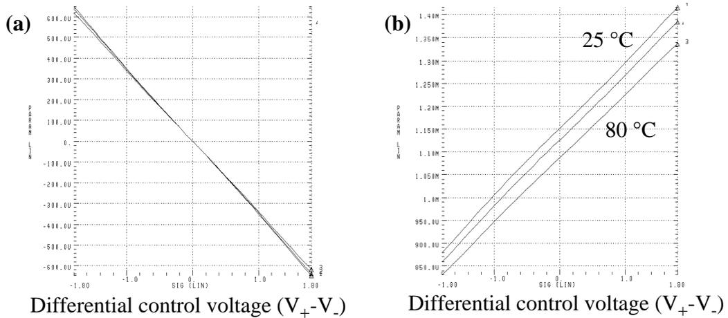
Figure 4.18: (a)  $I_p - I_n$  and (b)  $I_{po} - I_{no}$  for revised LVIC for temperature of 25 °C, 45 °C, and 80 °C.
