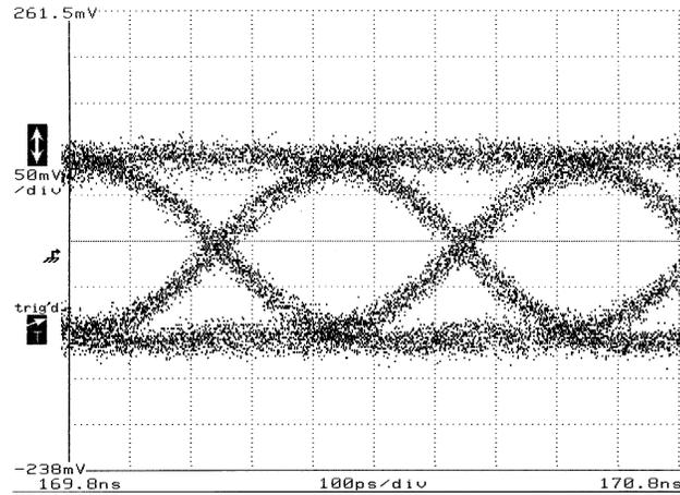
Figure 6.4: 2.5 Gb/s  $2^{31} - 1$  NRZ PRBS eye-diagram for LD L1 driven by BERT.
