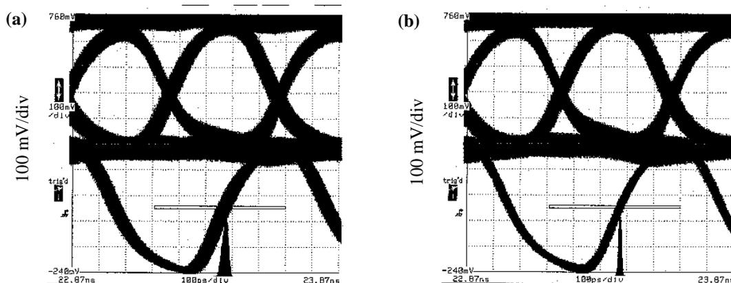
Figure 5.32: Clock jitter when (a) PDOUT7 and (b) PDOUT5 are active. The horizontal scale is 100 ps/div and the vertical scale is 100 mV/div for both (a) and (b).
