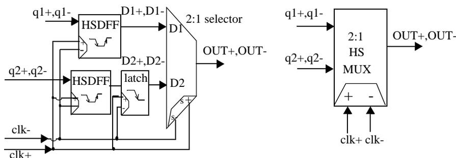
Figure 5.5: Schematic and symbol of high-speed 2:1 mux composed of HSDFFs (Figure 3.12).
