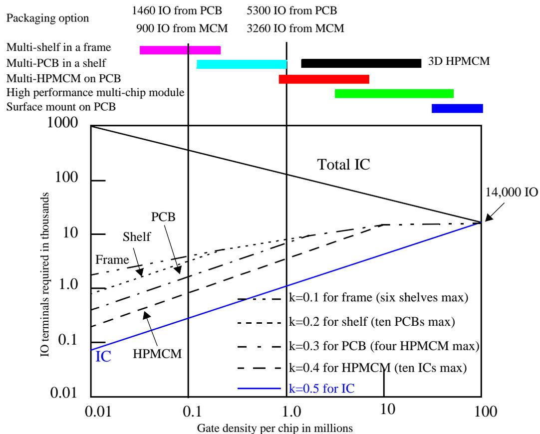
Figure 1.2: Rent's rule for large system IO.  $k$  represents sharing of interconnects [13].
