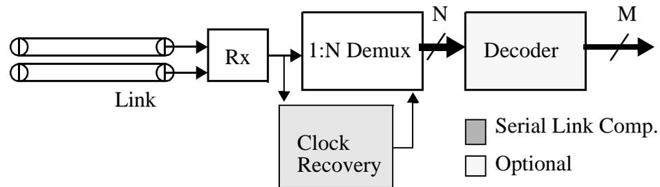
Figure 2.1: Block diagram of typical serial data link receiver.
