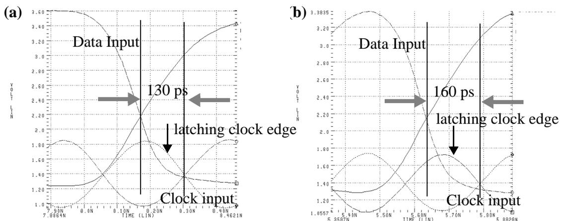
Figure 3.24: Setup time for D flip-flop in Figure 3.21 at 2 GHz. Hold time is -20 ps.
