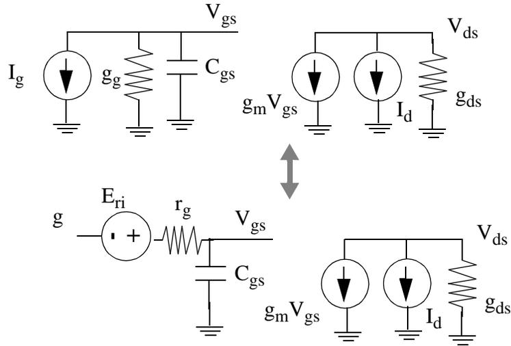
Figure 6.22: MOSFET noise model [183], showing noise sources considered in this work.
