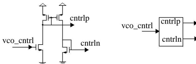
Figure 4.24: Schematic and symbol of noise-oscillator control circuit.
