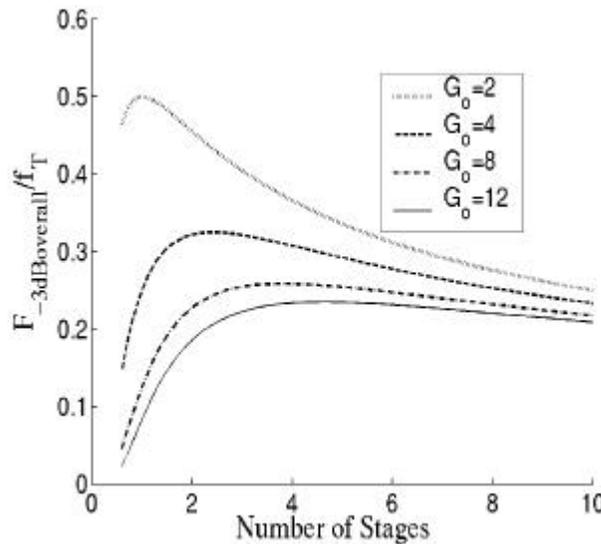
Figure 6.15: Variation of  $F_{-3dBoverall}/f_u$  with the number of amplifier stages,  $n$ , for overall gain  $G_0$  of 2, 4, 6 and 8.
