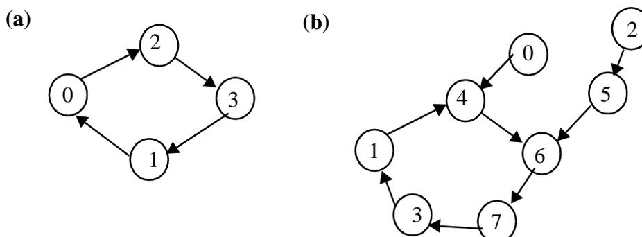
Figure 3.16: State diagram of the 4/5 prescaler in (a) divide-by-4 and (b) divide-by-5 operation.
