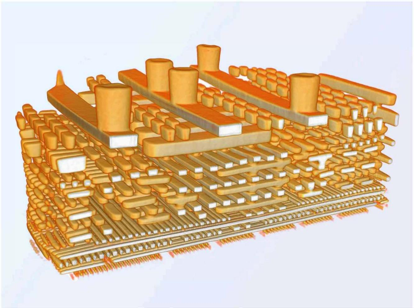
A 4-nanometer resolution X-ray technique can render a chip's inner workings from the large interconnects at the top to the transistors at the bottom.
