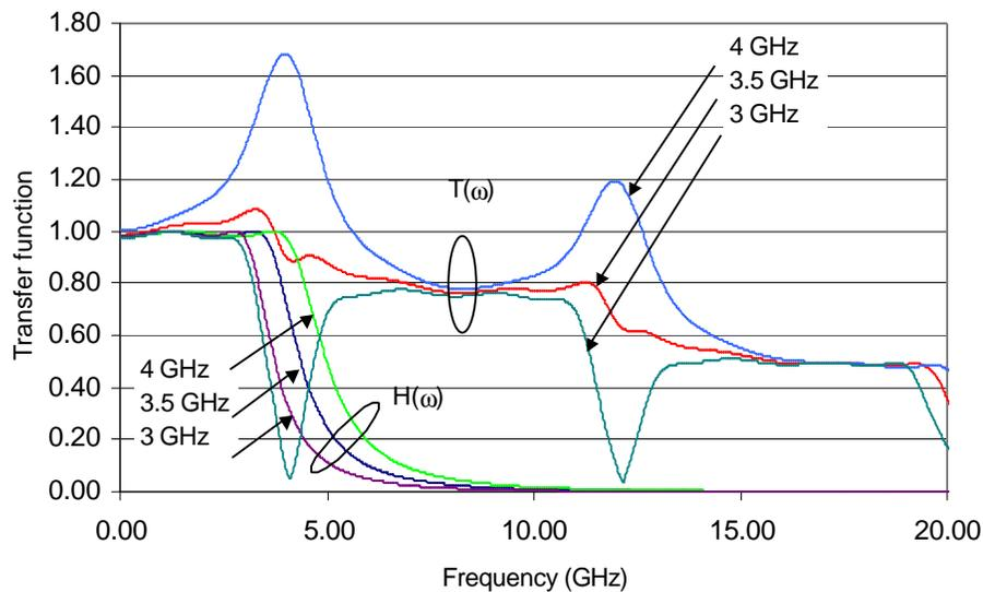
Fig. 3 - Transfer function  $H(\omega_{RF})$  of the LPF and corresponding 5-channel system transfer functions  $T(\omega_{RF})$  for different LPF  $-3$  dB bandwidths for four-pole Chebyshev filters.
