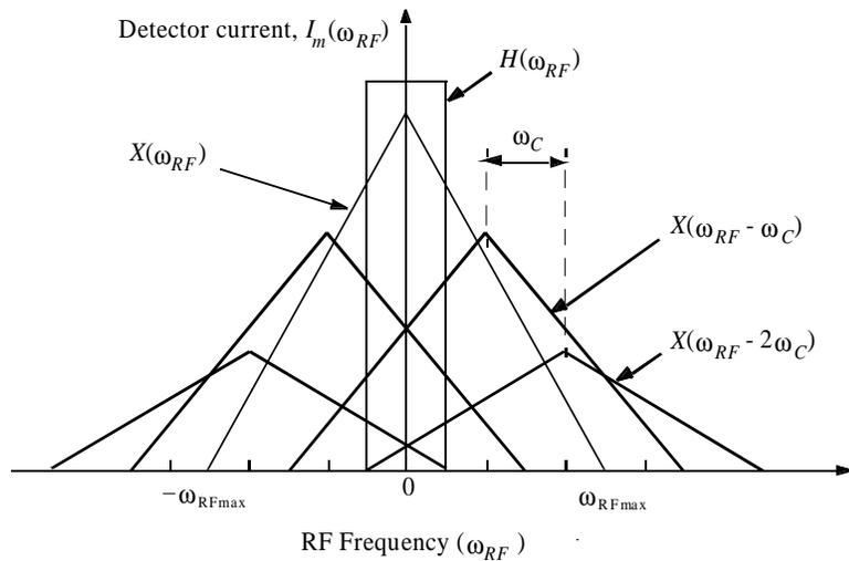
Fig. 2 - Schematic diagram of signal mixing in each detector. The high frequency components are mixed with low frequency components because of the mode spacing  $\omega_C$  is small compared to the RF bandwidth  $\omega_{RFmax}$ .
