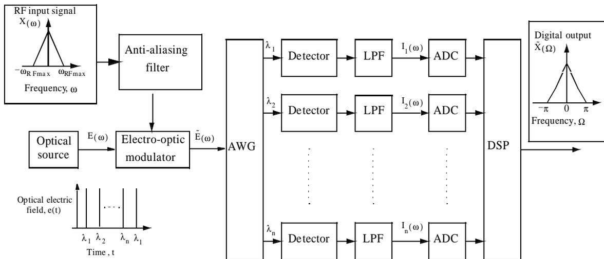
Fig. 1 - Schematic diagram of the hybrid opto-electronic WDM ADC system architecture. The optical multi-wavelength source is RF modulated and demultiplexed using an AWG. The output of the AWG is detected, low-pass filtered, and quantized. DSP reconstructs the original signal.
