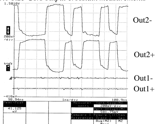
FIGURE TE01.3: Measured output at 1.25 Gb/s. Cross-talk is less than -24 dB
