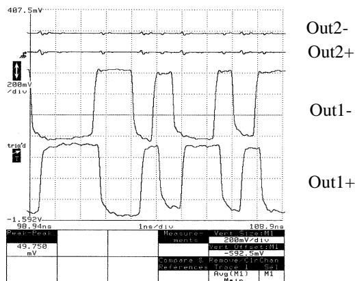
FIGURE TE01.4: Measured output at 1.25 Gb/s. Cross-talk is less than -23 dB
